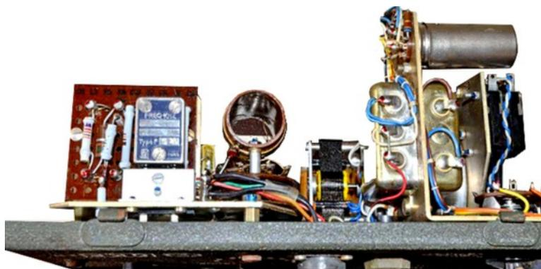
Internal view of TAL 6 seen from bottom showing crystal, RF output coil and parts of the auto keyer assembly.
