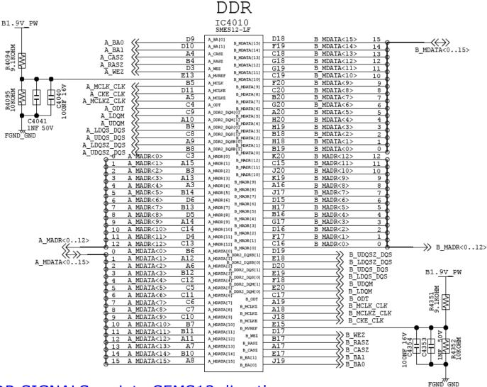
DDR SIGNALS go into SEMS12 directly
