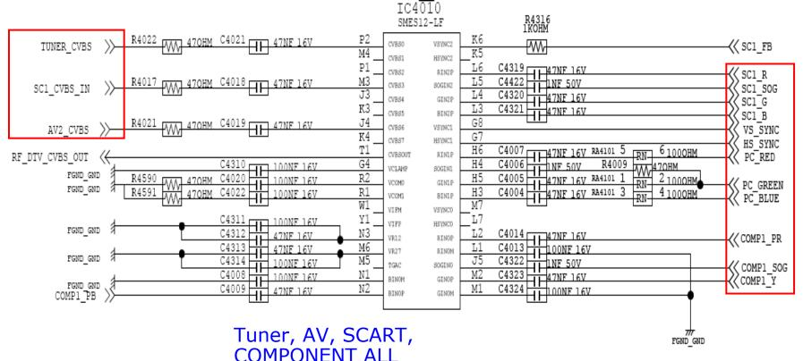
COMPONENT ALL VIDEO INPUT SIGNALS go into SEMS12 directly,
