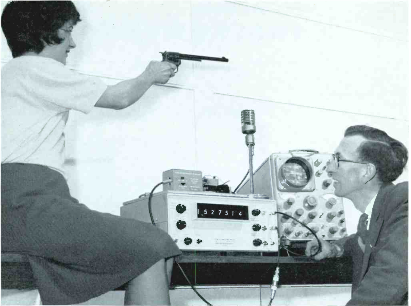
Work on a problem in the Marconi Instruments applications laboratory. Preparations are being made for a television programme in which a TF 1417 Counter is being used to find out how quick a cowboy is on the draw. A pulse from the microphone stops the counter when the gun is fired.
