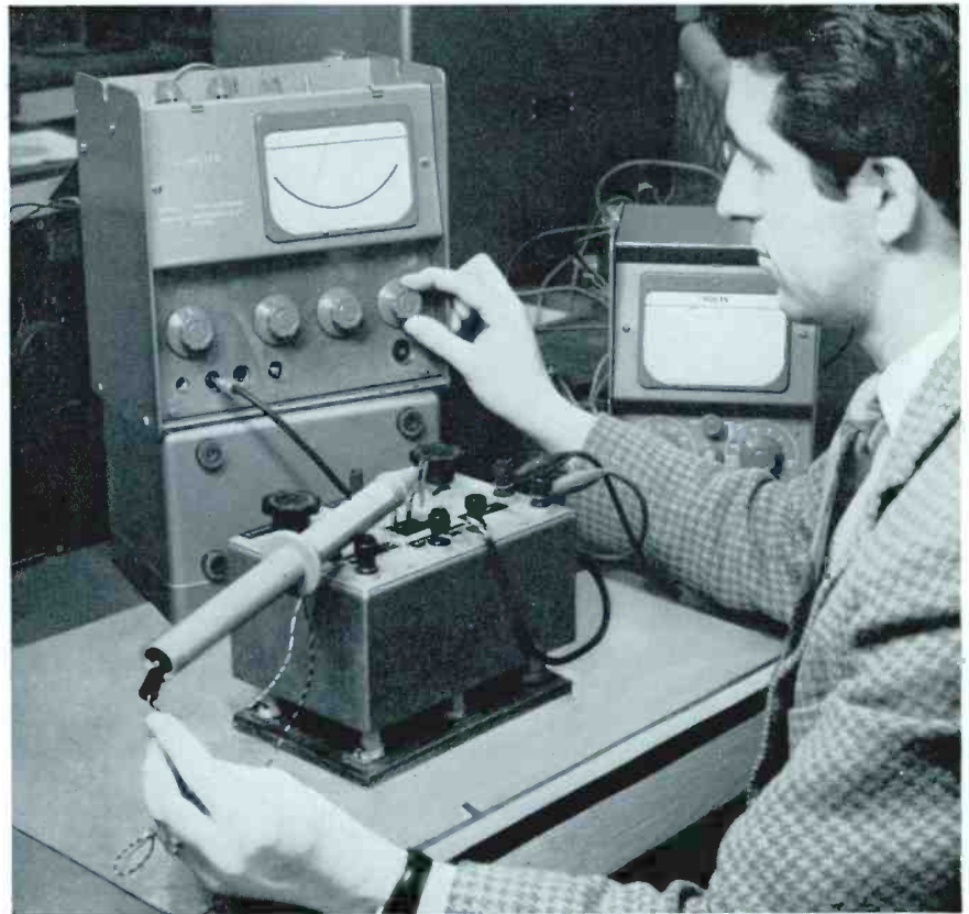
A calibration engineer uses the TF 1093 pH meter as a bridge detector in measuring the resistance of a d.c. multiplier for the TF 1041C valve voltmeter
