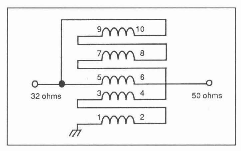
Figure 1. Schematic diagram of the quintufilar UNUN transformer designed to match 50 ohms to 32 ohms
