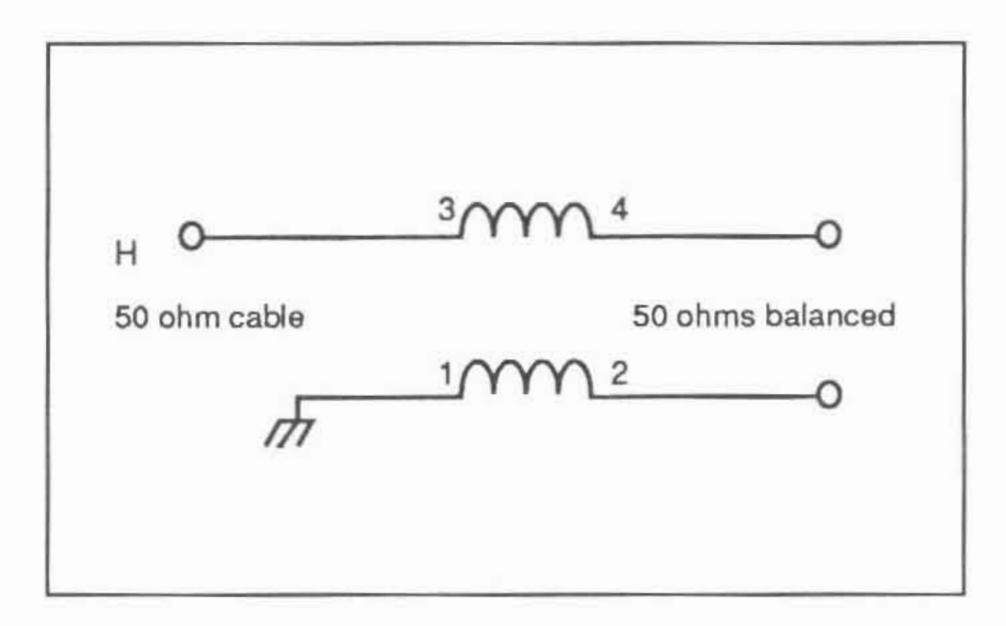
Figure 1. Schematic diagram of the Guanella 1:1 balun transformer
