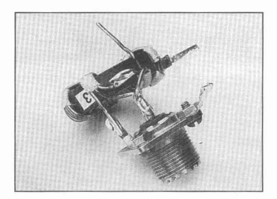
Figure 2 - Bottom-view of the highly efficient and broadband dual-output W2FMI-2:1-LDU50 transformer.
