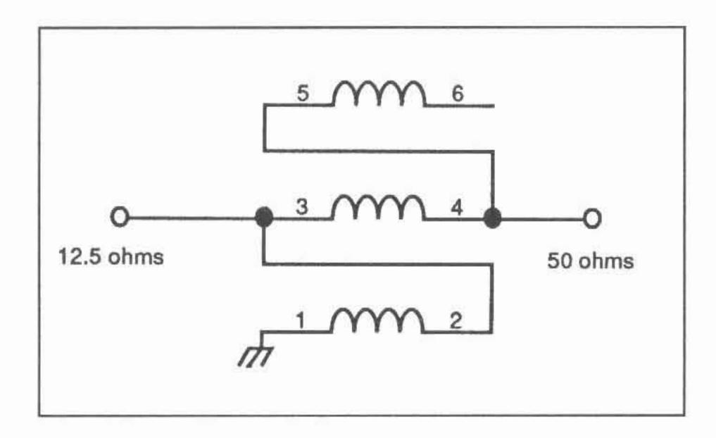
Figure 1. Schematic diagram of the "floating-third wire" UNUN transformer desinged to match 50 ohms to 12.5 ohms
