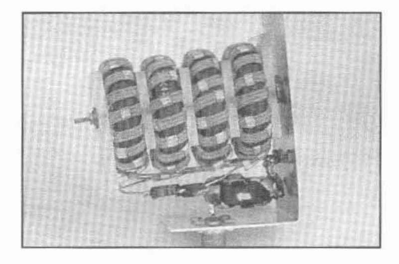
Figure 2 - A view of the high power and broadband W2FMI-12:1-HB600 transformer.
