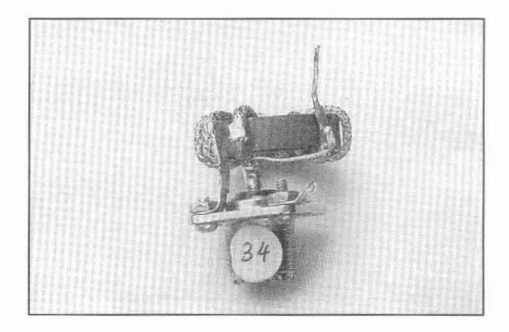
Figure 2 - Bottom-view of the highly efficient and broadband W2FMI-4:1-LCU50 transformer.
