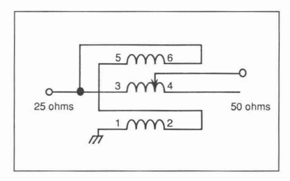
Figure 1. Schematic diagram of the trifilar UNUN transformer designed to match 50 ohms to 25 ohms
