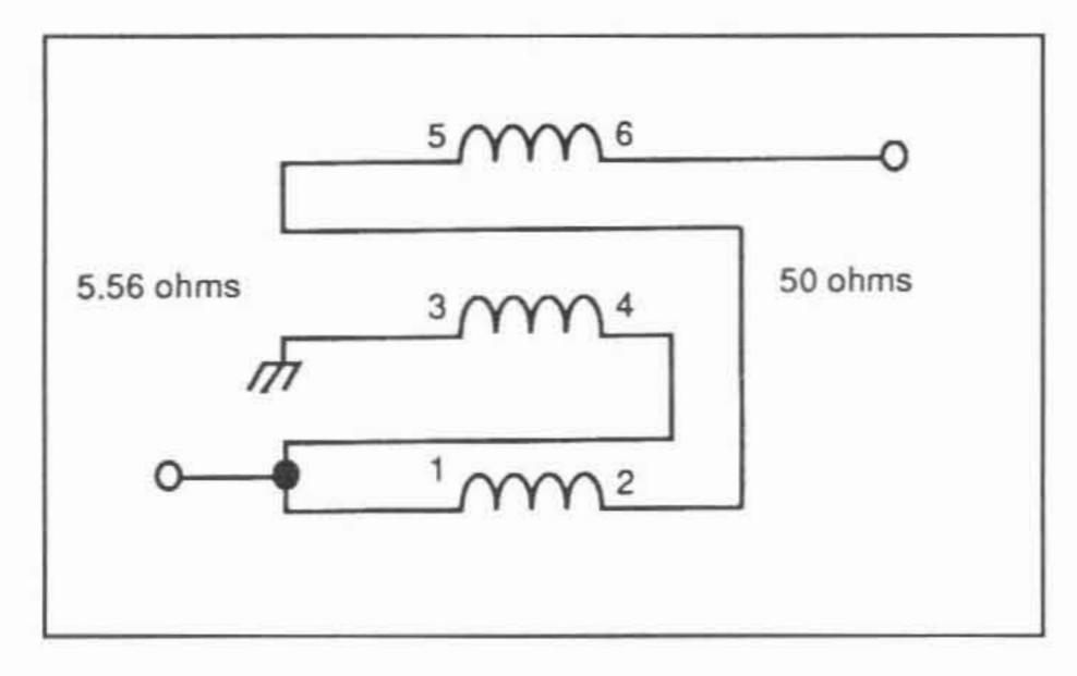
Figure 1. Schematic diagram of the trifilar UNUN transformer designed to match 50 ohms to 5.56 ohms
