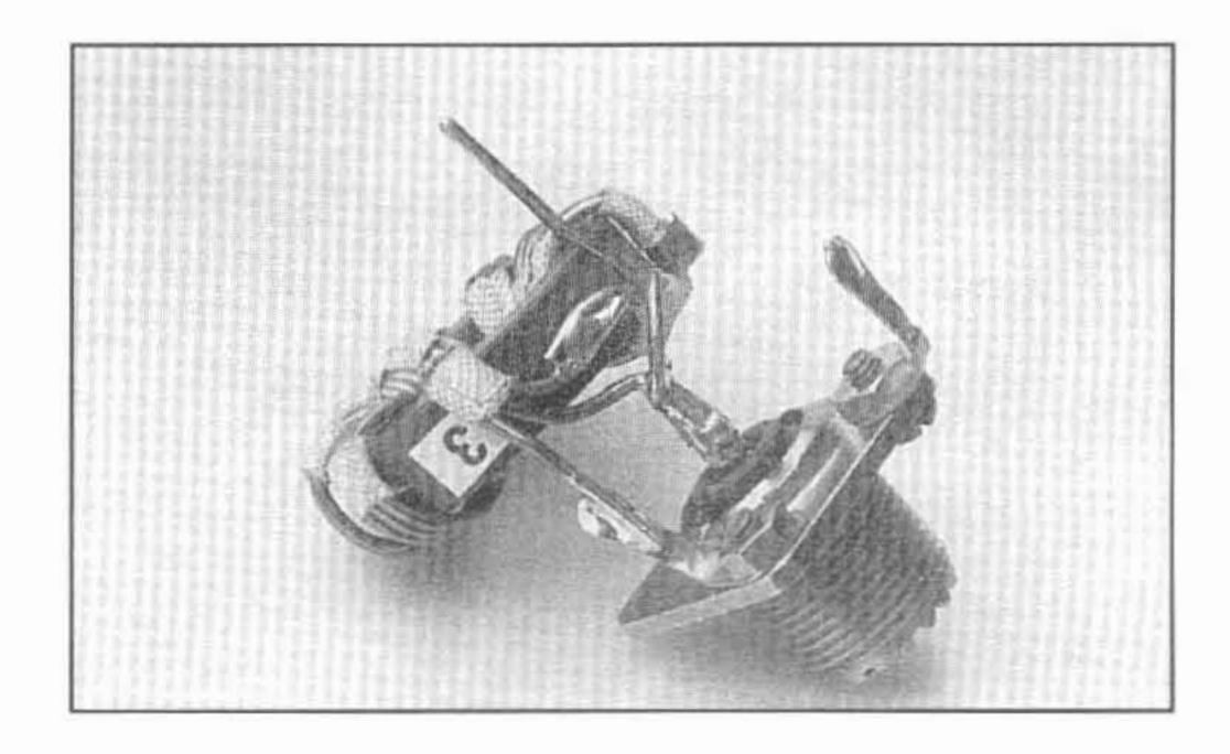
Figure 2 - Bottom-view of the highly efficient and broadband W2FMI-2.25:1-LU50 transformer.
