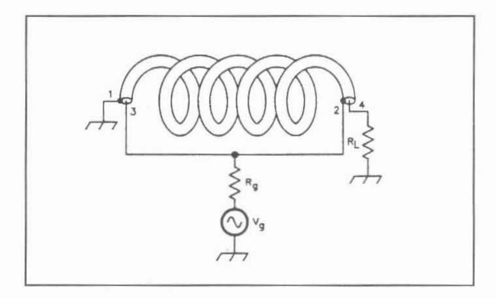
Figure 1. Schematic diagram of the coaxial cable version of the Ruthrof 4:1 UNUN transformer designed to match 50 ohms to 12.5 ohms
