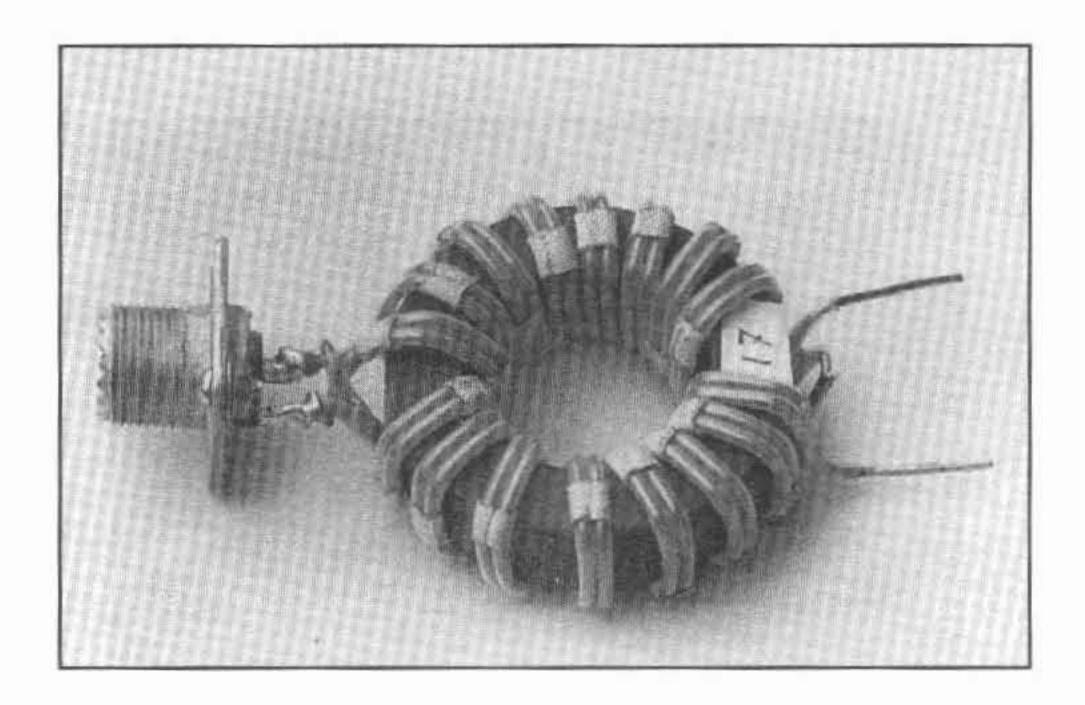
Figure 2 - Bottom-view of the high power and broadband W2FMI-4:1-HBM200 transformer.
