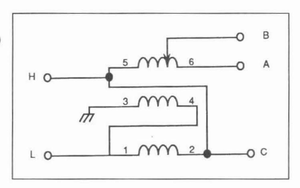
Figure 1. Schematic diagram of the multi-match UNUN transformer designed to match 50 ohms to five lower impedences
