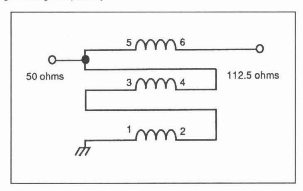
Figure 1. Schematic diagram of the trifilar UNUN transformer designed to match 112.5 ohms to 50 ohms
