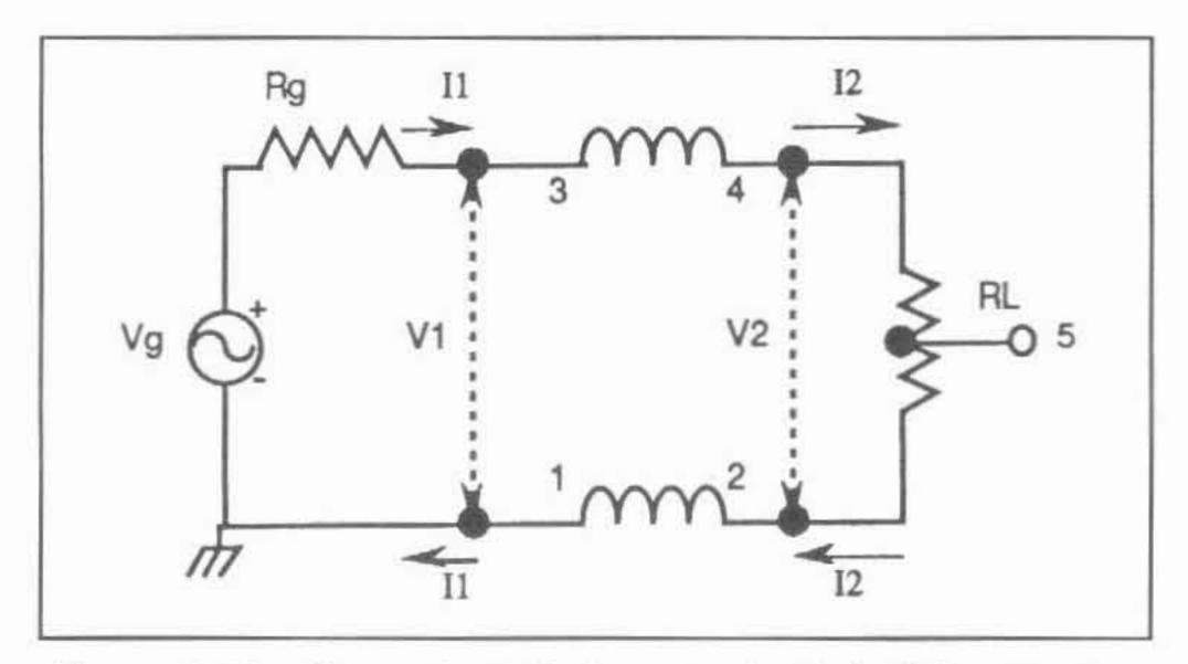
Figure 1. The Guanella 1:1balun: the basic building block
