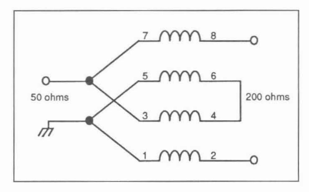
Figure 1. Schematic diagram of theGuanella balun transformer designed to match 50 ohms to 200 ohms
