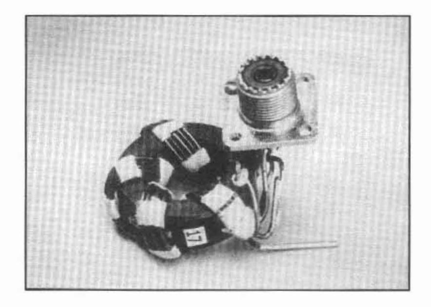
Figure 2 - Bottom-view of the highly efficient and broadband W2FMI-1.56:1-HDU50 transformer.
