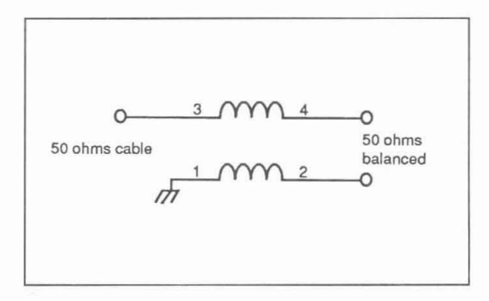
Figure 1. Schematic diagram of the Guanella 1:1 balun transformer
