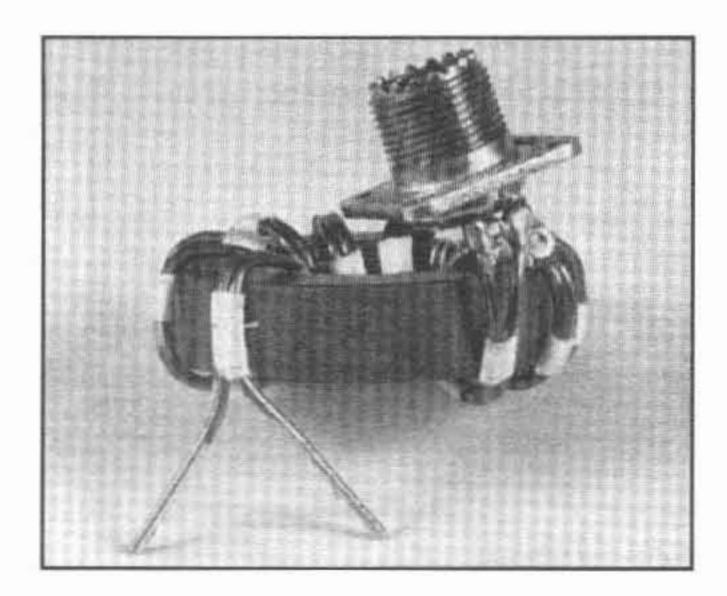
Figure 2 - Bottom-view of the highly efficient and broadband W2FMI-1:1-HBL50 transformer.
