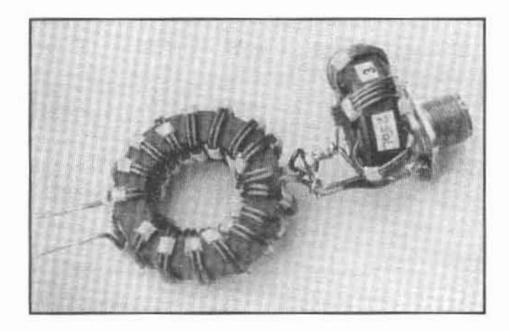
Figure 2 - A view of the compound-balun W2FMI-2.25:1-HB112.5 transformer.
