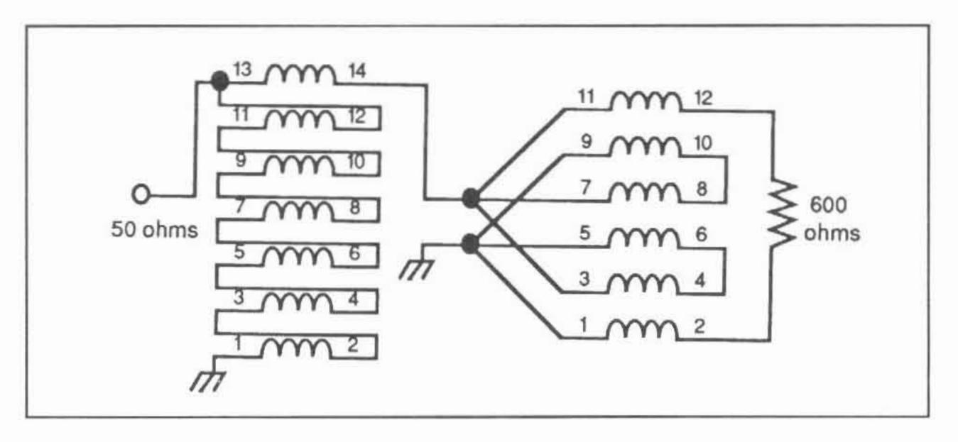
Figure 1. Schematic diagram of the compound balun with a 12:1 ratio designed to match 50 ohms to 600 ohms
