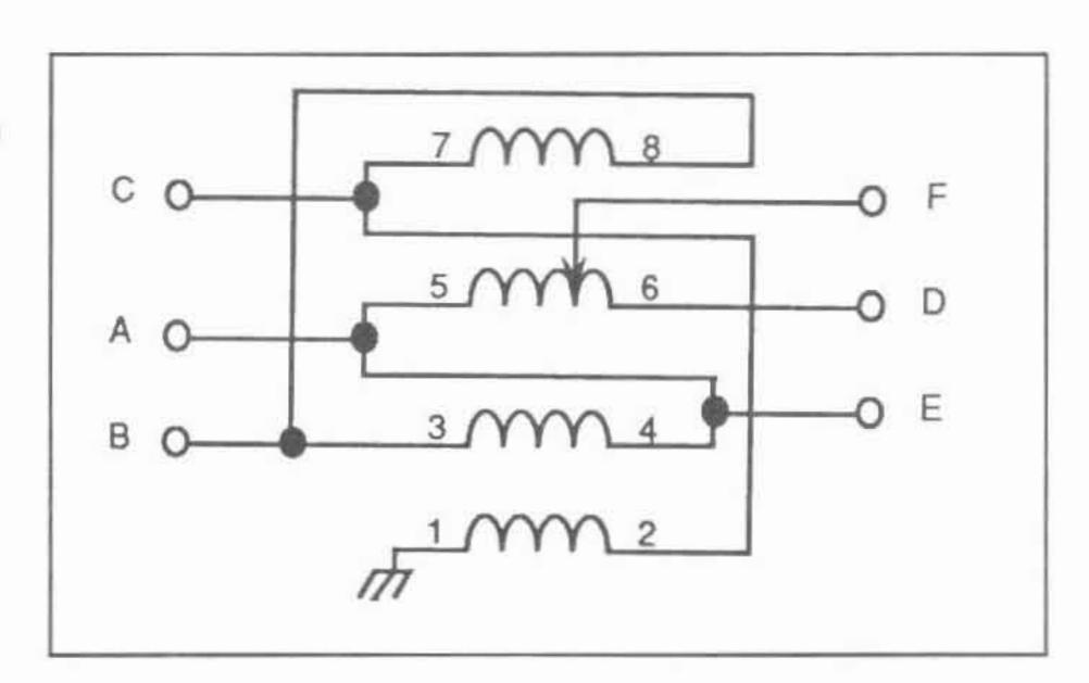
Figure 1. Schematic diagram of the multi-match UNUN transformer designed to match 50 ohms to five lowe impedences
