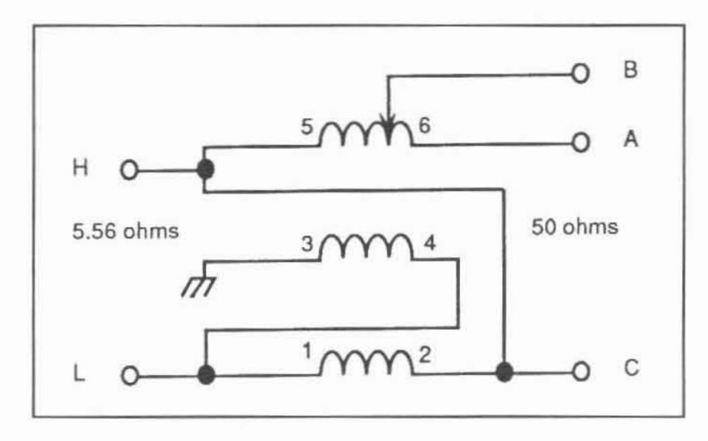
Figure 1. Schematic diagram of the trifilar multi-match transformer designed to match 50 ohms to 6 lower impedances
