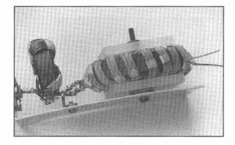
Figure 2 - Bottom-view of the high power and broadband W2FMI-6:1-HB300 transformer.
