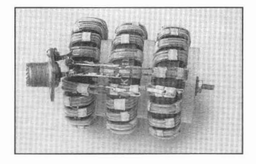
Figure 2 - Bottom-view of the high power and broadband W2FMI-9:1-HB450 transformer.
