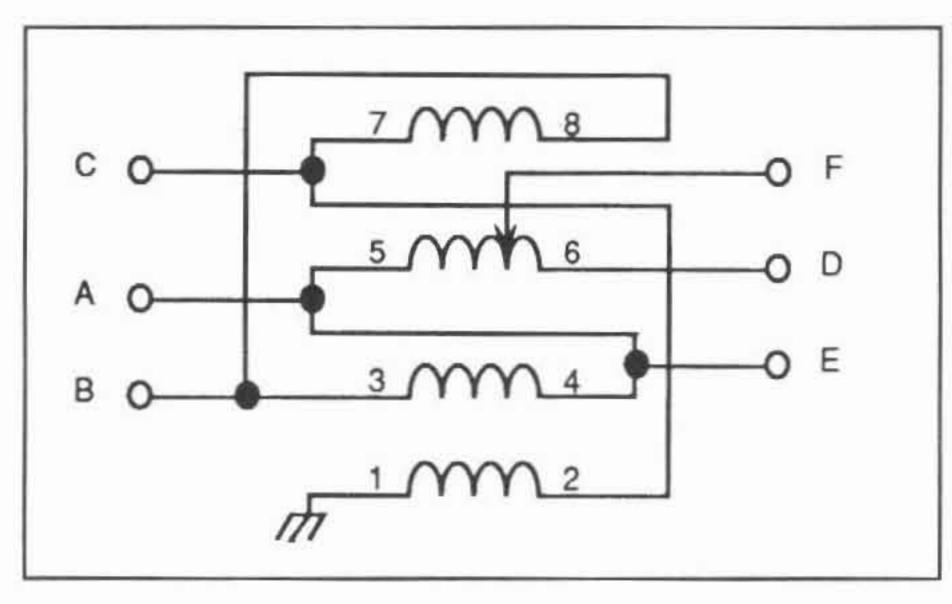
Figure 1. Schematic diagram of the dual-output transformer designed to match 50 ohms to 32 ohms or 18 ohms
