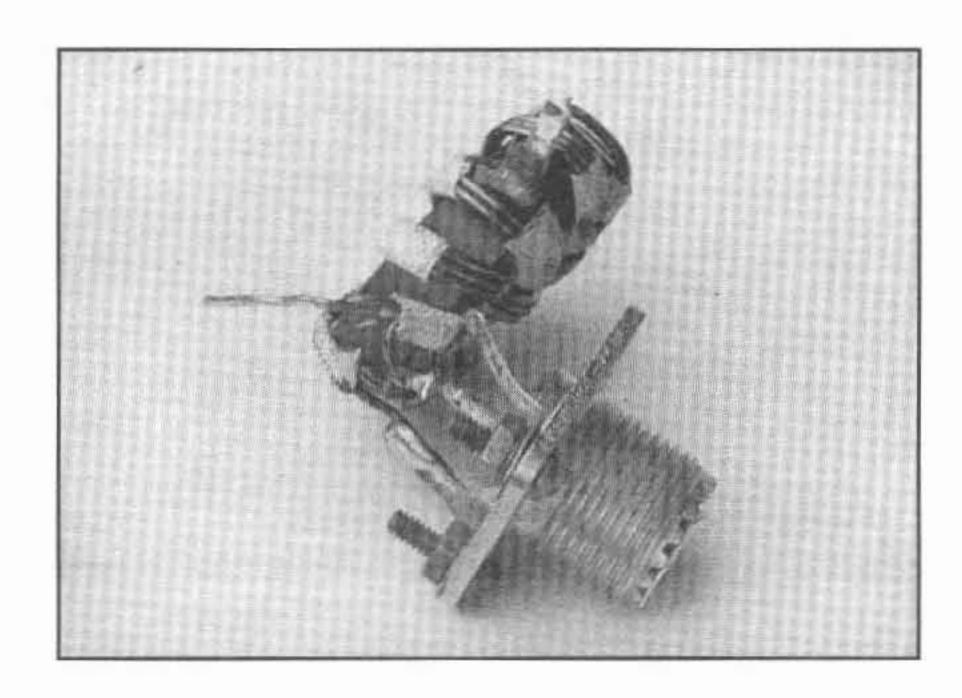
Figure 2 - Bottom-view of the highly efficient and broadband W2FMI-2:1-LDU100 transformer.
