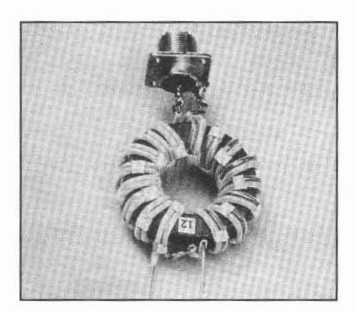
Figure 2 - Bottom-view of the highly efficient and broadband W2FMI-4:1-HBL200 transformer.
