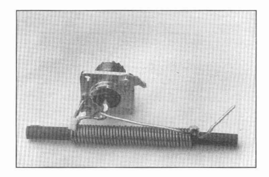
Figure 2 - Bottom-view of the highly efficient and broadband W2FMI-4:1-LRU100 transformer.
