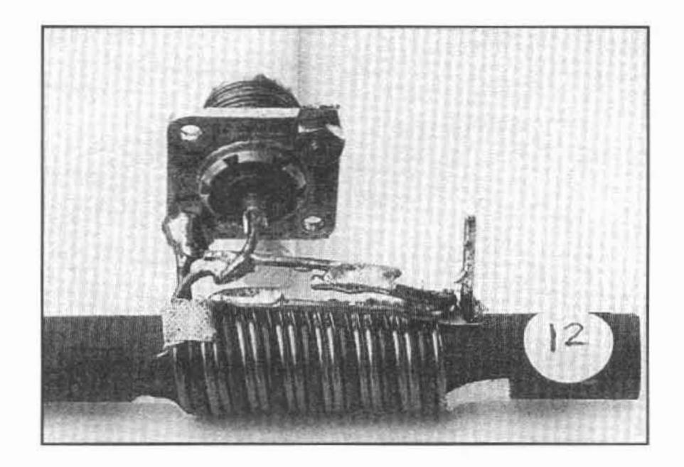
Figure 2 - Bottom-view of the highly efficient and broadband W2FMI-9:1-HRU50 transformer.
