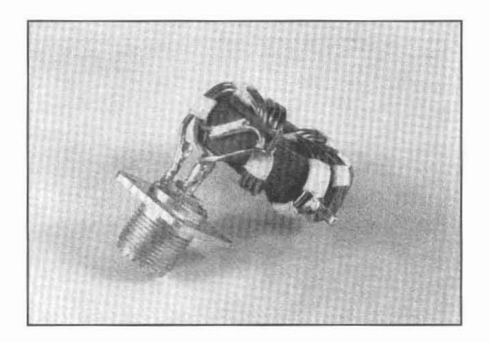
Figure 2 - Bottom-view of the highly efficient and broadband W2FMI-2:1-HU50 transformer.
