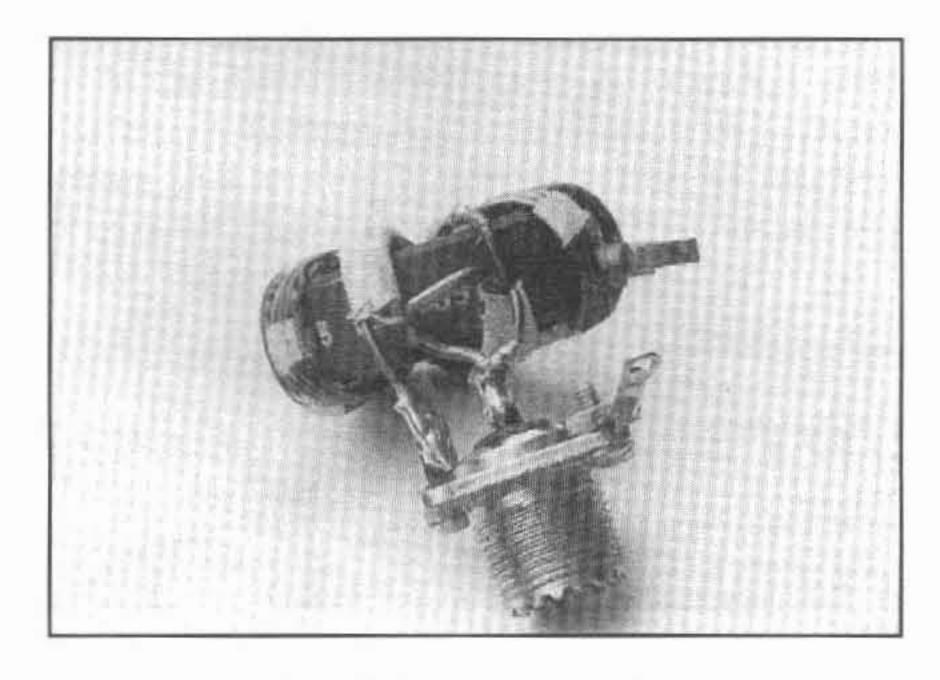
Figure 2 - Bottom-view of the highly efficient and broadband W2FMI-2:1-HU100 transformer.
