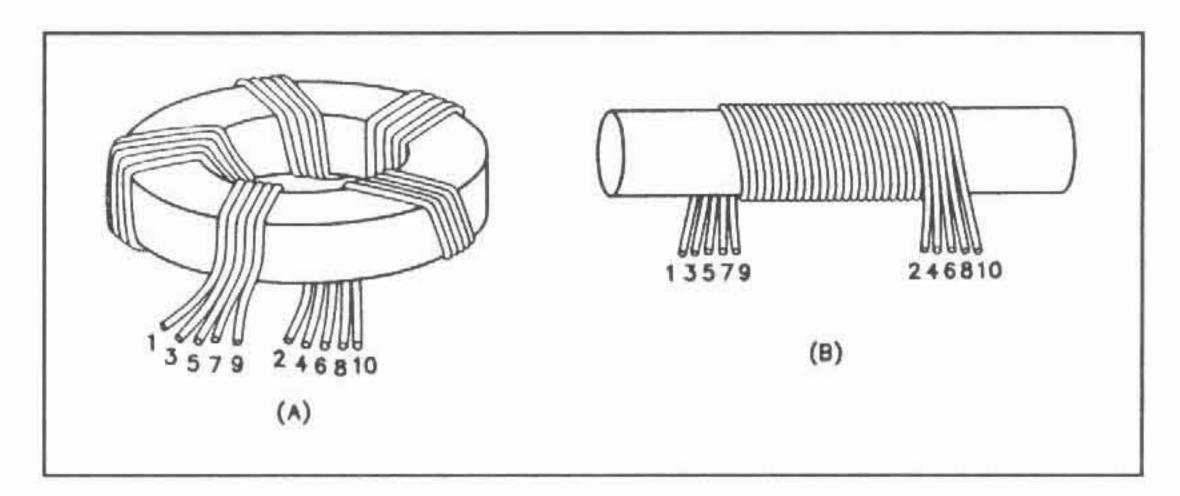
Figure 2 - Pictorials of quintufilar windings: (A) toroid and (B) rod.
