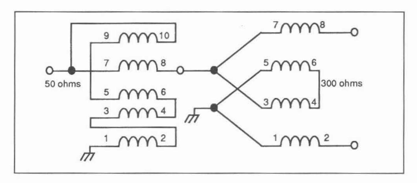
Figure 1. Schematic diagram of the compound balun with a 1:6 ratio designed to match 50 ohms to 300 ohms
