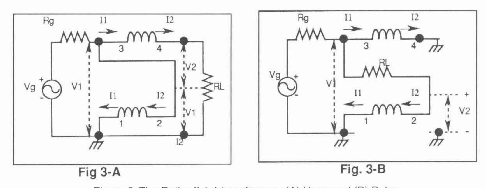
Figure 3. The Ruthroff 1:4 transformer: (A) Unun and (B) Balun
