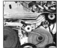
Tachometer wheel continuously controls the speed of tape.
