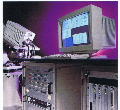
Computerized dynamic validation bench used to qualify the operational flight program.
