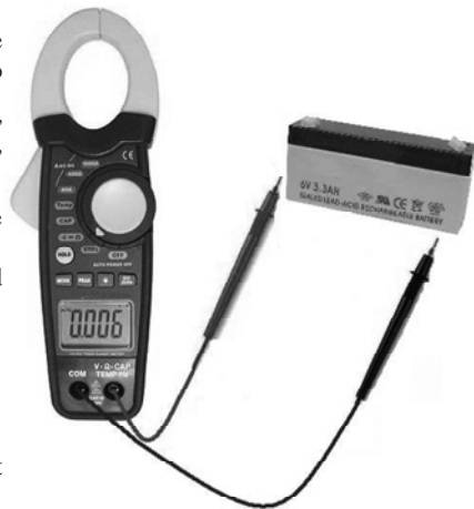
Example of DC voltage measurement
