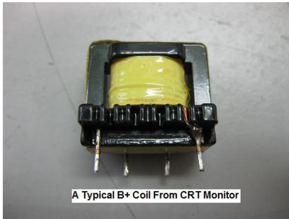
Figure 14.9- A Typical B+ Coil From CRT Monitor
