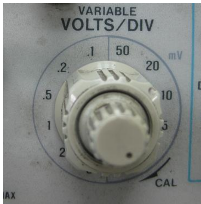
Figure 12.8- Set The Right Voltage
