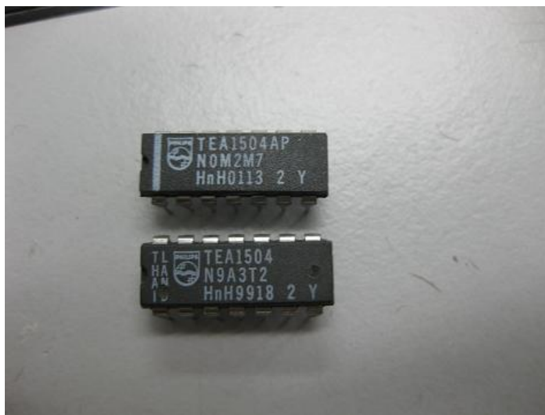
Figure 6.4- Insist on Getting The Same Part Number Especially The Power IC
