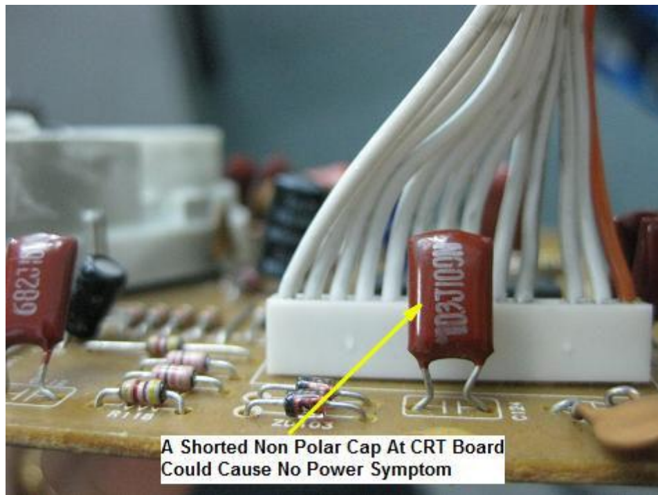
Figure 18.1- Shorted Non Polar Capacitor At CRT Board
