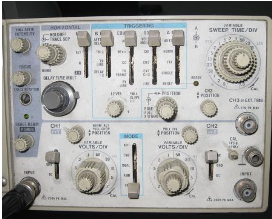
Figure 12.5- A Typical Analog Scope
