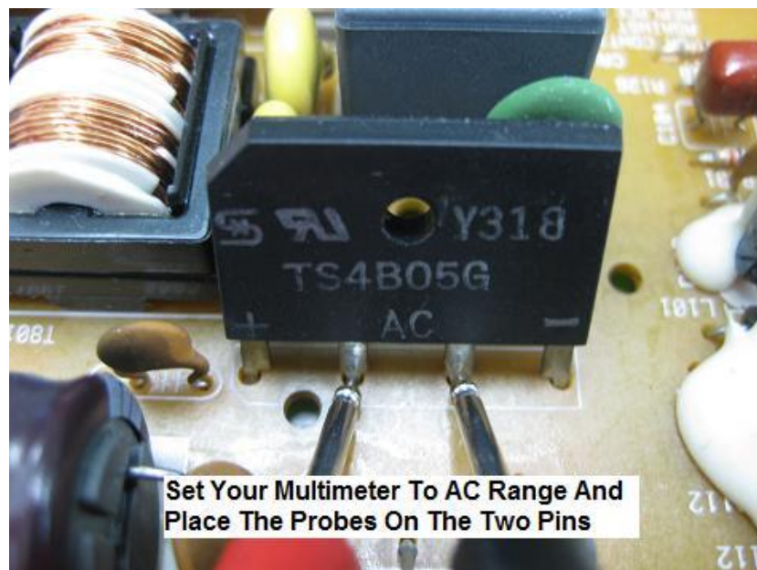
Figure 11.2- Place Your Test Probes To The Right Points
