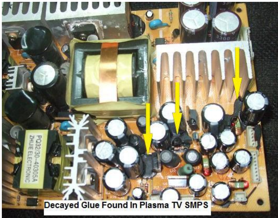
Figure 15.12- Decayed Glue Found In Circuit Board
