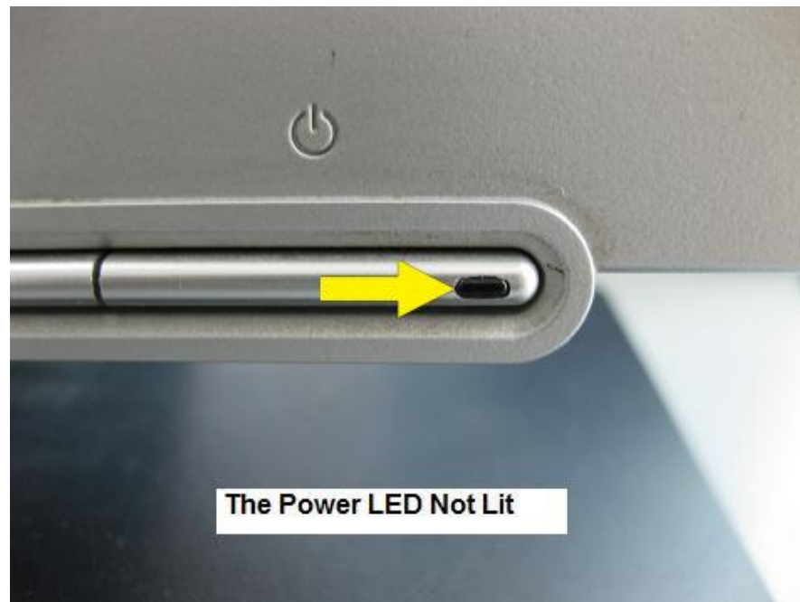
Figure 9.1- The LED Act As A Power Indicator
