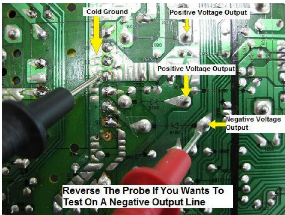
Figure 14.8- Reverse The Probe If You Want To Test On A Negative Output Line
