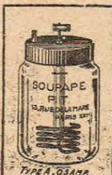
**UN MOYEN PRATIQUE DE RECHARGER LES ACCUS DE 40 ET 80 VOLTS SUR UNE TENSION DE 4 VOLTS**
