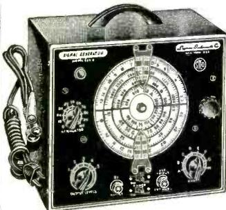
• Tubes used: 1-6BE6 as R. F. Oscillator, mixer and amplifier. 1-6BE6 as Audio Oscillator. 1-6MG as Power Rectifier.
