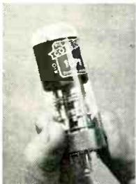
The *Cossor* 1CP1 has a standard Loktal base, electrostatic deflection, and fixed electrostatic focus, all of which simplify its application to compact test and monitoring equipment. The 1CP1 operates
