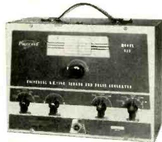
MODEL 635 UNIVERSAL AF SINE, SQUARE AND PULSE GENERATOR. For accurate testing audio and video circuits. 1% Ceramic precision resistors; Wien Bridge; variable Z and cathode-follower output; minimum overshoot and roundoff through 100,000 cycles; sine waves through 200 KC
