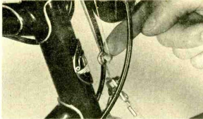
The front brake light switch is attached to the brake cable with strong nylon cord. The cord is in turn fastened to a specially drilled bolt which, when tightened onto the brake cable, tensions it to the switch.
