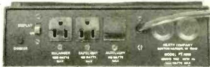
The back panel of the PT-1500 shows the 2 supplied jacks, as well as the cutout for the optional third jack for accessory use.
