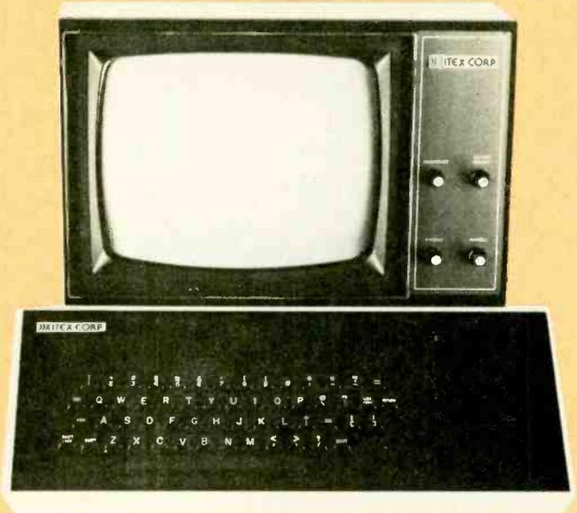
The XITEX MRS-100 is a complete unit which will allow owners of the TRS-80 computer to interface with their rigs to send and receive CW at speeds of up to 150 WPM. Circle no. 72.
