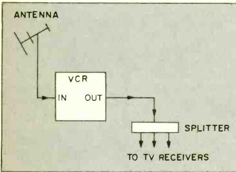
Shown here in its simplest form, this VCR system carries signal from the antenna, to the VCR itself, and then to the various TVs.
