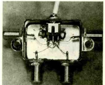
Line splitters are easily modified to take a switch. This switching ability is vital.
