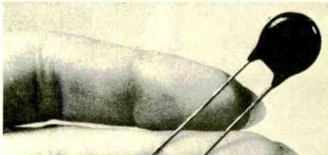
Metal oxide varistors are installed across AC power lines, protecting against line transient surges caused by lightning hitting a nearby power line.
