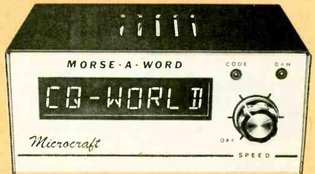
The "Morse-A-Word" by Microcraft is a CW only reader with eight digit LED display. Like all CW readers, it works best with a good fist on the other end. Circle no. 71 on the R.S. Coupon.
