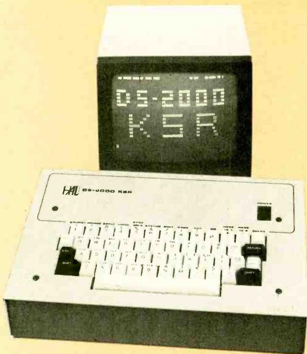
The HAL DS-200KSR offers RTTY with five speeds. It is modular, and can be expanded to include CW. A video monitor can also be added later. Circle number 76 on the R.S. Coupon.
