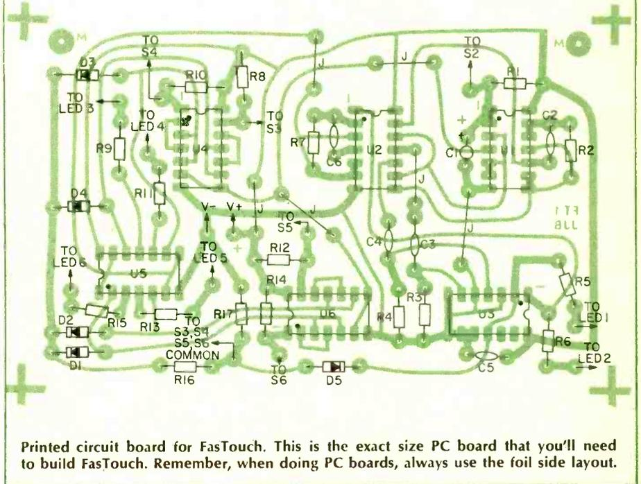
Printed circuit board for FasTouch. This is the exact size PC board that you'll need to build FasTouch. Remember, when doing PC boards, always use the foil side layout.
