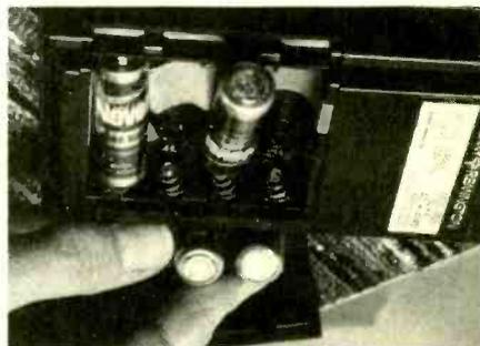
**Corroded Battery Terminals.** When batteries are left unused for a long period of time, they begin to leak and corrode around the battery terminals. Try to keep fresh batteries in the calculator to prevent corroded terminals. Replacement with leak-proof and long life batteries helps, but after a long it takes only a very small amount of corrosion to prevent juice from getting to the calculator's circuitry. A light going over with alcohol very often does the trick.
