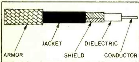
This cutaway diagram shows the several concentric (or coaxial) layers which make up coaxial cables. Armor is an optional item.
