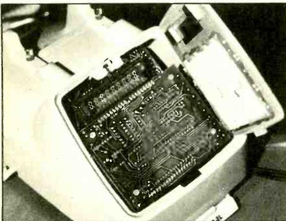
Intelli-Phone with its front dial plate off. You're looking at the nine-digit fluorescent display, and the foil side of the PC board. Circle R. S. number 80.
