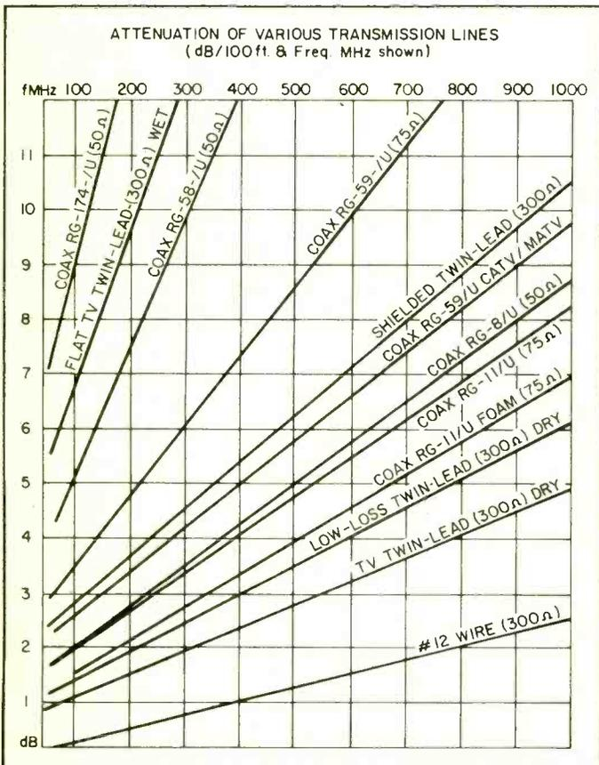
The table shows the attenuation characteristics of various transmission lines; calculations are for 100 foot lengths under wet and dry conditions. Measurements show dB attenuation as it corresponds to frequency in MHz. It shows the variance.
