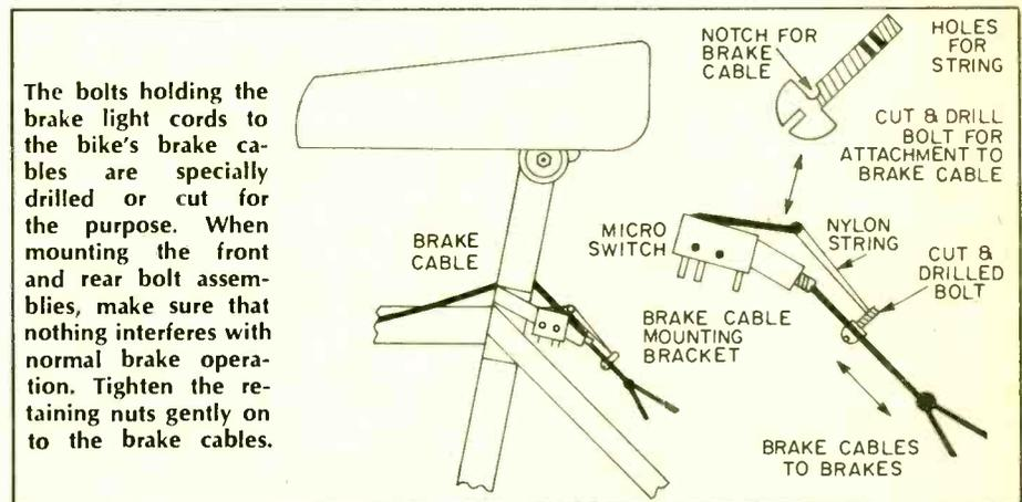
The bolts holding the brake light cords to the bike's brake cables are specially drilled or cut for the purpose. When mounting the front and rear bolt assemblies, make sure that nothing interferes with normal brake operation. Tighten the retaining nuts gently on to the brake cables.
