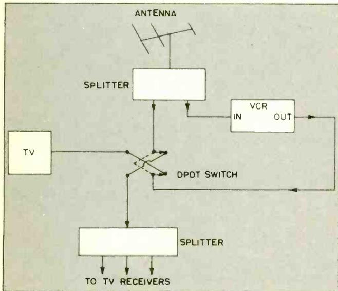
This is a diagram of a fancy home VCR system. It feeds up to four separate sets, and can be switched to provide live TV, or "canned" video programming. Without getting into elaborate and expensive equipment like metal towers or cable TV grade hook-ups this system will give a great deal of satisfaction for a reasonable pricetag.
