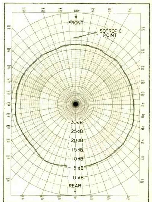
Fig. 4. An array with 0-degree phasing and  $\frac{1}{4}$ -wavelength element spacing (9-feet) puts out a nice omnidirectional pattern, but how many people do you know that have 9-foot wide automobiles?
