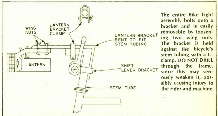
The entire Bike Light assembly bolts onto a bracket and is easily removable by loosening two wing nuts. The bracket is held against the bicycle's stem tubing with a U-clip. **DO NOT DRILL** through the frame, since this may seriously weaken it, possibly causing injury to the rider and machine.
