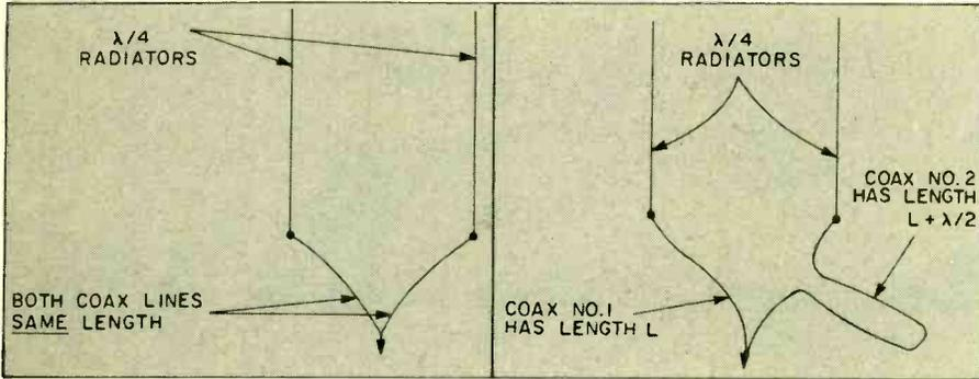
Fig. 2. Configuration depicts a co-phased array using equal length feed lines to obtain a 0-degree phase relationship.
