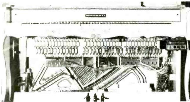
encode, then reenact a performance as it was originally played. The cassettes are inserted in a small tape recorder which activates the piano keys via a logic circuit board mounted across the open space behind the keys. Installation takes from 8 to 12 hours. Pianocorder kits, including all componentry, step-by-step instructions and a bonus set of ten tapes, start at \$1495. For more information or direct ordering, write Superscope, Inc., 20525 Nordhoff St., Chatsworth, CA 91311.
