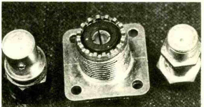
The most commonly used coaxial connectors are, from left to right, the BNC, SO-239 and F-type. These cover nearly every coax use.
