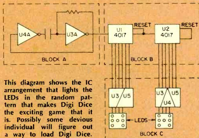
This diagram shows the IC arrangement that lights the LEDs in the random pattern that makes *Digi Dice* the exciting game that it is. Possibly some devious individual will figure out a way to load *Digi Dice*.
