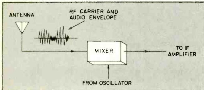
In CB sets the frequency to which the oscillator is tuned is often two to 11 MHz above (or below) the incoming RF carrier frequency, instead of 455 kHz.
