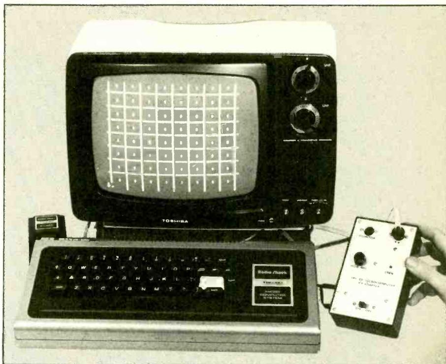
tips at ground and video white level at about 1.4-volts. The TV adapter also allows tandem display of the TRS-80 and a TV for group viewing.
