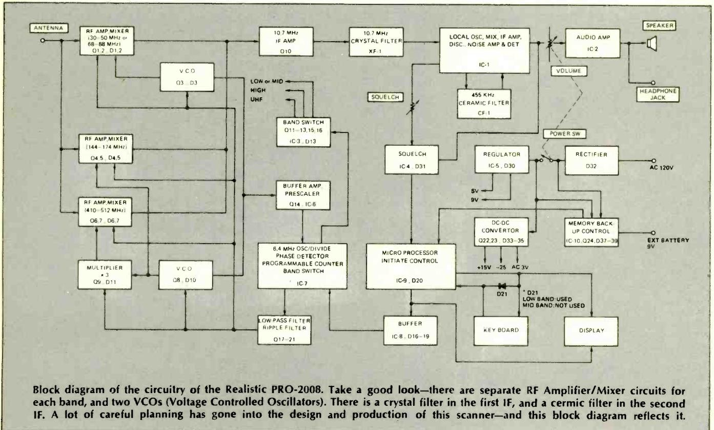
Block diagram of the circuitry of the Realistic PRO-2008. Take a good look—there are separate RF Amplifier/Mixer circuits for each band, and two VCOs (Voltage Controlled Oscillators). There is a crystal filter in the first IF, and a ceramic filter in the second IF. A lot of careful planning has gone into the design and production of this scanner—and this block diagram reflects it.
