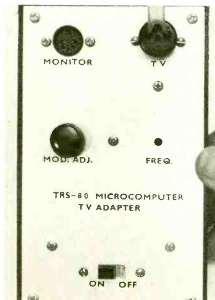
The completed project, showing modulation and frequency adjustment controls in front.
