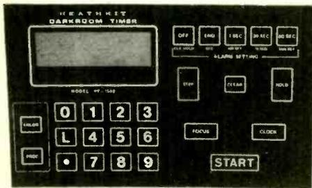
The front panel, which is made up of the switch matrix, has a very tough adhesive on it. If you apply the panel unevenly to the chassis, that's the way it will stay, so be very very careful!
