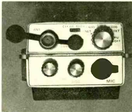
The top panel outlets for: (clockwise) antenna, earphone, scan select, offset split, microphone, squelch/tone, on-off volume.
