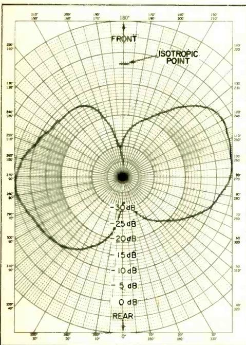
Fig. 3. A co-phased array utilizing  $\frac{1}{2}$ -wave radiators spaced  $\frac{1}{8}$ -wavelength apart will give a radiation pattern similar to this. This is not a particularly effective pattern for mobile use, as the maximum amount of energy is radiated off the sides of the array instead of front and back as is needed for road usage.
