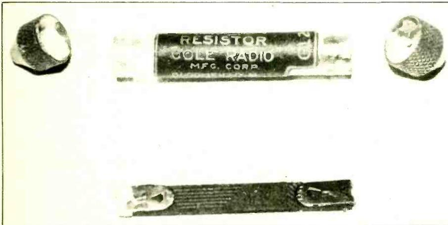
These parts make up one type of old grid leak. The grid leaks in use during the early days of radio tended to vary from 100,000 ohms to 10 megohms. While purists will insist on accurate restorations or replicas, a 500,000 ohm, 1/2-watt resistor is as good.
