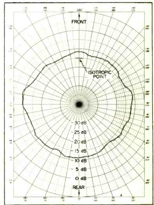
Fig. 6. The radiation pattern of a single element 2-meter whip mounted on the roof should be circular, but the irregular geometry of the car's shape precludes this.
