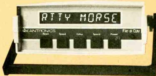
The "Field Day" by Kantronics is a highly compact Morse Code and RTTY reader, with a bright LED display. It can read Morse at up to eighty words per minute. Circle 74 on R.S. Coupon.
