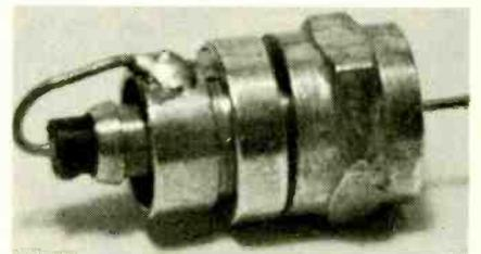
If you get "ghosts" from unused splitter outputs, make up terminations from F-type connectors and 1/2-watt carbon resistors.
