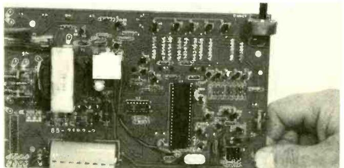
This is the completed circuit board, with the lone LSI chip seen at right center, and the power supply transformer at the left. It connects with the switch panel via a ribbon connector.
