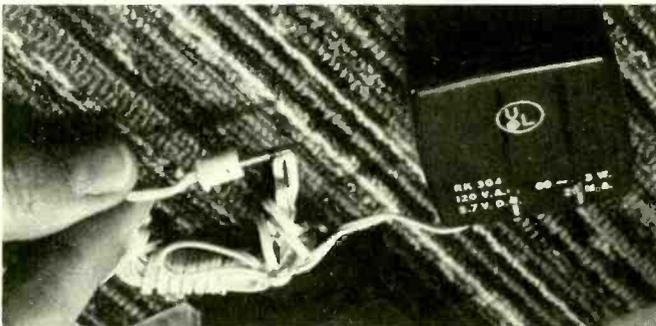
**Bad AC Adapter Jack.** When the calculator will function on batteries and not with the AC power supply, suspect a defective power supply or adapter
