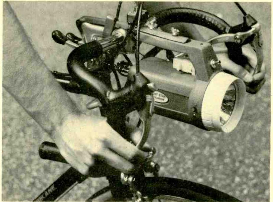
the plastic lantern housing to provide weatherproofing and resistance to vibration and road shocks.
