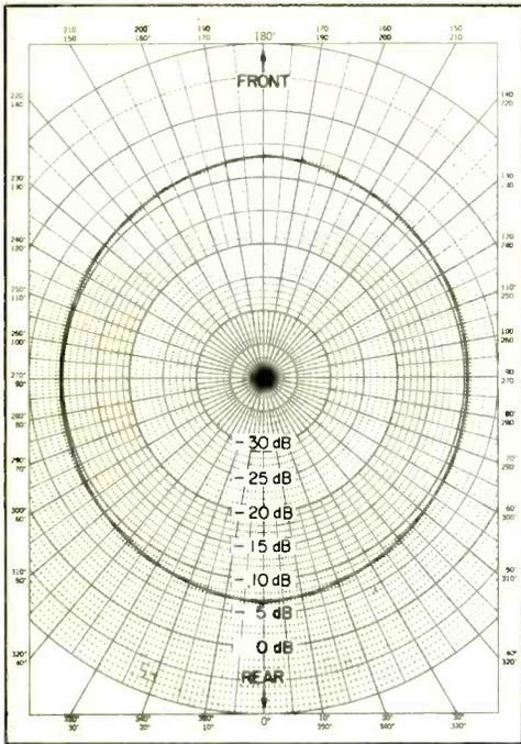
Fig. 5. The ideal radiation pattern for  $1/8$ -wavelength spacing of elements results in a fat ellipsoid. It's strongest front to back.
