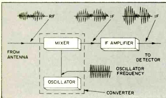
**The IF Amplifier**—The abbreviation for **intermediate frequency** is **IF**. In most home receivers the IF is 455 kHz. Amplifying a single frequency in the IF circuit is much easier and causes less distortion than if it were necessary to tune this amplifier to each of the many station frequencies. The only purpose of this stage is to amplify the IF (which still retains the original audio frequency) and pass it on to the detector.
