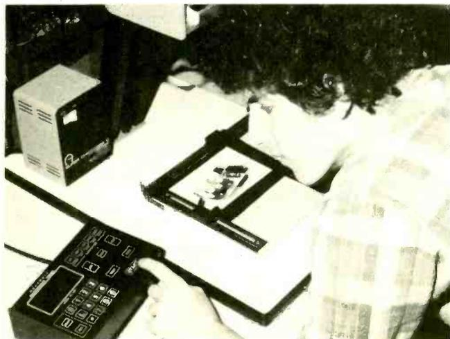
Here the PT-1500 is being programmed to time an enlarger exposure. There is an AC outlet on the back for switching the enlarger on and off.
