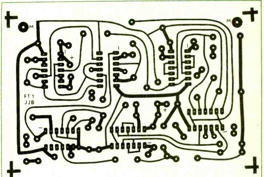
This is the parts location sketch for FasTouch. While FasTouch is not exactly an easy kit to build, there really aren't any stumbling blocks on the component layout side.
