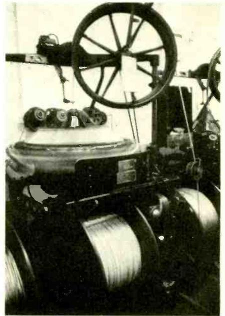
A patent weaving machine is used to spin the shielding braid around the foam dielectric in this photo from Alpha Wire Corp.
