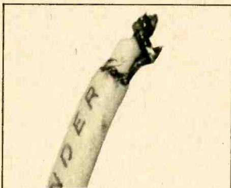
Here's a closeup of the probe assembly. Anode is soldered to the coax center wire.
