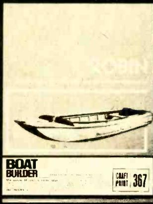
367. ROBIN is a versatile skiff that can be used for hunting or fishing, as a yacht club tender, or a work boat. It is rugged, yet its plywood construction makes it easy to build; no special jig or tools are needed. It can take a motor of 7-10 hp. L.O.A., 12'; beam, 5'1". \$5.00
