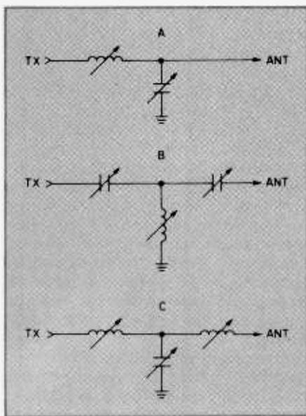
Fig. 1. These are the three basic circuit configurations for antenna tuners. Type A is an L network, B and C are T networks.
