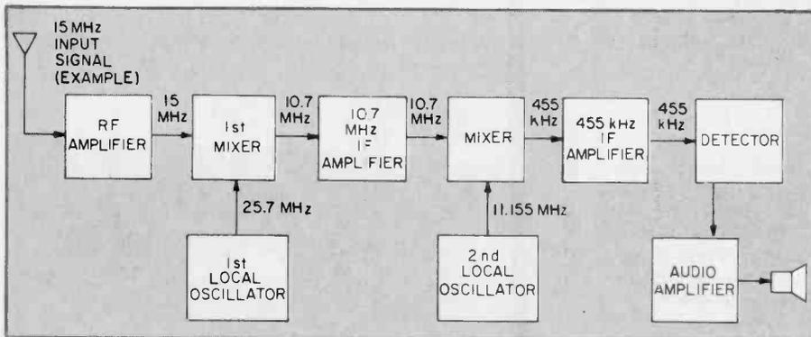
The dual conversion receiver features greater selectivity by narrowing the frequency width of the incoming signal in the second mixing stage, keeping out unwanted signals.
