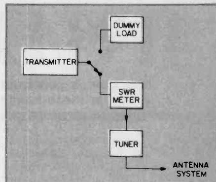
Fig. 6. This shows the basic configuration of the antenna line circuit with antenna tuner and SWR bridge in position on one side, and the dummy load (for tune-up purposes) on the other side of the coaxial antenna switch. See the text for all details.
