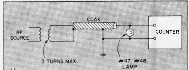
Three turns of number 18 gauge wire is fed by a suitable length of coaxial cable that is terminated in a number 47 lamp. This lamp will act as a 50 ohm termination for the coax. Such a scheme will work at the counter's one megohm or 50 ohm input impedance sources.
