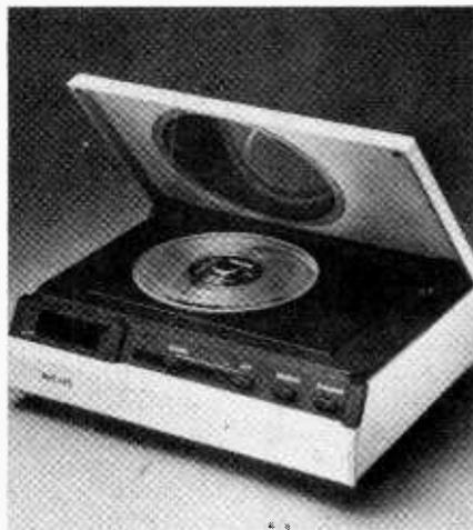
The demonstration prototype of the Philips Compact Disc player looks rather plain for the forerunner of an audio revolution. The controls parallel those of a regular record player except for the search controls.
