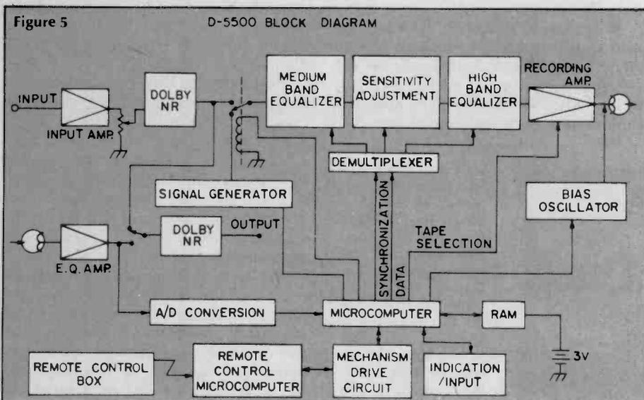
The microcomputer is the heart of the D-5500's systems. It automatically controls the test sequence and determines the correct bias level. The computer has two microprocessors.
