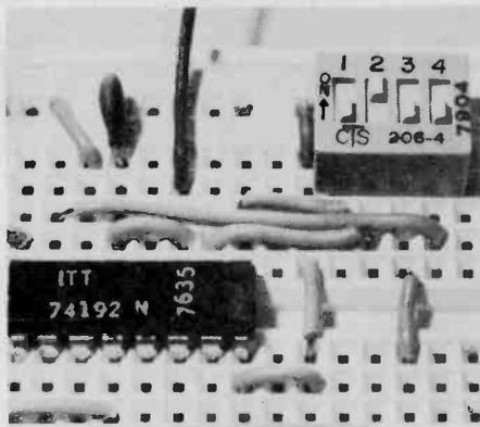
The heart of the circuit is the 74192 IC chip and the DIP switch that controls it.
