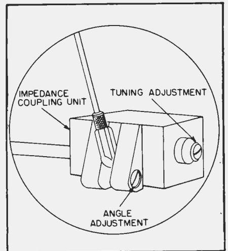
The coupling unit of the Avanti AH 151.3G includes a tuning adjustment, working it into the tuned circuit, can lower the SWR.
