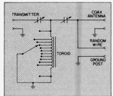
Fig. 2. This is a simple schematic for an antenna tuner showing the tapped inductor, and outputs for longwire and coax-fed antennas. You can see that this is based on example B in Figure 1. This is probably the most popular design for the smaller types of commercial antenna tuners sold.
