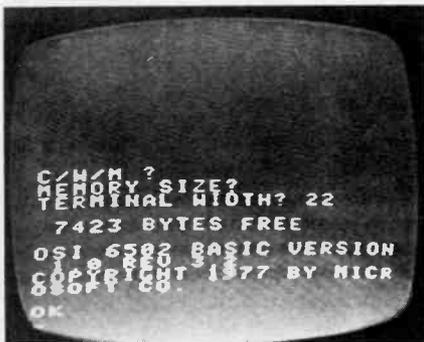
Overscanning, shown in the top photo, is easily cured by setting a shorter terminal width that will fit on the screen being used.
