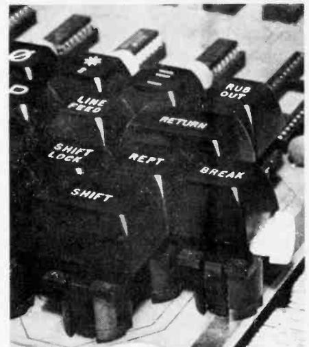
The BREAK key is just too easy for a hunt-and-peck typist to hit at the wrong time. Wedge a small piece of plastic under it.
