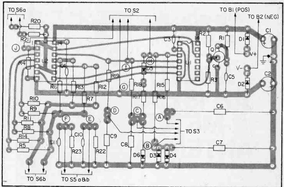
This is the component location guide used with the printed circuit board. Just about all of the components used in Imagician, with the exception of the switches, jacks and R24, are mounted directly on the board. Use IC sockets and be sure to orient them properly. Take special note of the takeoff points that lead away to the switches.
