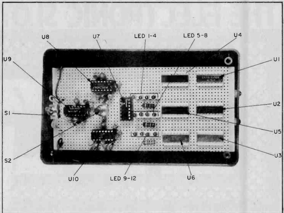
We cut some surplus DIP sockets in half to hold the rows of LEDs. If you don't care to ruin your sockets, wire the LEDs directly to the perfboard, using tie points to raise the LEDs up off the surface of the board so that they can protrude through the faceplate.
