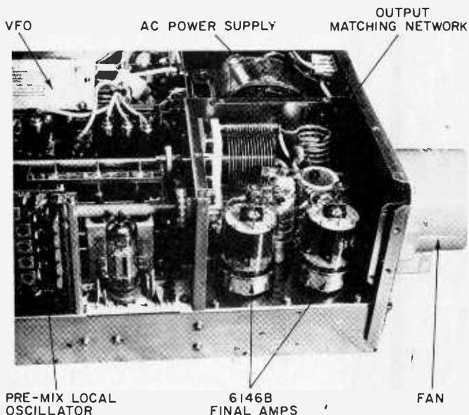
This closeup photo of the business end of the Yaesu FT 101ZD shows the two rugged 6146B final amplifiers nestled next to their pi-network at the right rear of the rig. In this photo, we've already installed the optional cooling fan through the rear chassis wall. We consider the fan a "must" option to protect the finals from overheating. The integral AC power supply is seen in the top right.
