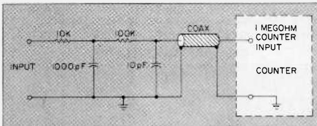
Here, the two cut-off frequencies are arbitrarily chosen at 10 kilohertz and 100 kilohertz and may be changed by varying the resistor-capacitor combinations of (R<sub>1</sub>, C<sub>1</sub>) and (R<sub>2</sub>, C<sub>2</sub>).
