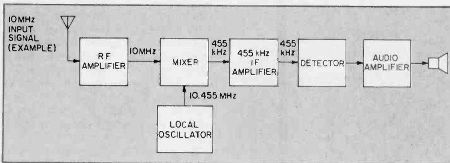
A single conversion receiver combines the incoming signal with the local oscillator's signal, to create a 455 kHz IF signal which can then be converted into an audio signal.
