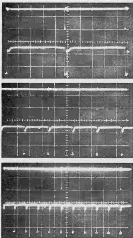
These three oscilloscope photos show the clock signal (top trace) and the resulting marker signal (bottom trace) for 100 kHz, 50 kHz and 20 kHz outputs respectively.
