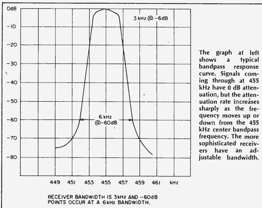
The graph at left shows a typical bandpass response curve. Signals coming through at 455 kHz have 0 dB attenuation, but the attenuation rate increases sharply as the frequency moves up or down from the 455 kHz center bandpass frequency. The more sophisticated receivers have an adjustable bandwidth.
