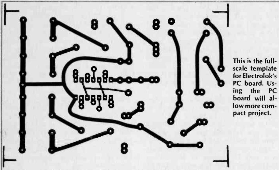
This is the full-scale template for Electrolok's PC board. Using the PC board will allow more compact project.
