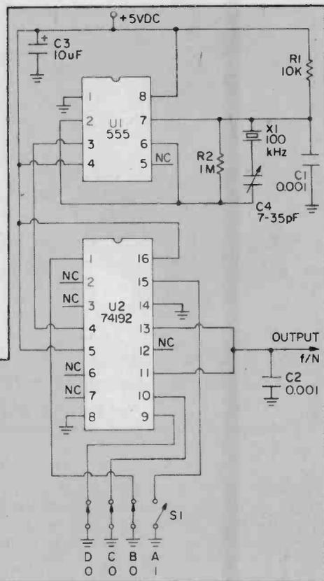
and begin to program other frequency divisions. Note for the 0010 (2-to-1) division to 50-kHz that you can now find an intermediate marker between the two previous 100-kHz positions. Go to a 4-to-1 division and you will hear tones each 25-kHz over the 100-kHz section of the spectrum. Try vari-
