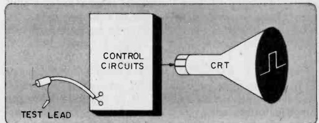
The signal voltage size is indicated by the *amplitude* (height, up-and-down dimension) of the beam movement on the screen. The *time period* (duration) is shown by the distance the beam travels across the screen horizontally, from left to right.
