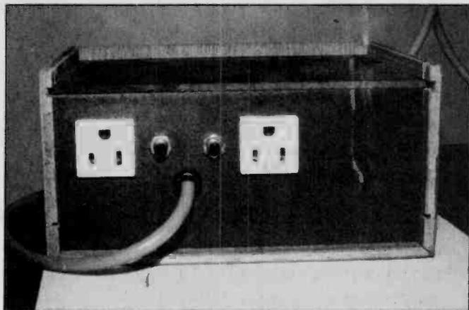
The back of the Remote unit shows the two relay-switched AC outlets. They are also controllable by means of two pushbutton switches, so the operator can manually override the computer without entering new commands or returning to the terminal.
