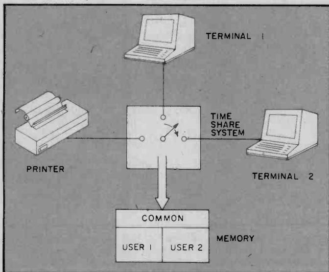
In a time sharing system various terminals, printers and other "slow" peripherals share the use of a single computer to enable more efficient use of the machine. This requires a special operating system to keep the different inputs and programs sorted.
