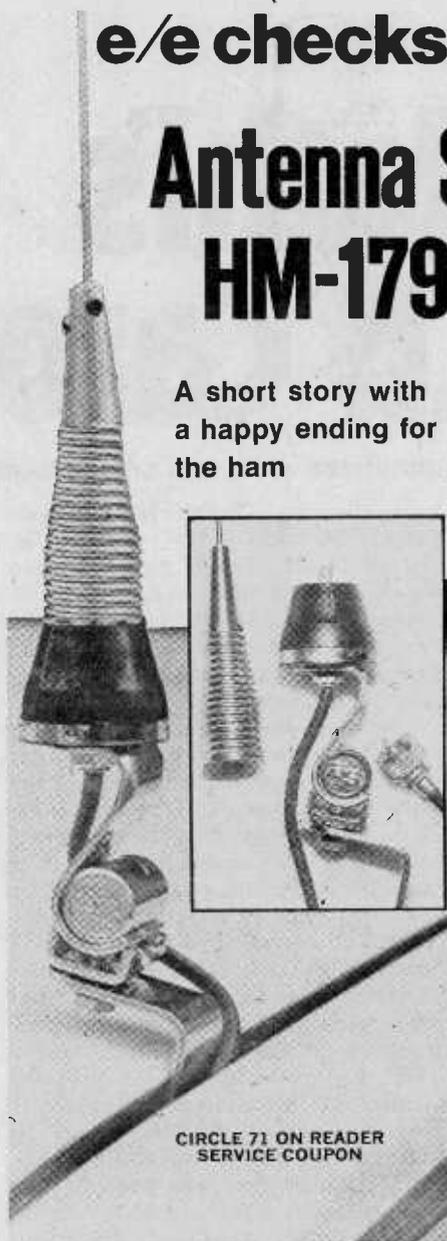
perform electronically in the same manner? With the SWR meter in line, it was an easy matter to check the broad-bandedness of the antenna by dialing up frequencies on the synthesizer at each extreme of the band. At 146 MHz, the frequency to which we had cut the whip, the SWR was not enough above 1:1 to budge the needle on the meter. In fact, at both 144.000 and again at 147.995, the SWR never exceeded 1.4:1. That, friends, is called "flat."
