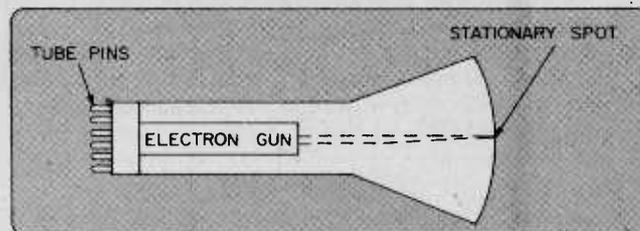
By varying the voltage between the two vertical-deflection plates, the spot on the face of the tube can be made to move up and down. The distance will be proportional to the change in voltage between the plates. Changing the voltage difference between the
