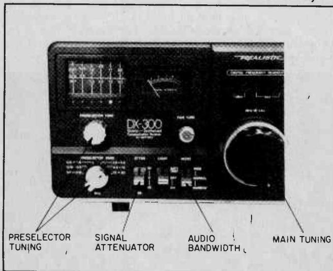
After a little practice, you can zero the DX-300 in on any band in a second or two. The preselector is really sharp, and helps to attenuate unwanted off-frequency signals. The audio bandwidth control can really sort out a signal when two or more are bunched.
