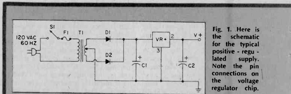
Fig. 1. Here is the schematic for the typical positive-regulated supply. Note the pin connections on the voltage regulator chip.
