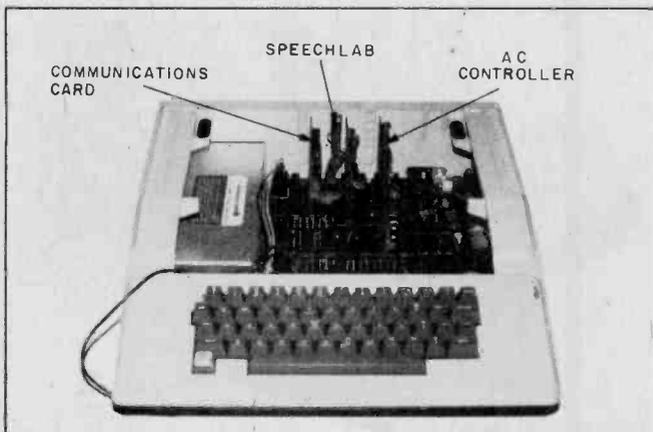
Both the Heuristics *Speechlab* vocal encoder, and the *AC Controller* by Mountain Hardware, are available in configurations suitable for use with the Apple II computer, as well as the many S-100 bus computers available on the home computer market.
