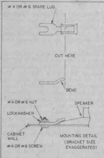
Here's a novel way to mount subminiature speakers that don't have tabs for mounting screws. A few spade lugs bent to the proper angle will solve the problem. You might use this same method (on a larger scale, of course) to flush-mount speakers in your car, where space doesn't allow for running screws through the mounting tabs in the speaker frame, as on door mounts.
