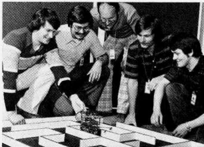
The Moonlight Special has optical sensors that follow the walls and indicate obstacles.
