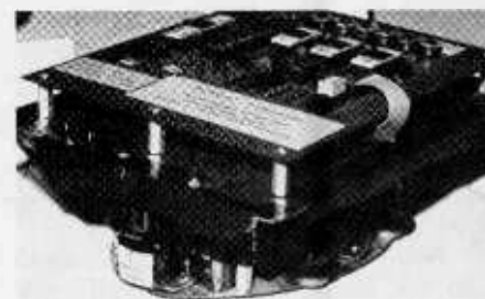
The Berkeley Micro-mouse used an optical sensor and bumpers to find its way through.
