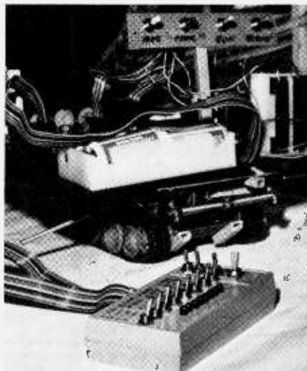
This programmable mouse can be told how to get through the maze by pre-instruction.
