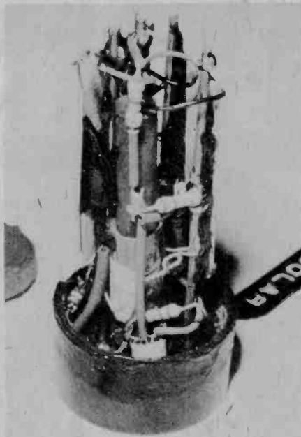
The photo cells are mounted on two sides of the frame. The loop stick fits neatly in the middle of all the components. The transistors are in the base of the tube. Wire support number 8 is used only as a wiring tie-point for the small components. All other support terminals will be tied into the circuit after the tube socket is bolted to the wooden base.
