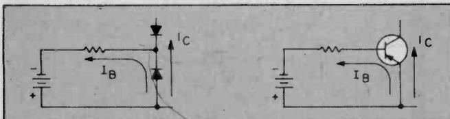
Note how the battery polarity is reversed and the current flows in the opposite directions through the diodes.
