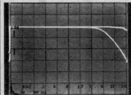
This 'scope shot shows how the high frequency filter affects the top end of the spectrum. The signal is 10dB down at 15 kHz.
