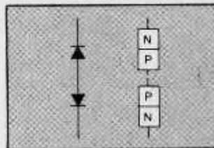
In its simplest form a transistor can be considered as two diodes, connected back to back, as in this drawing.
