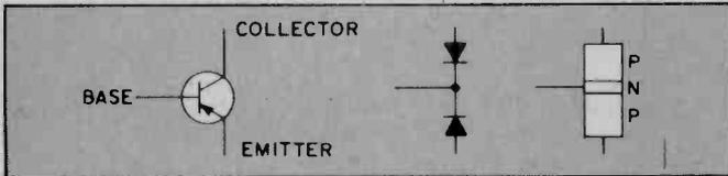
Both types, NPN and PNP, are made from either silicon or germanium.
