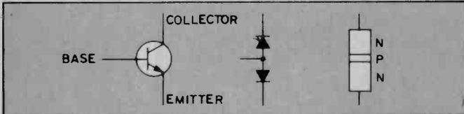
Because of the way the semiconductor materials are arranged, this is known as an NPN transistor. Which transistor terminal has the arrowhead? ..... the emitter
