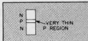
However, in the construction process one very important modification is made. Instead of two separate P regions as shown above only one very thin region is used.
