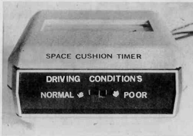
While almost any case can be used for the space cushion timer, this Radio Shack clock case seems ideal. This unit can be mounted at almost any convenient spot on the dashboard of your car.
