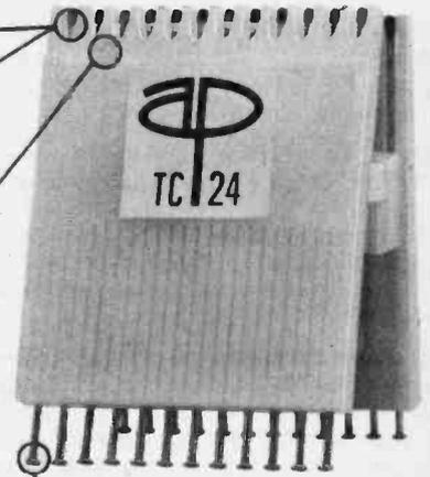
New button-head pins keep probes from sliding off. (Straight pin models for logical connections.)
