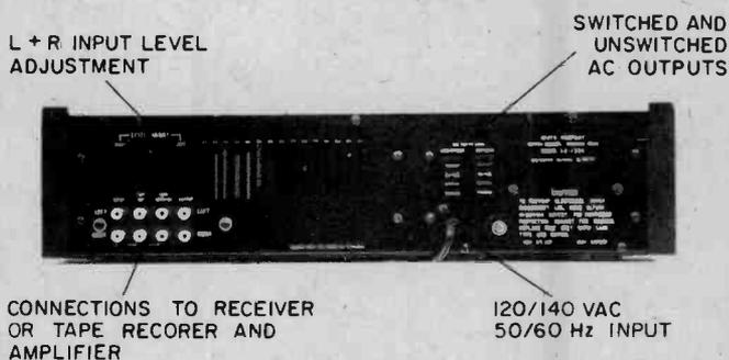
Since the processor will utilize a receiver's tape connections, the tape connections are moved to the processor along with the tape/source monitor switch. It can be built for 120 or 240 use.
