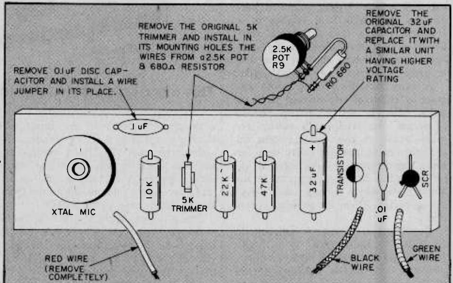
This pictorial diagram shows all the modifications that are needed on the S-210U module. The 32 uF capacitor should be replaced by one with a 16-VDC or higher voltage capacity.
