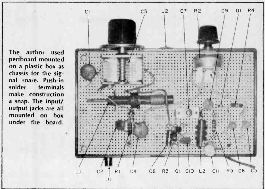
The author used perfboard mounted on a plastic box as chassis for the signal snare. Push-in solder terminals make construction a snap. The input/output jacks are all mounted on box under the board.
