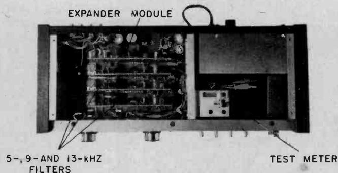
The expander and three filter modules plug into the main board assembly. The test meter is built into the cabinet and is used for circuit alignment during construction and for circuit testing.
