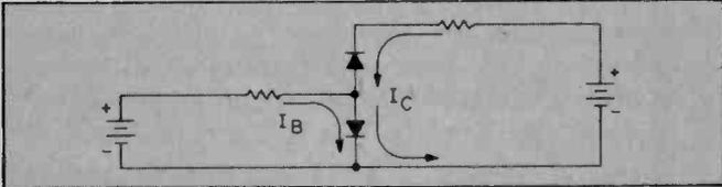
Base current ( $I_B$ ) flows through the base-emitter diode and causes the collector current ( $I_C$ ) to flow through the base-collector diode.
