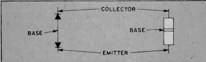
The two diodes are usually called the **base-emitter diode**, and the **base-collector diode**.
