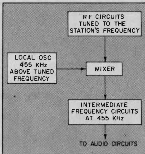
This block diagram shows how an image signal is formed. It will always be twice the intermediate frequency below the station. Double conversion receiver may cure image.
