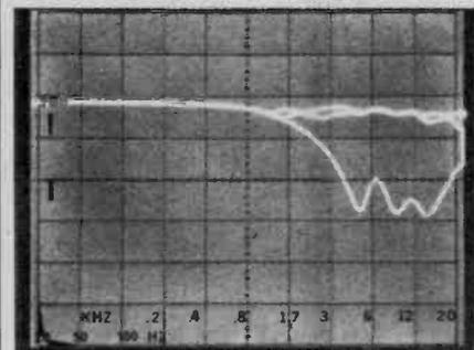
Here you can see the nulls of the 5-, 9- and 13-kHz dynamic noise filters. The top line shows when they are not activated.
