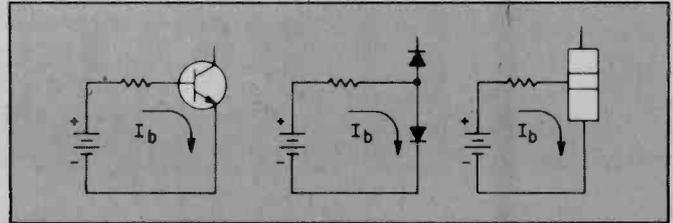
Would base current flow if the battery were reversed? Base current would not flow as the diode would be back biased.
