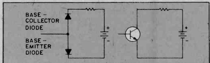
Will current flow in this circuit? Why or why not? It will not flow as the base-collector diode is reverse biased.
