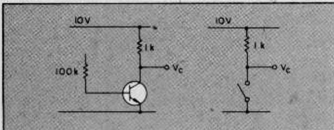
Since the base circuit is broken—that is, it is not complete—there is no base current flowing.
