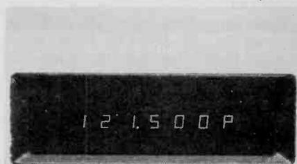
The L.E.D. frequency readout indicates the channel or received (searched) frequency. The letter “P” following the frequency indicates it is one of two user-programmed priority channels. An “L” following the frequency indicates the user has locked that channel out of the SCAN, though it can be manually selected. A letter “d” following the frequency indicates that a 2-second delay has been programmed before scanning resumes after the station carrier goes off.
