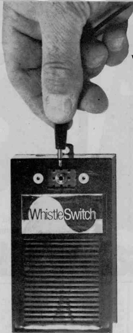
Here, the new control jack is shown installed in place of the original AC outlet. We strongly suggest the use of a miniature jack, as clearance under the cover is severely limited. Use a thin flexible wire to connect the jack to the PC board.
