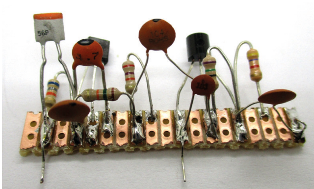
Figure 4.42: Construction of the active stage.
