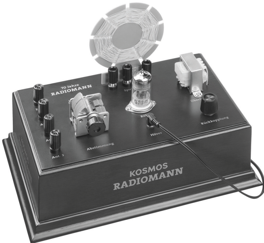
Figure 3.10: The Kosmos-Radiomann kit fitted with a medium wave coil installed.
