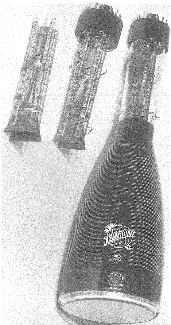
Figure 4.56 Tektronix T54 and electron guns (1956). (Courtesy of Tektronix, Inc.)
