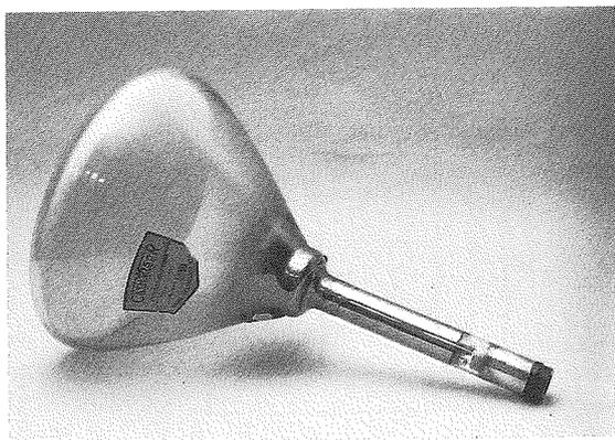
Figure 5.3 Baird 12MW2 Cathovisor of 1939. (Courtesy of C. E. "Sonny" Clutter.)
