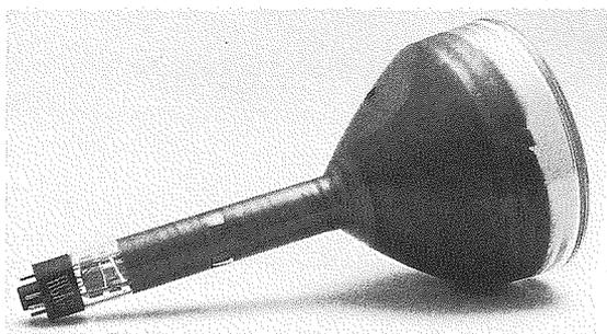
Figure 5.12 RCA 7DP4 of 1946. (Courtesy of C. E. "Sonny" Clutter.)
