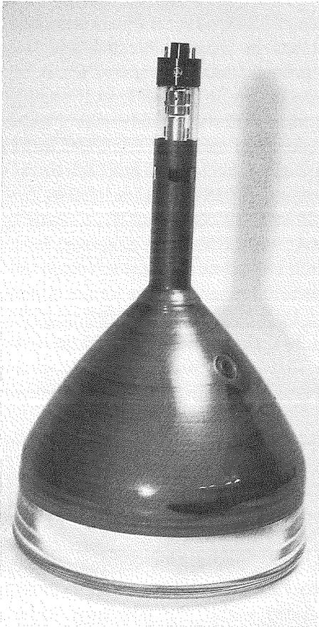
*Figure 3.14 RCA 10KP7 magnetic deflection radar CRT manufactured in 1954. (From the author's collection.)*
