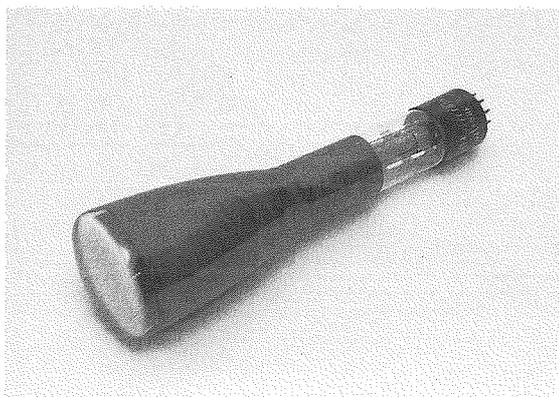
Figure 5.9 RCA 3KP4 electrostatic deflection picture tube manufactured in 1948. (Courtesy of James Richardson.)
