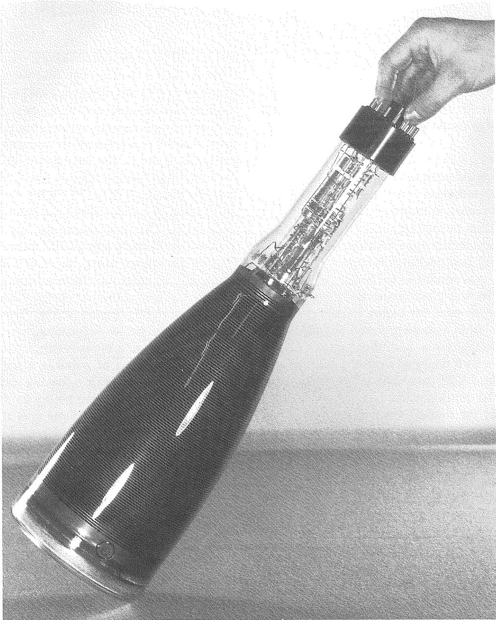
Figure 4.49 Tektronix T551 dual-beam, spiral accelerator CRT of 1958. (Courtesy of Tektronix, Inc.)
