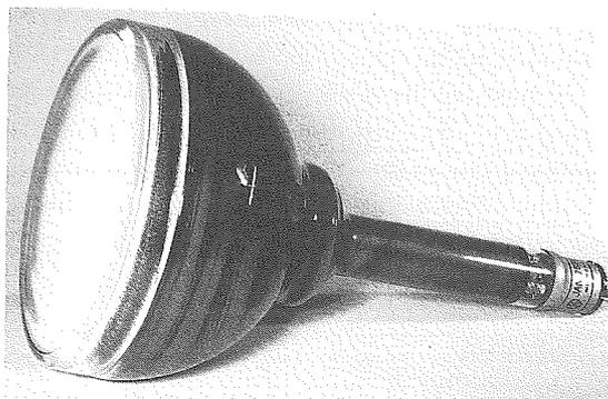
Figure 3.12 General Electric 7BP7 magnetic deflection radar CRT circa 1944. (From the author's collection.)
