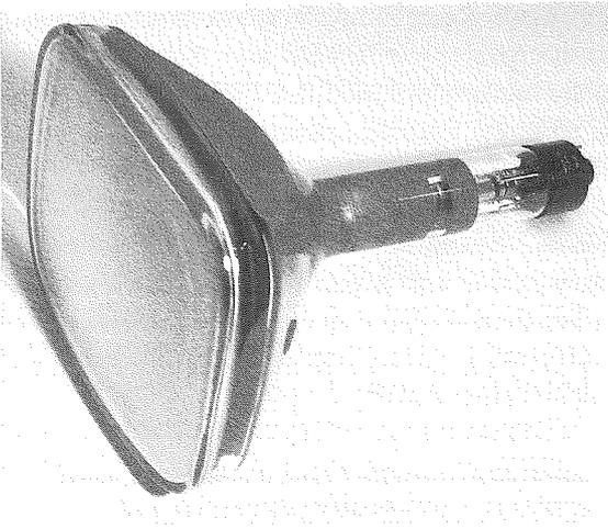
*Figure 5.38 RCA 8DP4 employing 90-degree deflection to greatly shorten the funnel. Example manufactured in 1956. (Courtesy of James Richardson.)*
