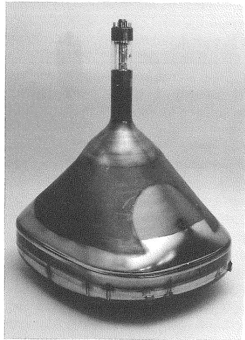
Figure 6.22 Westinghouse 22EP22 rectangular glass color picture tube of 1956. (Courtesy of James Richardson.)
