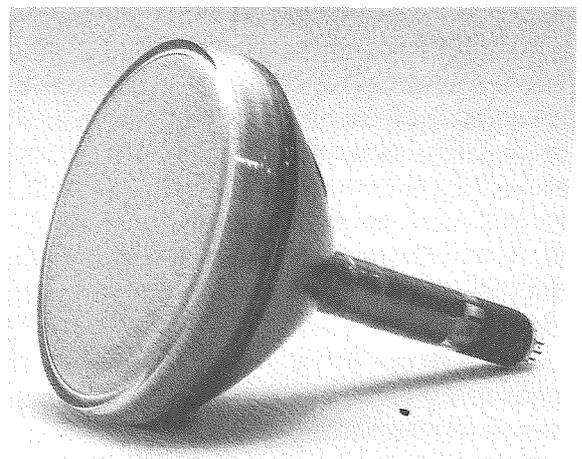
Figure 8.5 Thomas Electronics 5BCP7 short radar CRT. (Courtesy of Jake Brain.)
