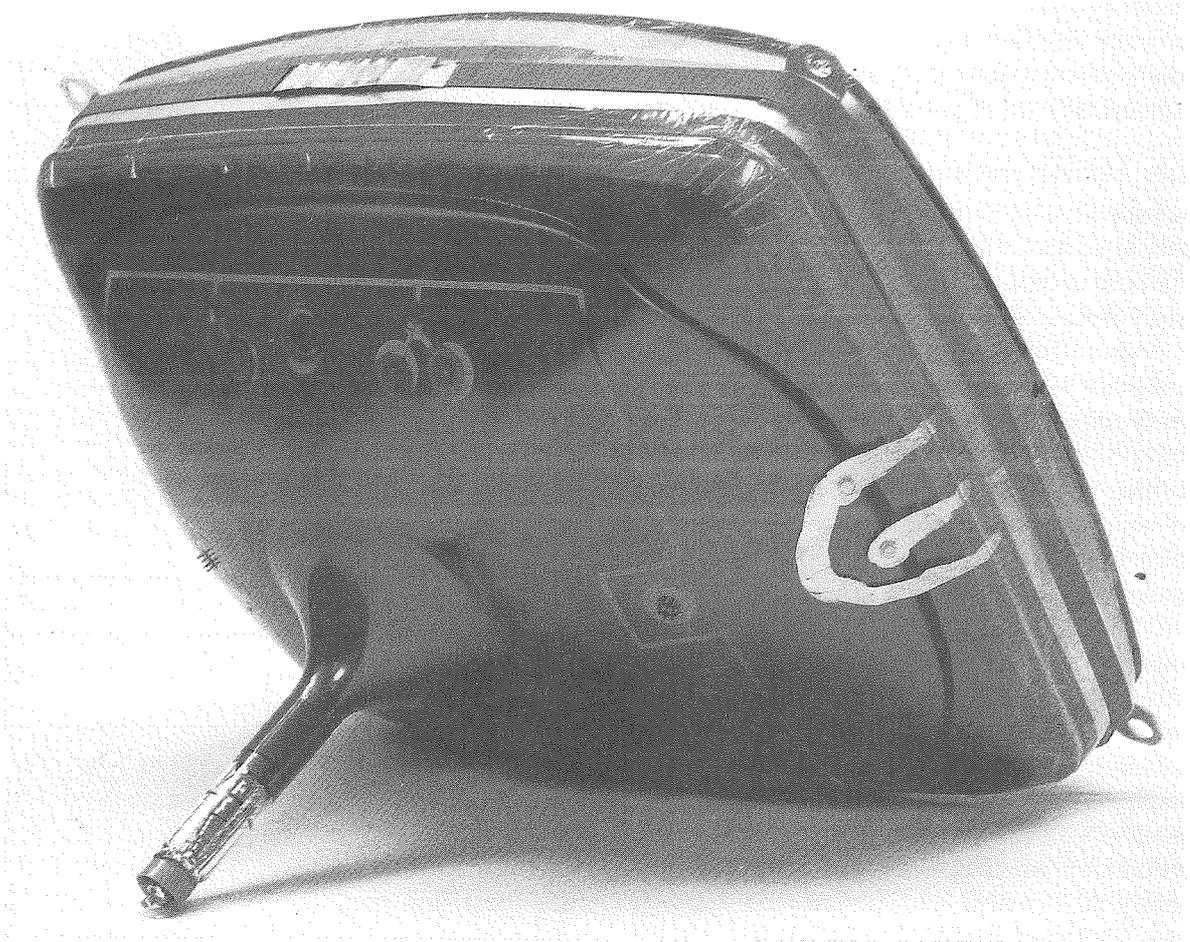
Figure 7.6 Tektronix T4016 25-inch storage tube. (Courtesy of Tektronix Inc.)
