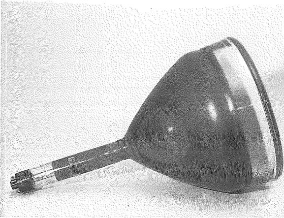
Figure 1.1 RCA Victor 10BP4 electromagnetic-deflection and focus cathode-ray tube, circa 1946. (From the author's collection.)
