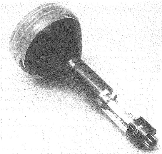
Figure 8.4 Du Mont 5FP7-A radar CRT manufactured in 1957. (From the author's collection.)
