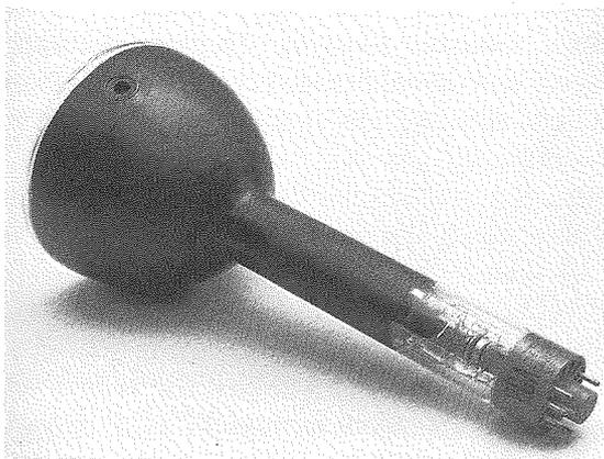
Figure 5.19 RCA 5TP4 projection kinescope manufactured in 1954. (Courtesy of C. E. "Sonny" Clutter.)
