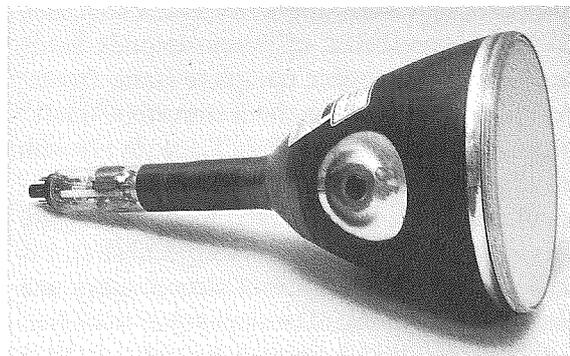
Figure 9.11 Thomas Electronics 7M280 seven-inch film recorder CRT.
