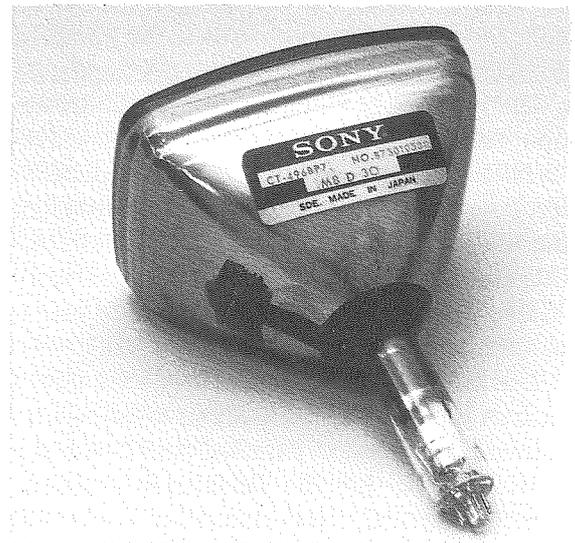
*Figure 5.49 Sony five-inch CRT as used in portable television receivers. (Courtesy of James Richardson.)*
