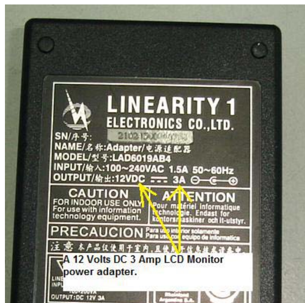
The specification of a LCD Monitor power adapter
