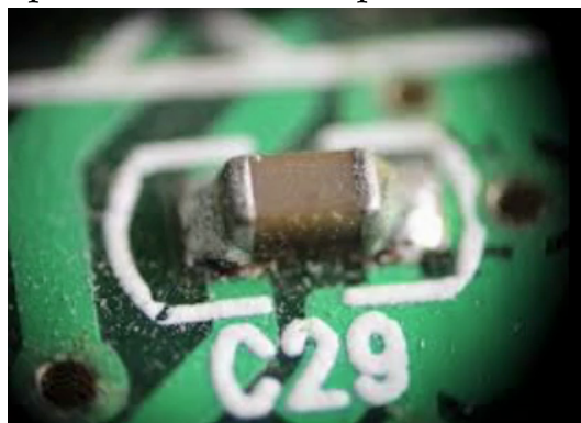
Figure 1.3: A surface-mounted component attached to a PCB.
