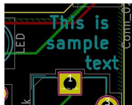
Figure 28.9: The text appears in three lines, justified to the right..
