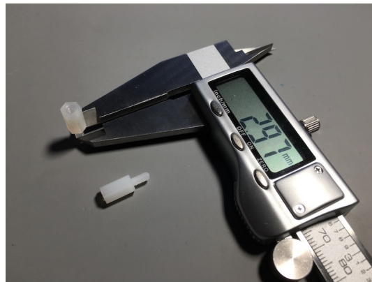
Figure 9.62: Measuring sizes with a calliper is easy and accurate.
