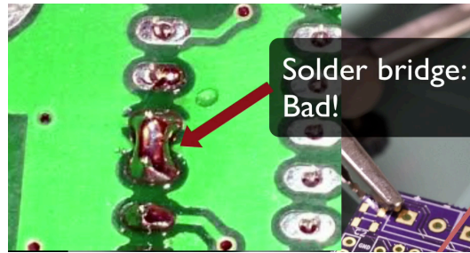
Figure 1.6: A solder bridge like this one is a defect that solder mask helps in preventing.
