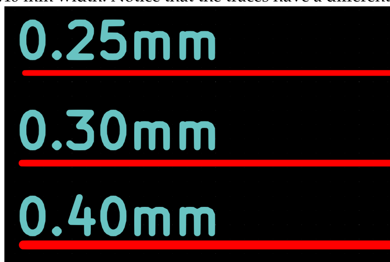
Figure 26.5: Three traces with different widths.
