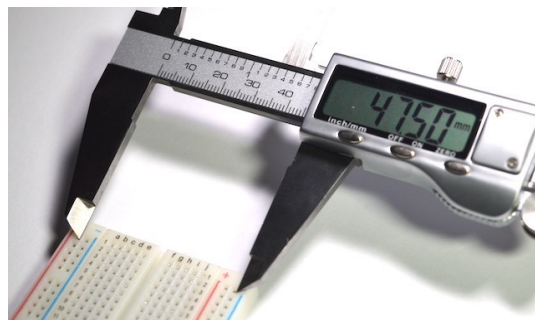
Figure 17.49: The distance between the top and bottom rows is critical for this project.
