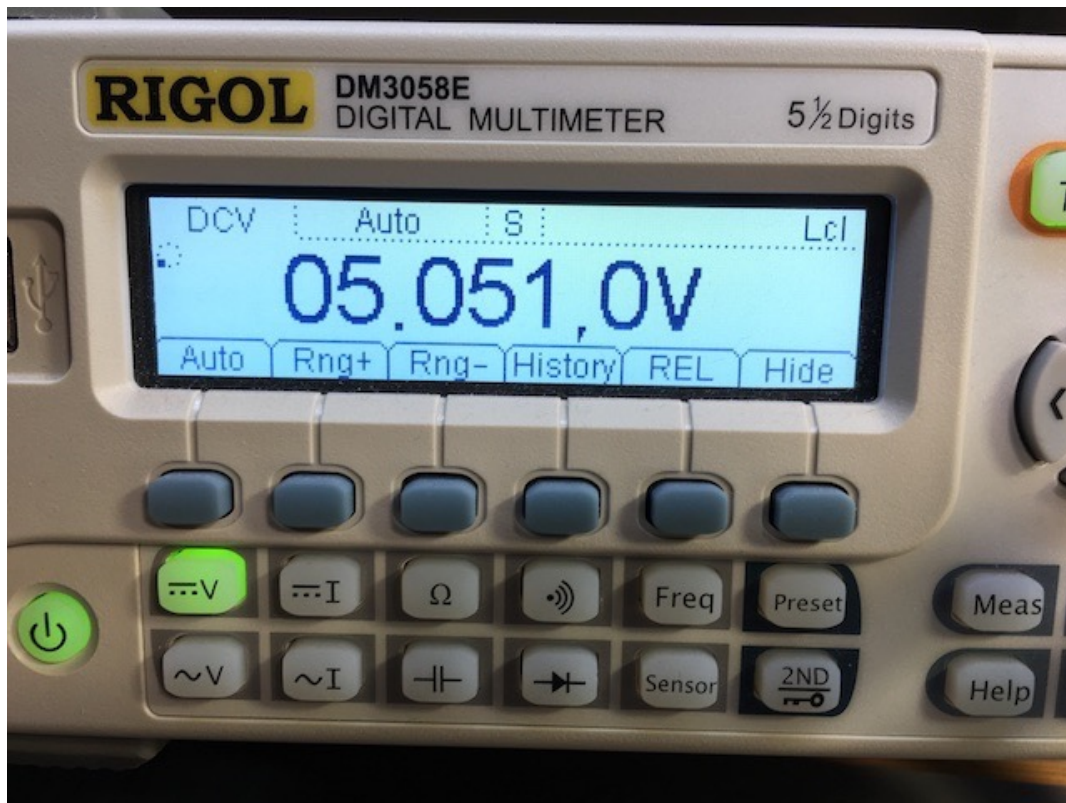
Figure 17.6: Actual output voltage, when input power comes from a 9 V DC mains power supply.
