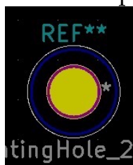
Figure 9.67: When duplicating a footprint using Ctrl-D, take care to place the mouse pointer on the yellow line.
