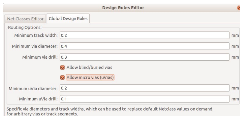
Figure 48.4: Enable blind and micro vias.
