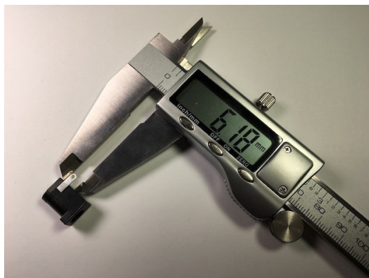
Figure 17.21: The distance between two of the connector pins is 6.18 mm.
