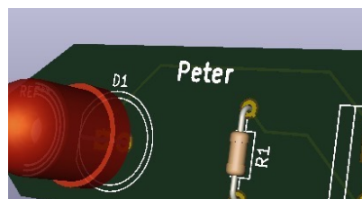
Figure 9.83: Top silk screen with additional text.
