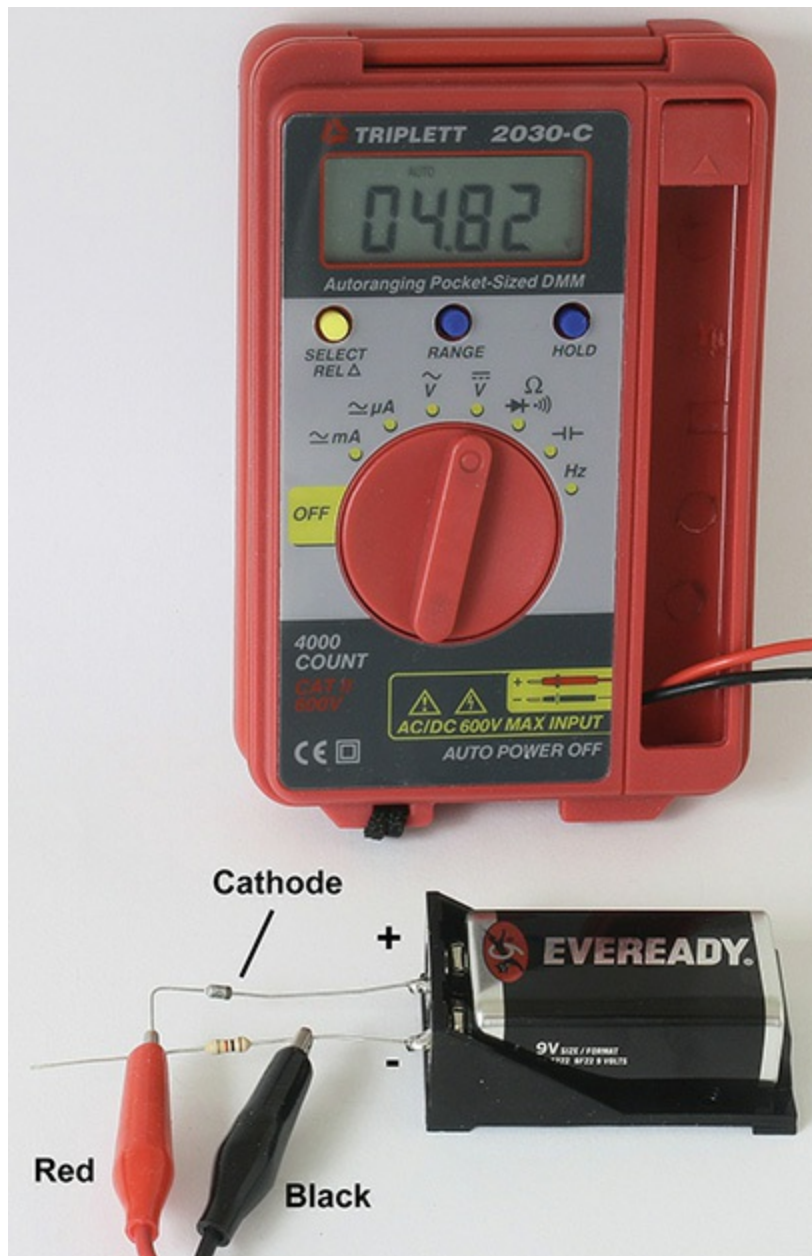
FIGURE 5.17 A 4.3-volt 1N749A, 400 mW Zener diode is connected in series with a resistor to drop or subtract 4.3 volts from the 9-volt battery.
