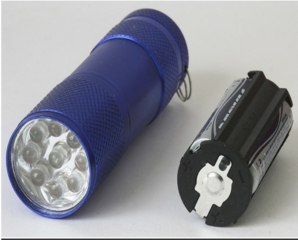
FIGURE 6.8 A three AAA cell 9 LED flashlight, where the LEDs are matched in terms of turn-on voltage.
