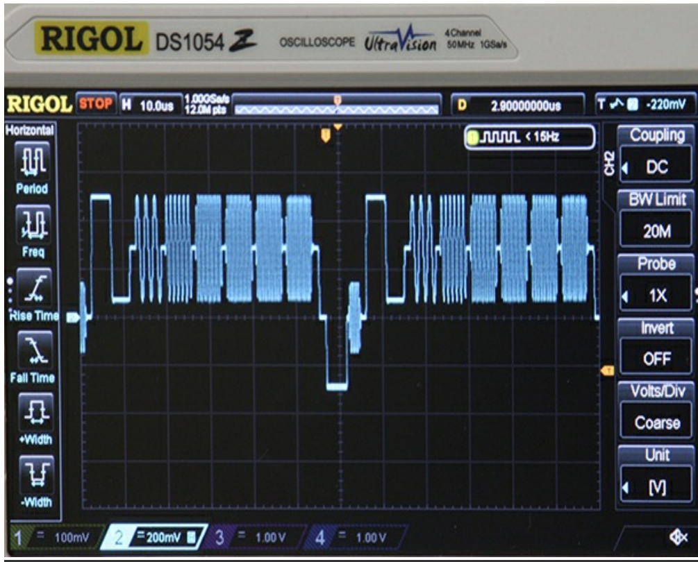
FIGURE A-8 Rigol 480x800-pixel display but with 12M points gives a better looking waveform.
