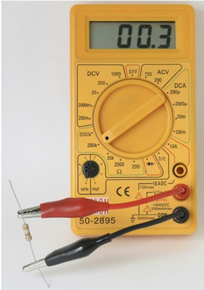
FIGURE 4.21 At the 200kΩ setting, the DVM is “looking” for resistors in the 10kΩ range. So the 390Ω resistor is measured as 0.3kΩ = 300Ω. Note that we are further losing measurement accuracy.
