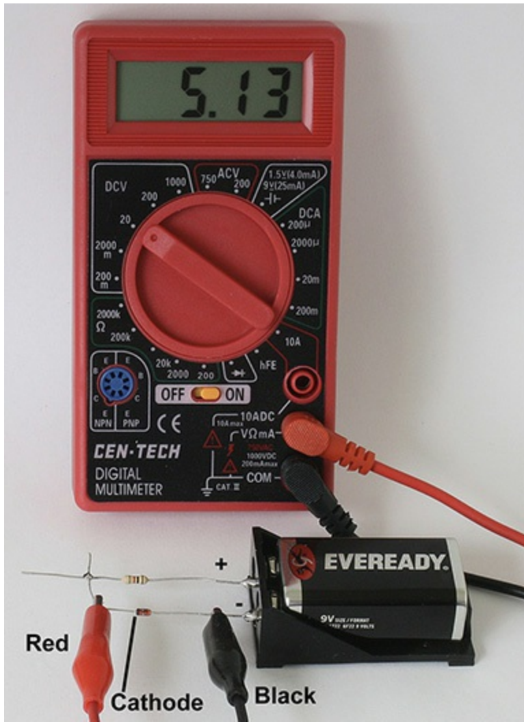
FIGURE 5.19 A 5.1-volt 1N751 400 mW Zener diode configured as a “shunt” regulator circuit that provides 5.13 volts as shown in the DVM. The red lead is on the cathode.
