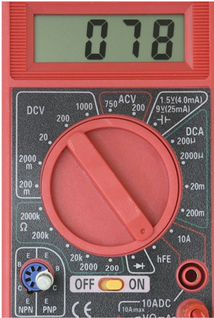
FIGURE 7.4 A TO-18 transistor with its emitter tab pointed up toward “E” with the DVM selector knob set to h_{FE} . Here, we see the transistor has a current gain, h_{FE} = 78 .
