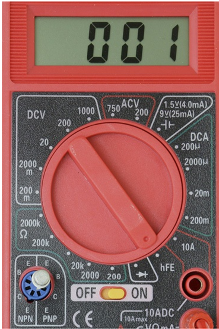
FIGURE 7.5 The same transistor tested “backwards” with the emitter inserted in the collector, C, portion of the socket and the transistor’s collector lead inserted into the E portion of the socket. Note that the tab that identifies the emitter is pointing down. The resulting current gain is very low at h_{FE} = 1 when the transistor is wired backwards this way.
