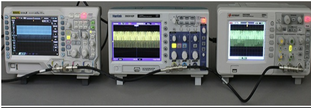
FIGURE A-10 From left to right: Rigol (12M points), Hantek (40K points), and Rigol (32K points), and all three oscilloscopes are set to the “Stop” mode to store the waveform. Only the Rigol (on the left side) with 12 million memory points seems to display the test signal properly at 200 \mu\text{sec}/\text{div} . The other two have random gaps in the waveform that are caused by sub-Nyquist sampling.
