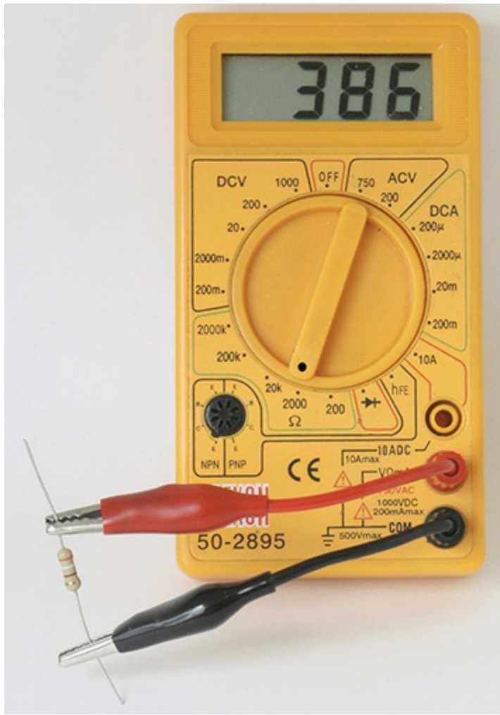
FIGURE 4.19 At the DVM's 2000Ω setting we see a reading of 386Ω for the 390Ω resistor.
