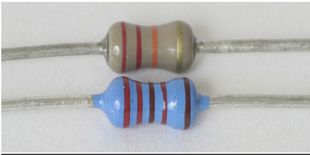
FIGURE 4.16 A 22\text{K}\Omega , 5 percent resistor on the top and 22.1\text{K}\Omega , 1 percent resistor on the bottom. Note that the fifth band that denotes tolerance rating is closest to the edge in the 1 percent resistor, and it has wider spacing between the adjacent fourth band.
