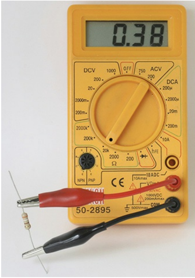
FIGURE 4.20 With the DVM's 20kΩ setting, the DVM is displaying in kilo-ohms. The 390Ω resistor is measured as 0.38kΩ = 380Ω. Note that we just lost some accuracy compared to Figure 4-19 , which measured 386Ω.
