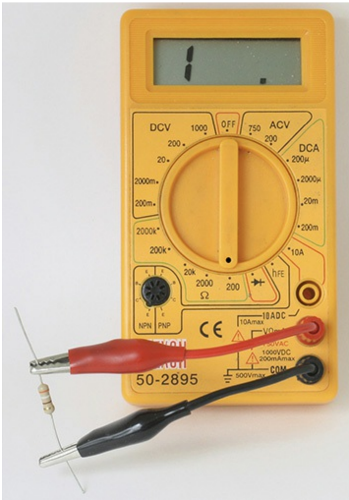
FIGURE 4.18 The 390Ω resistor shows a “1” and blank digits indicating “out of range” at the DVM’s 200Ω setting.
