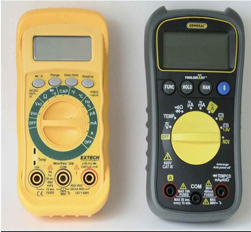
FIGURE 3.6 Two auto ranging DVMs by the Extech MN26 and General Tools and Instruments model TSo4. Note: Extech replaced the MN26 with the MN36 DVM.
