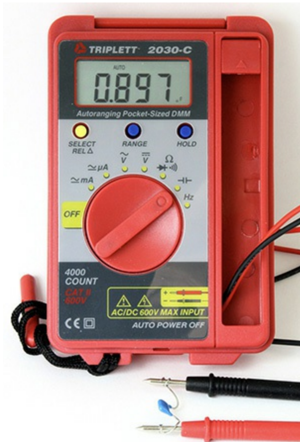
FIGURE 4.5 Measuring a 1 \mu\text{f} (105M) capacitor with an auto-ranging DVM that reads 0.897 \mu\text{f} .
