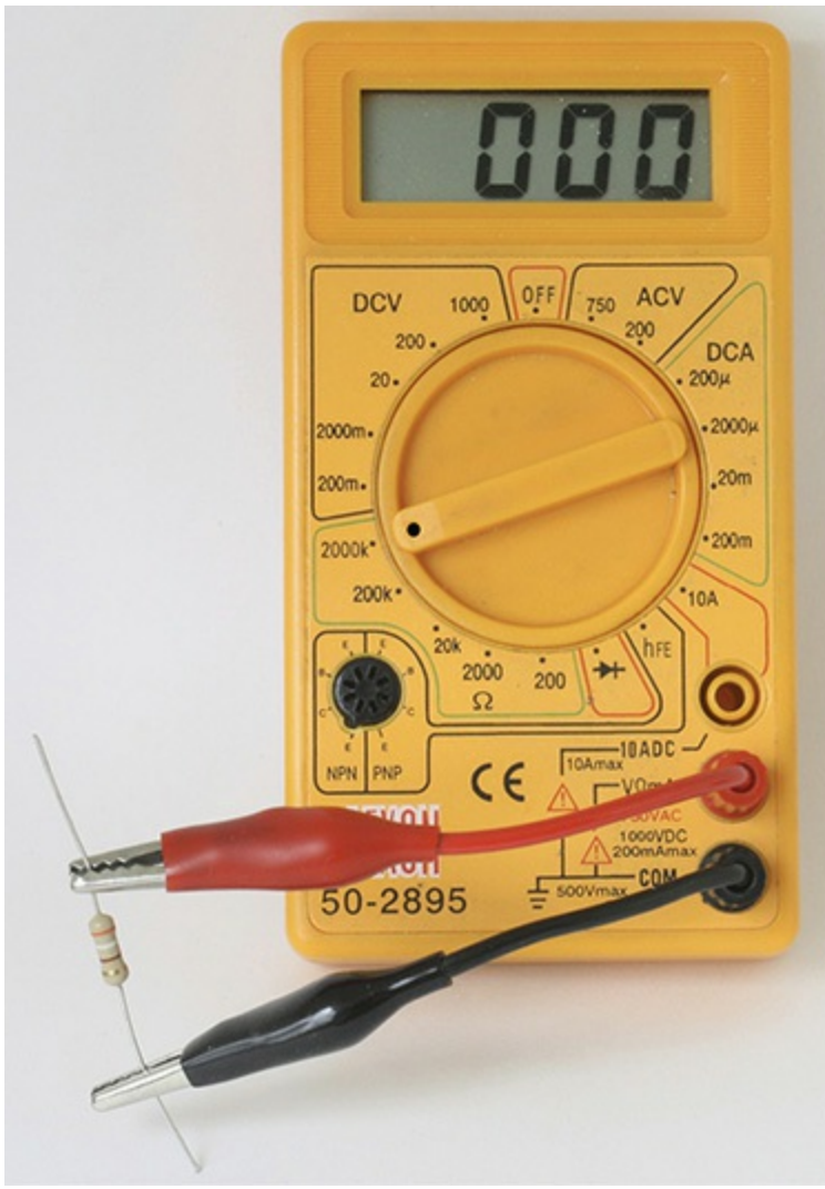
FIGURE 4.22 With the DVM's resistance set to 2000k \Omega or 2M \Omega , it is expecting resistance values in the 100k \Omega range. And with this setting it cannot resolve measuring resistances below 1000 \Omega . Any resistor value below 1000 \Omega , such as 390 \Omega , will register as zero as shown above.
