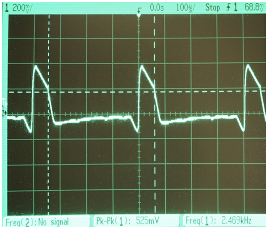
FIGURE 14.29 V_{out} of the circuit in Figure 14-28(a) , an oscillating waveform at about 2.5 kHz, which is the incorrect frequency since the crystal is at 3.00 MHz.
