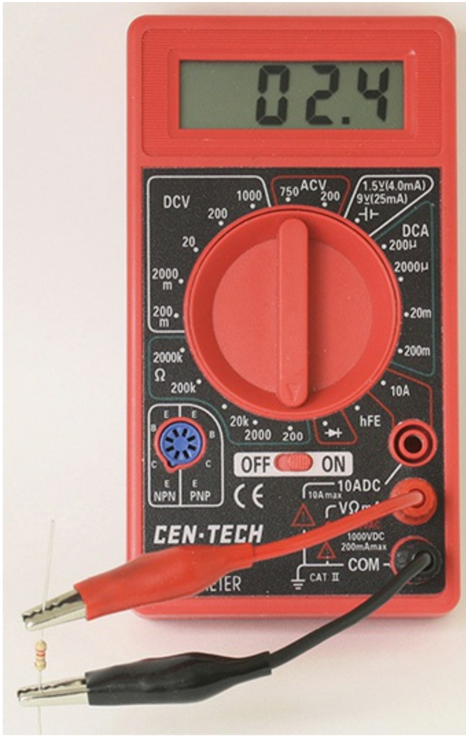
FIGURE 4.24 The combined test leads' resistance ( 0.2\Omega ) with the 2.2\Omega resistor is 2.4\Omega .
