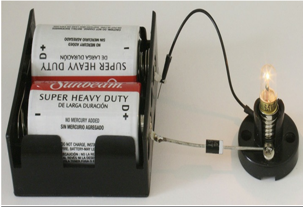
FIGURE 5.6 Positive terminal of battery is connected to the diode's anode to enable the diode into forward bias conduction that supplies current to the lit lamp.
