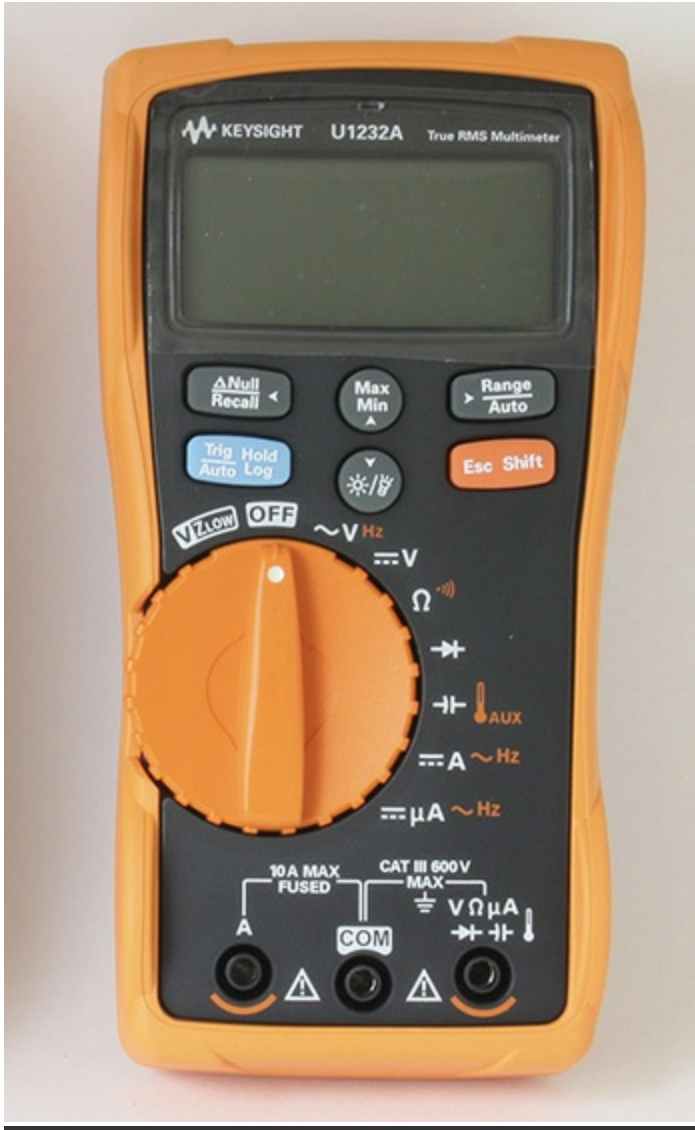
FIGURE 4.25 Keysight U1232A DVM with the \Delta Null/Recall button and to the right of it, the Max Min key.
