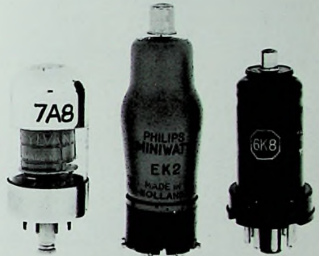
American 7A8 octode (L.), Philips EK2 octode and American 6K8 triode-hexode (R.).
