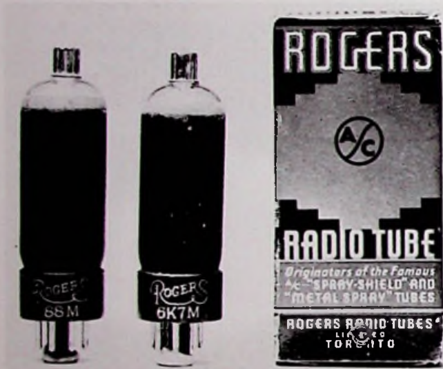
Rogers 'Metal Spray' tubes. Note corrugated grid caps.
