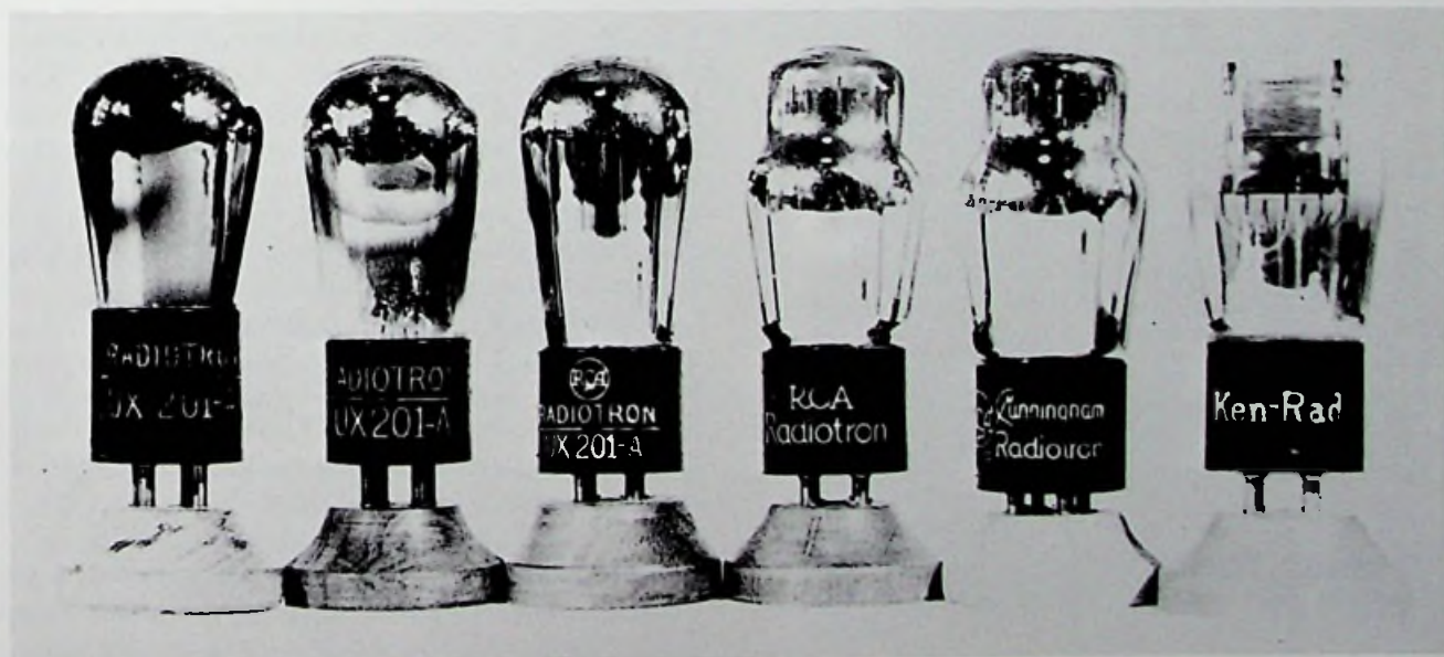
The '01-A story—the final issue had an oxide-coated filament.
