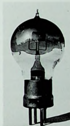
Example of the original French 4-pin metal base.
