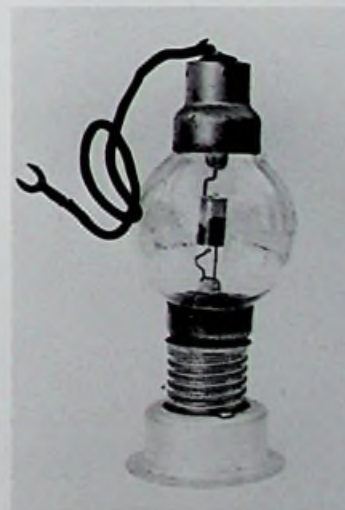
Cossor U.3 half-wave rectifier c. 1922.
