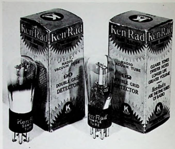
Types 90 and 92. Note base markings 'sample tube.'
