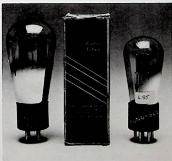
Tung-Sol TS280 (L.) and 485 (R.). The latter is a Sparton replacement.
