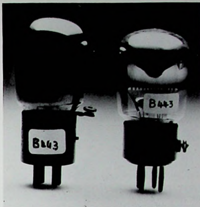
Philips Type B443. The world's first pentodes (1928).
