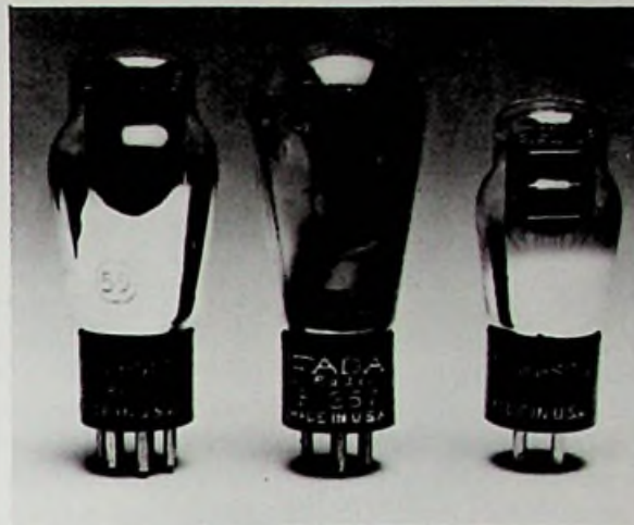
Tung-Sol 59 (L.) and 71A (R.). The centre tube is an F257 made for Fada.
