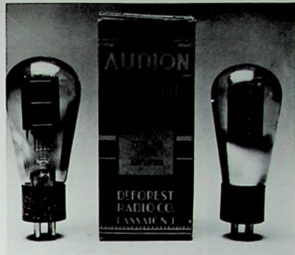
De Forest types 410 and 510. The 510 is a transmitting tube.
