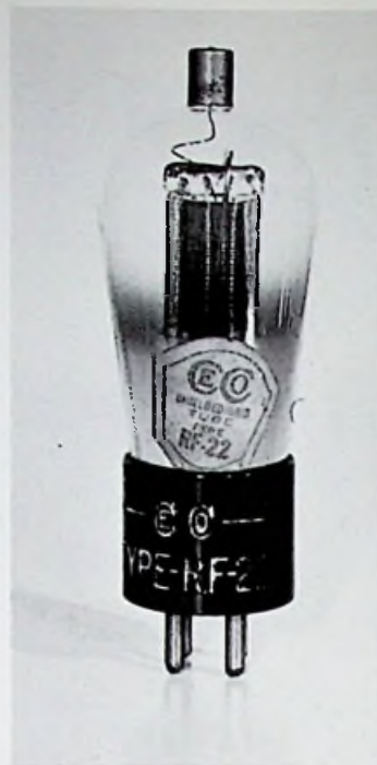
CeCo type RF22, equivalent to Radiotron UX-222.
