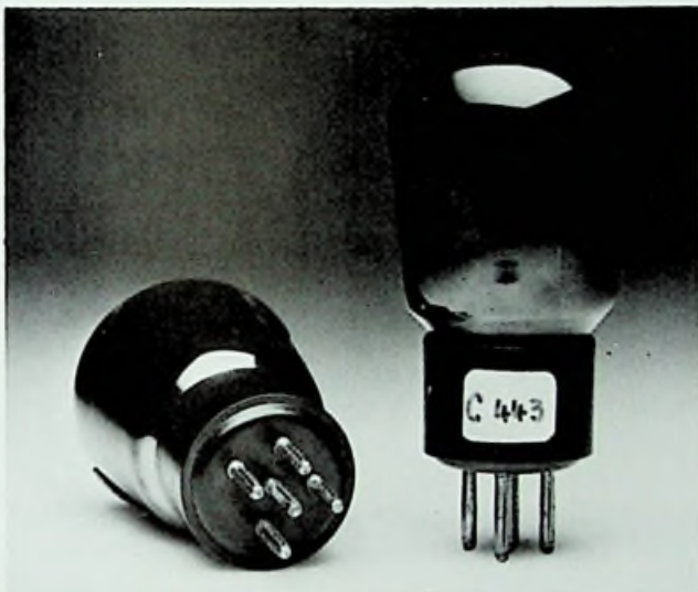
The standardised European 5-pin base introduced in 1929.
