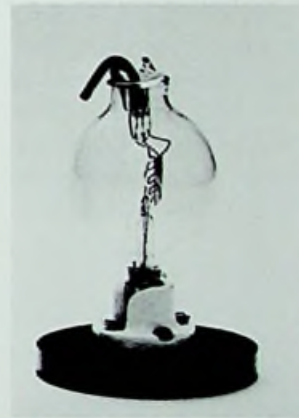
Single-wing Audion 1908, note spare filament lead.
