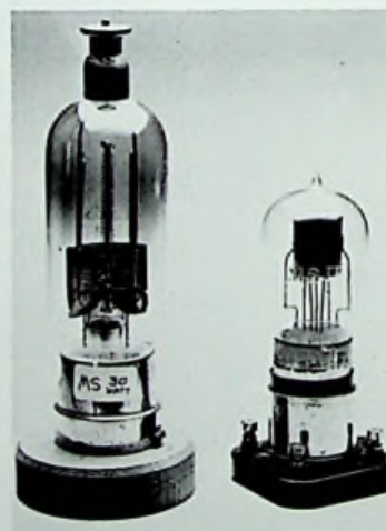
(L.) German Mueller 'MS' 30-watt. (R.) Mueller MSIV 5-watt c. 1926.
