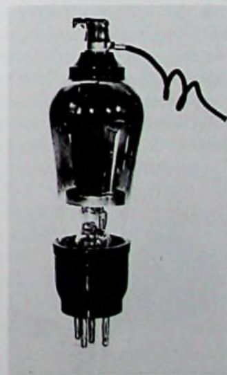
Osram VMS4 valve using hybrid top connector (1933).
