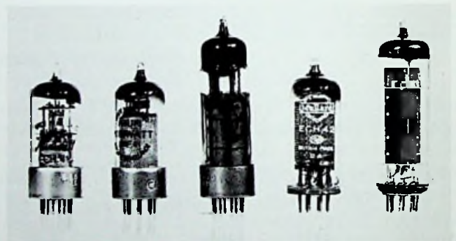
A group of Philips-Mullard 'Rimlock' valves. The earliest types had metal base shells.
