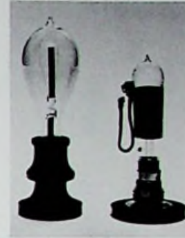
Replica of an Edison 110-volt carbon-filament lamp compared with a commercial version of a Fleming diode.
