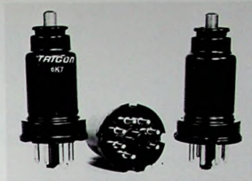
Russian metal tubes carrying markings of a British distributor c. 1958.
