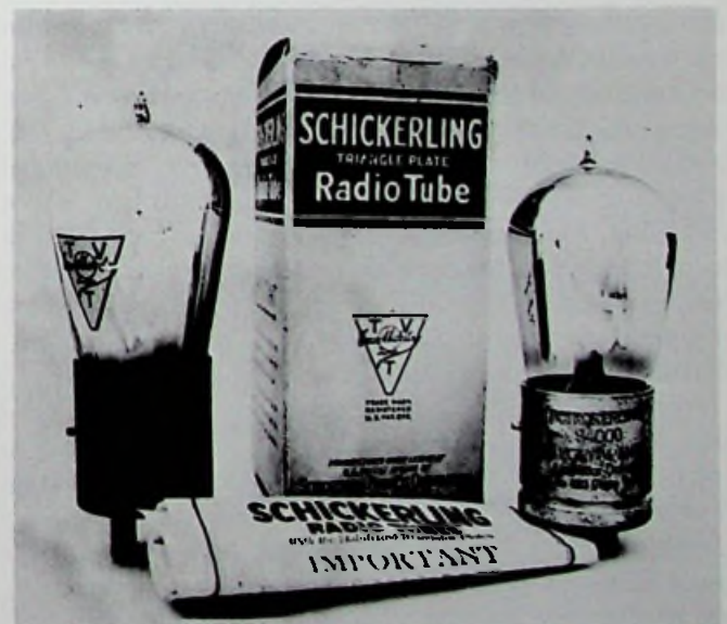
Schickerling SX400 and S-4000 typical 'bootleg' tubes of the 1920s.
