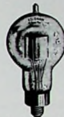
One Type of High Power Rectifier.
