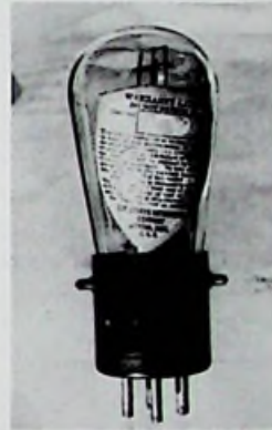
Sparton AC tube with side connections for heater wiring. 1927.
