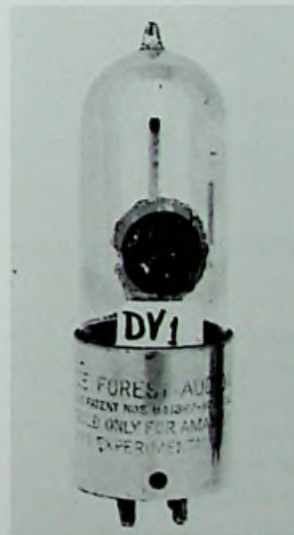
Example of a Shaw 4-pin base used on a De Forest type DV1 tube c. 1923.
