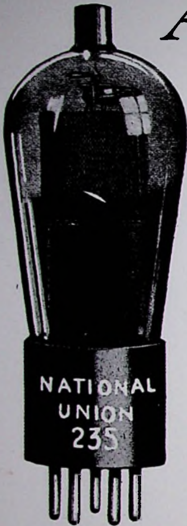
A remote cut-off screen-grid valve especially designed for operation as an R.F. or I.F. amplifier. Its particular merit is its ability to amplify without introducing disagreeable cross-talk or distortion. This valve will be used by set designers in many of their new models. It, however, should not be used to replace type 224 valves in sets originally designed for the 224 valve.
