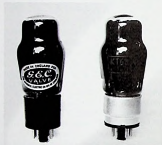
Osram KT63, the later version is on the right.
