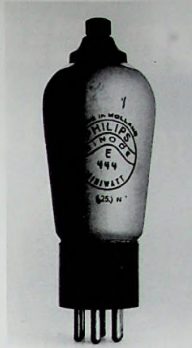
Philips E444 'Binode' fitted with American 6-pin base.
