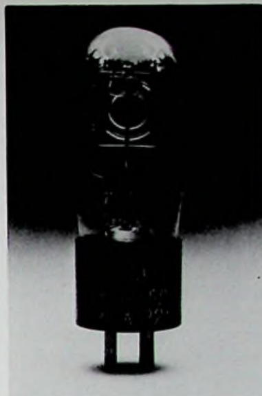
RCA-221. The 'export only' tube. Filament rating was 5V, 0.06A.
