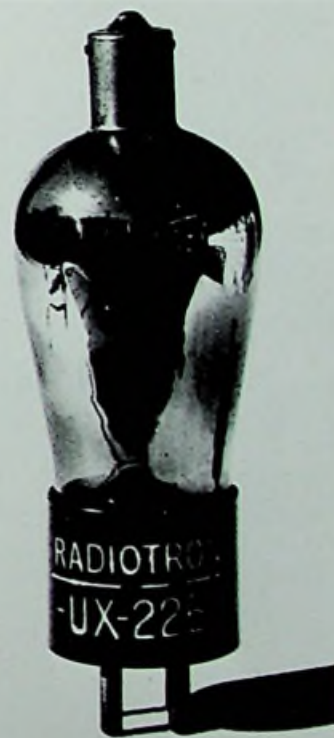
Experimental AC tube, prototype of UR-227. Note heater connections at top of bulb.
