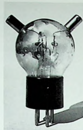
French Metal low-capacitance 'horned' tube c. 1925.
