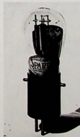
Sparton C401. Heater connections are to the side pins.
