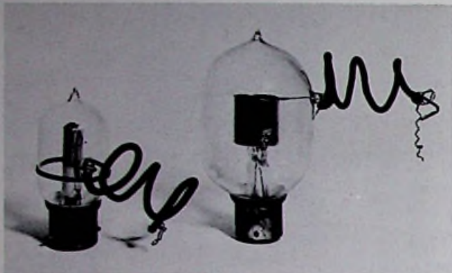
Photo courtesy Museum of Applied Arts & Sciences, N.S.W. Two commercial versions of Fleming's 'Oscillation Valve' by 'Royal Ediswan.' The smaller has a 4-volt filament, the larger has a 12-volt filament c. 1905-06.
