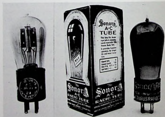
Arcturus AC28 and Sonora RA-1. These tubes had 15-volt carbon-heaters.
