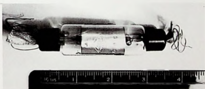
Expanse 'B' two-filament valve. Serial numbers were die-stamped on anodes.
