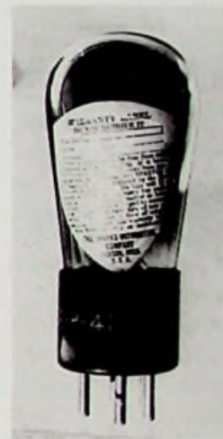
Sparton 686, battery triode. The fifth pin is unused.
