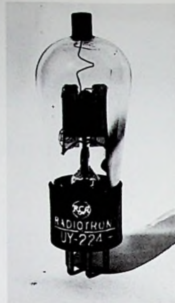
Early production model UY-224. Note fork-shaped screen assembly.
