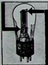
Showing the exclusive patented Eveready Raytheon 4-Pillar construction. Note the sturdy four-membered glass stem through which the four heavy wire supports pass, and the rigid mica sheet at the top.
