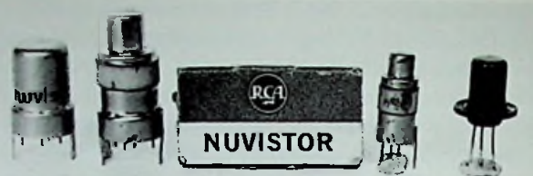
A group of three RCA Nuvistors compared with an early transistor (R.).
