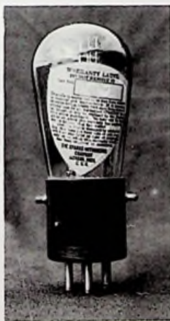
Sparton C181. Heater connections are to the side pins.
