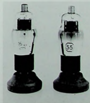
Radiotron 85 (6.3V) and 55 (2.5V).
