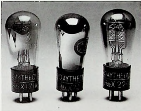
Raytheon Ray-X171A, 201A, 226. The centre tube was not of 4-pillar construction.
