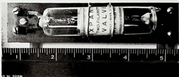
Expanse 'two-filament' valve. Note similarity to American 'Audiotron.'
