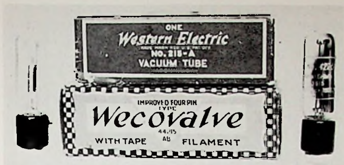
Standard telephones and cables. Wecovalve (R.) compared with a Western Electric 215-A (L.).
