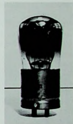
Example of a European tube using an American-style UV base c. 1924.
