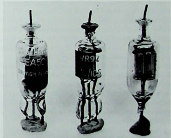
Mullard EA50. A detector diode originally released by Philips in 1939.
