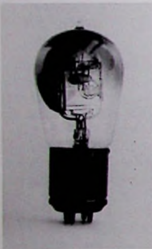
Rectron UV-196 single-anode full-wave rectifier (1925).
