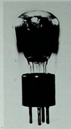
Example of tube using a Franco-British 4-pin bakelite base c. 1926.
