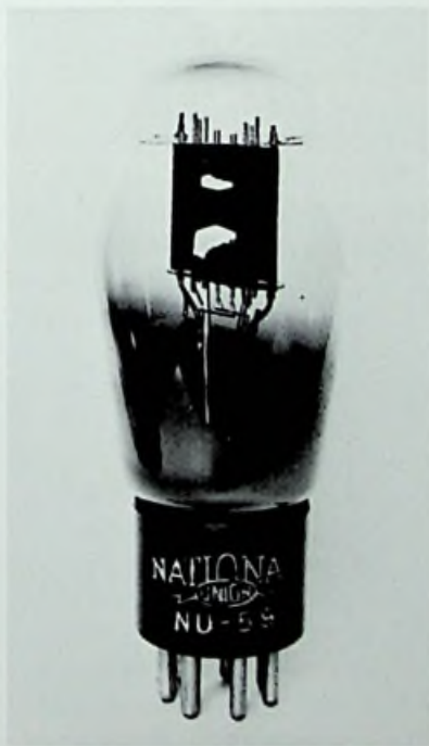
Example of tube using American large 7-pin base c. 1932.
