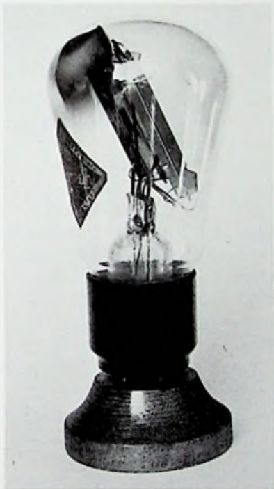
Standard-Micromesh R2, an early indirectly-heated rectifier.
