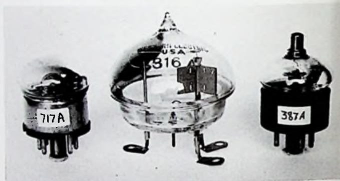
Western Electric 'doorknob' tubes designed for VHF and UHF use.
