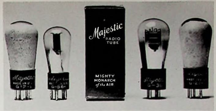
Typical Majestic tubes. Note the use of a large-size (S-14) bulb on the type G-30.
