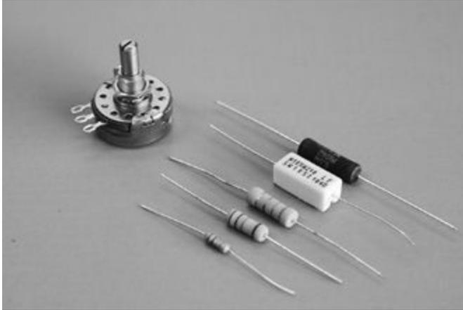
**FIGURE 2.1 A selection of various common resistors**
