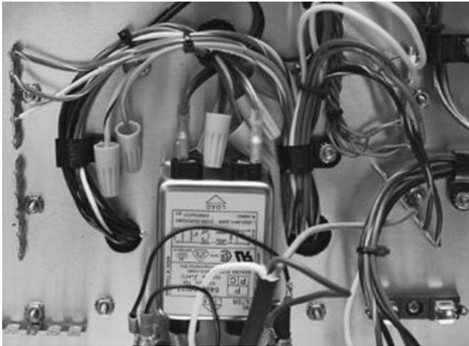
**FIGURE 8.4 Termination of unused transformer leads**
