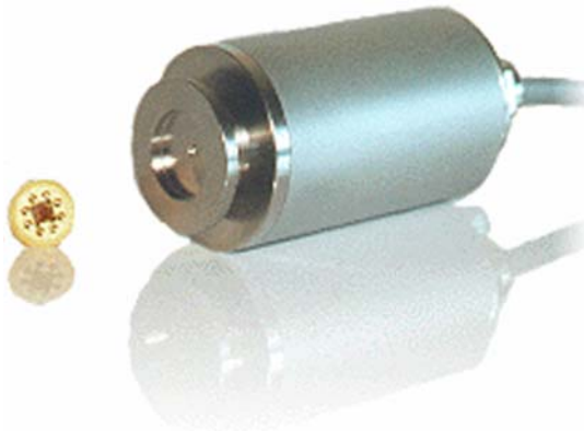
Fig. 11.18. Comparison of MicroPirani ( left ) and conventional Pirani gauges
