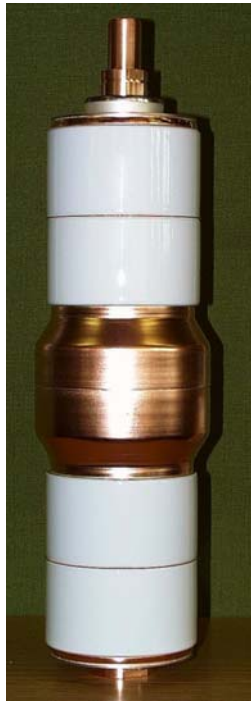
Fig. 9.11. High voltage vacuum interrupter (prototype): for 72.5 kV and 31.5 kA; 150 mm tube diameter; 500 mm length
