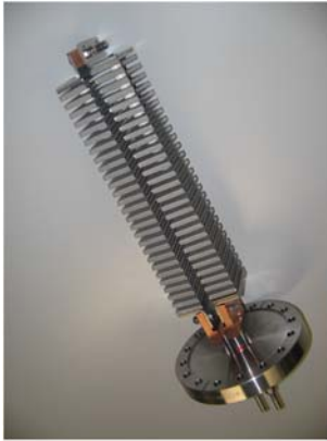
Fig. 11.10. Getter pump with two NEG strips ( left ) and diagram of activation of St 707™ ( right )
