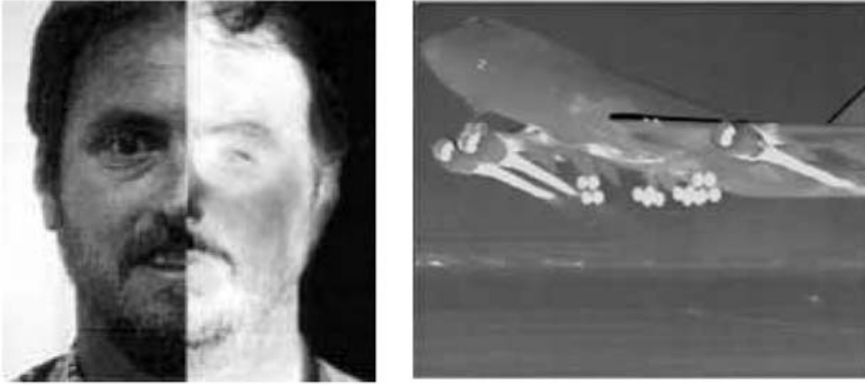
Fig. 7.8. Left: black and white image of a man's head in visible light, left , and the IR image, right . Right: airplane after takeoff with clearly shown jets and also hot tires of the wheels
