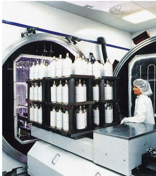
Fig. 9.1. One-shot-brazing technique (Siemens). In a batch of several tens or hundreds the bottles will be evacuated and brazed at 800–900°C in an ultrahigh-vacuum furnace in one process (one-shot)
