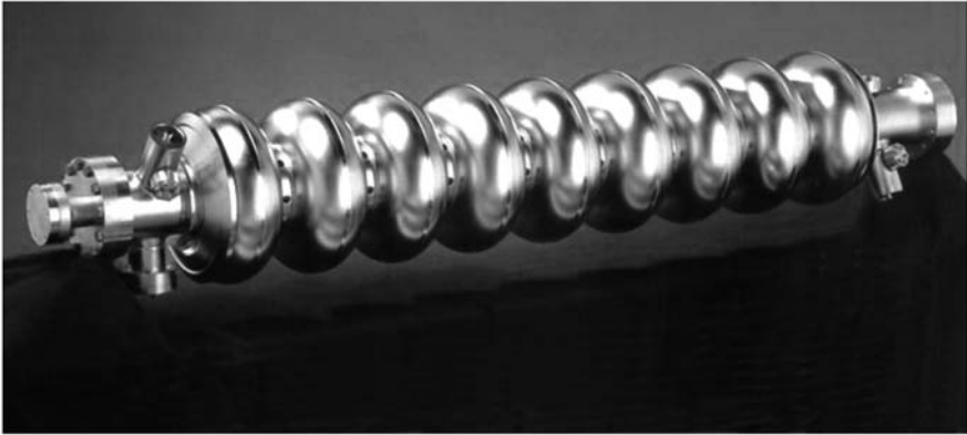
Fig. 8.6. Superconducting TESLA shaped 9-cell cavity for operation at 1.3 GHz
