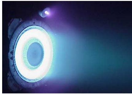
Fig. 6.10. Photograph of the exhaust plume of a PPS® 1350 HET, taken from [50]
