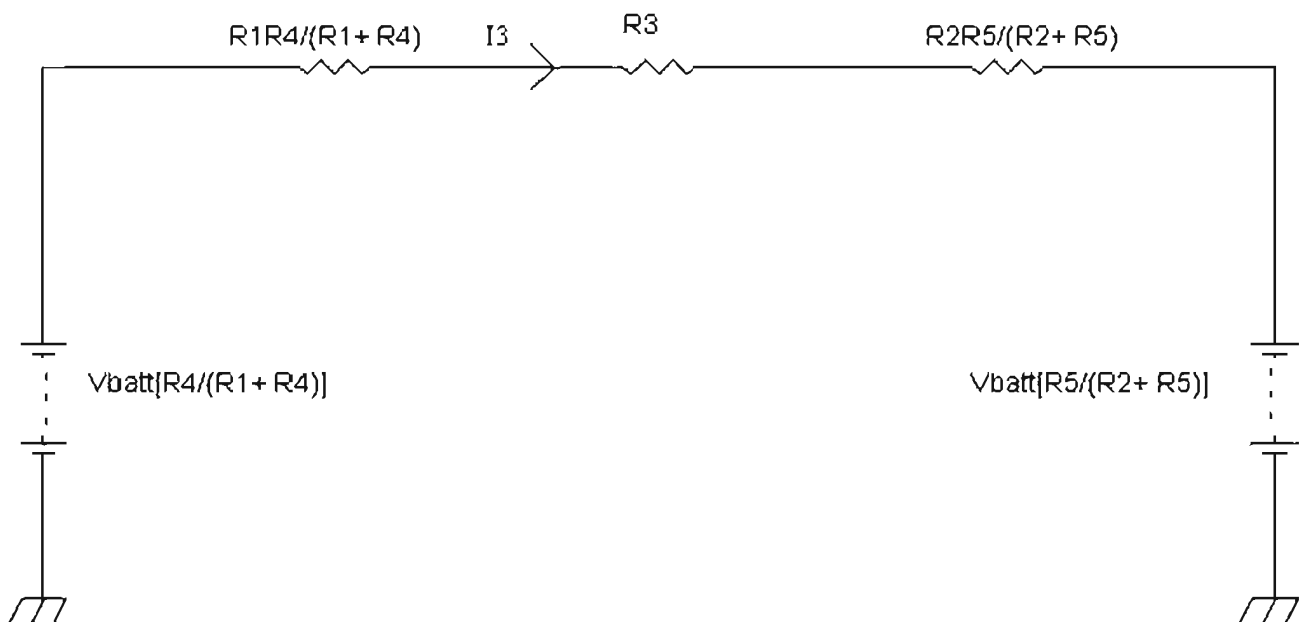
FIGURE 23-33 The circuit in Figure 23-32 is redrawn as two Thevenin-equivalent circuits.
