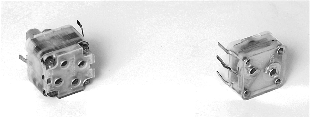
FIGURE 3-3 Variable capacitors using poly material for insulation between plates.
