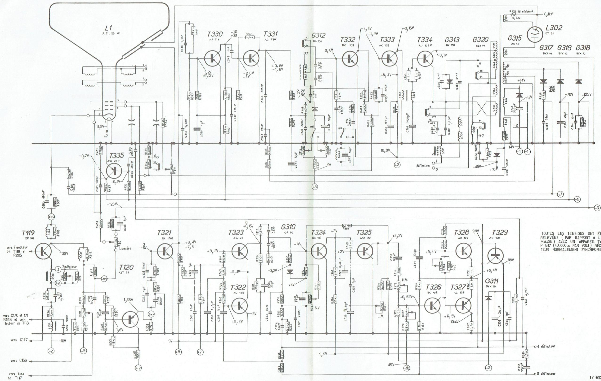
TOUTES LES TENSIONS ONT ÉTÉ RELEVÉES ( PAR RAPPORT A LA MASSE ) AVEC UN APPAREIL TYPE P 817 ( 40.000 Ω PAR VOLT ) RECEPTEUR NORMALEMENT SYNCHRONISÉ.
