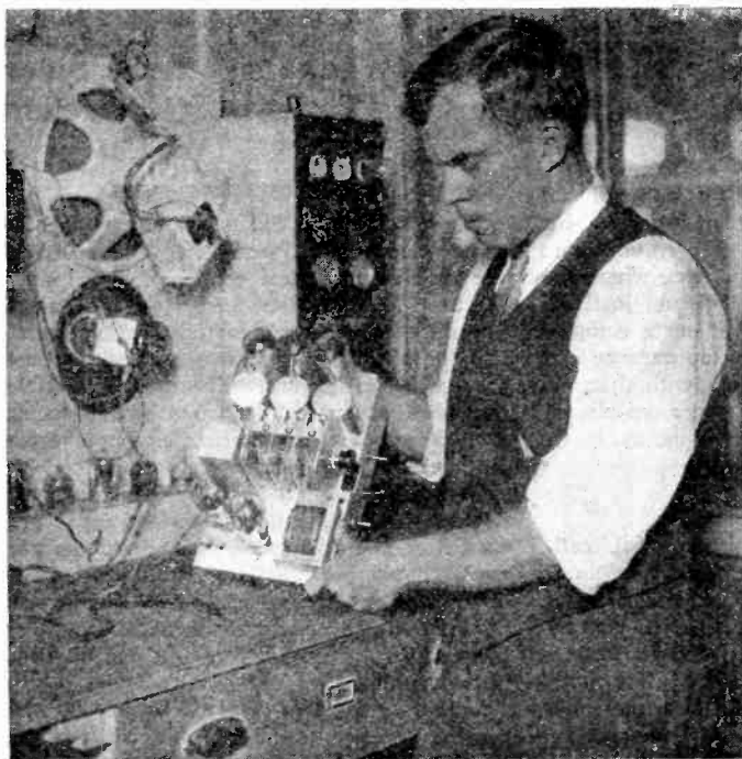
Mr. A. M. Morgan, of the Pilot engineering staff, showing the chassis construction of the TRF Midget. The RF transformers for the 200-550 meter range are in the shield cans next to the three-gang tuning condenser.
