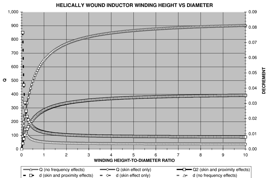
FIGURE 4-7 Optimum H -to- D ratio for close wound magnet wire, case 3.
