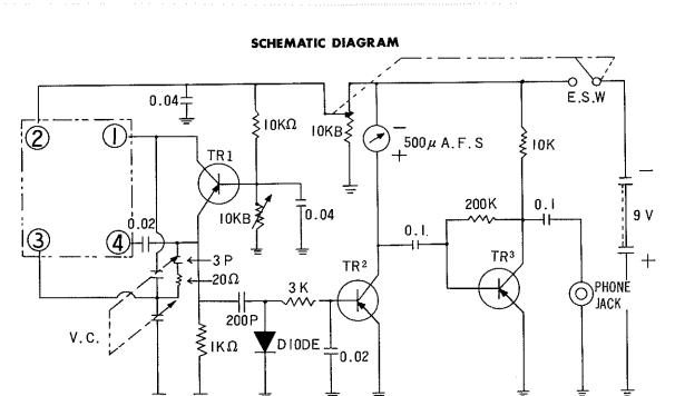
TRIPNP MESA TYPE GERMANIUM TRANSISTOR TR2, TR3, PNPTYPE ALLOY-JUNCTION GER. TRANSISTORS. 28854DIODE POINT CONTACT GER. DIODE. V. C. MITUMI PVC-25. BATTERY BL-006P.
