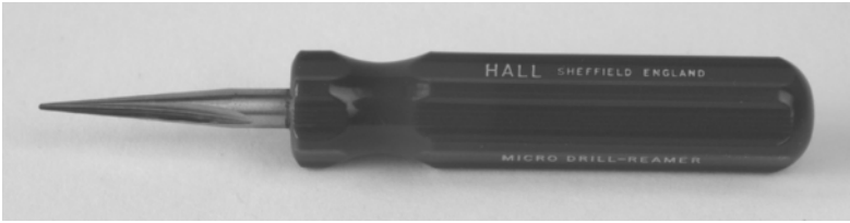
Figure 3.55 Tapered reamer for enlarging small holes
