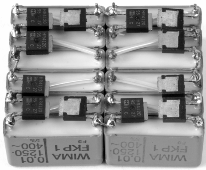
Figure 3.52 Once laid out, the rectifier can be constructed quickly and neatly, then potted
