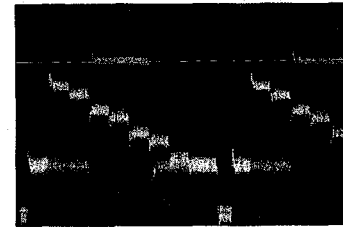
㉖ Pin 26 of IC301 (0.5Vp-p)
