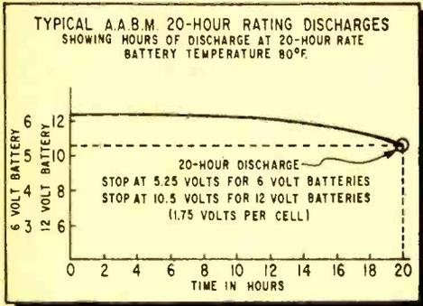
Fig. 6. Association of Automobile Battery Manufacturers established the 20-hour yardstick.
