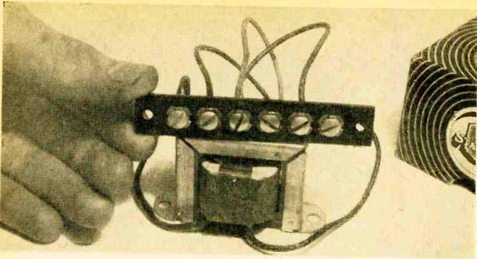
Handy for experimental hookups: Attach a terminal strip to a small transformer, soldering one lug to transformer housing; solder leads to the strip as shown. This prevents lead breakage due to twisting of the leads while they are being soldered and unsoldered from hookups.
