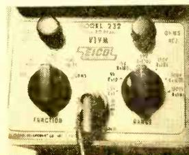
Left: VTVM is used on home project. Unit shown is an EICO 232 assembled from a kit. Top right: balance controls can be reached without removing case. Bottom right: controls are Zero and Ohms Adj.; Function, Range.
