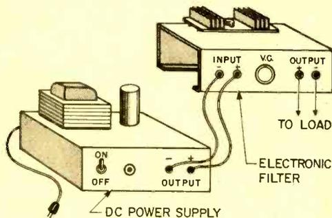
Fig. 3. Filter is placed between power supply and load which, on the cover, is a tuner.
