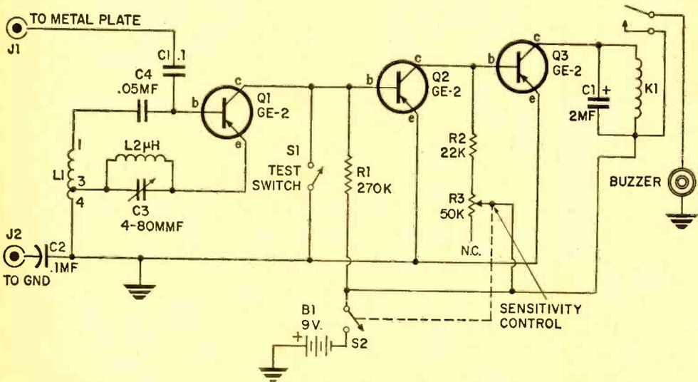
Capacitance between an intruder and the metal plate or strap is coupled to oscillator transistor Q1 through jack J1 to trigger the circuit.
