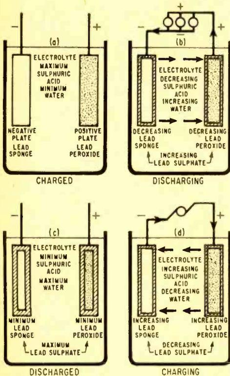
Fig. 1. These graphic illustrations trace the cycle of chemical reactions in storage batteries. Sulphuric acid,  $H_2SO_4$ , breaks down to water  $H_2O$ , during discharge; lead forms  $PbSO_4$ .
