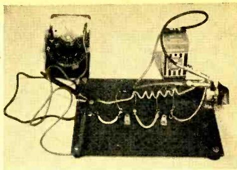
Fig. 6. Ammeter hooked to Fahnestock clips.
