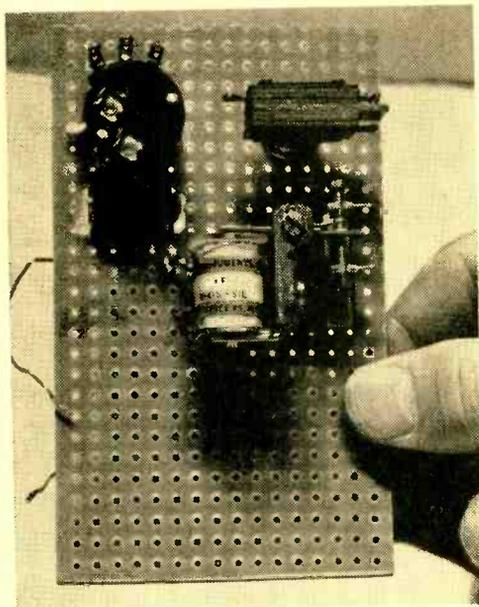
Construction is started by mounting the larger components on the perforated board.
