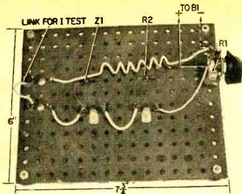
Fig. 5. Components are mounted on Masonite.
