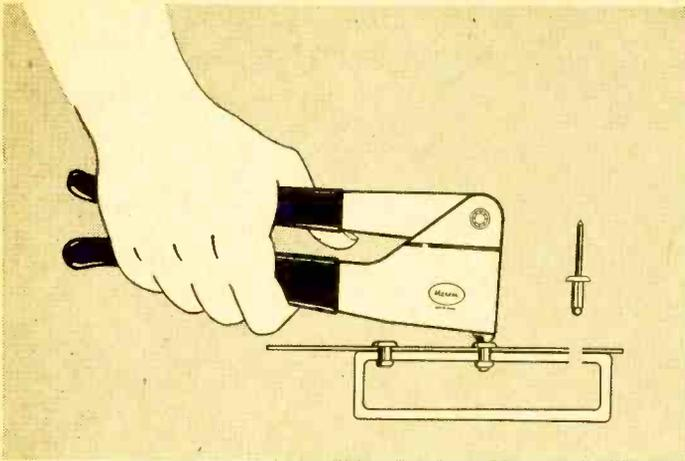
If you really turn out your projects in mass production, you'll save a lot of time by not fooling around with nuts and bolts with this riveting tool. It's quick, easy, and makes a lasting joint.
