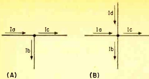
Fig. 1. Three-wire (A) or the four-wire junction (B) illustrates Kirchhoff's current law.
