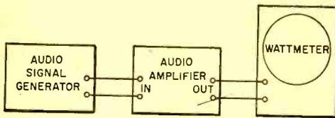
Fig. 1. Setup to measure db gain of an amplifier—wattmeter has 16-ohm resistor.
