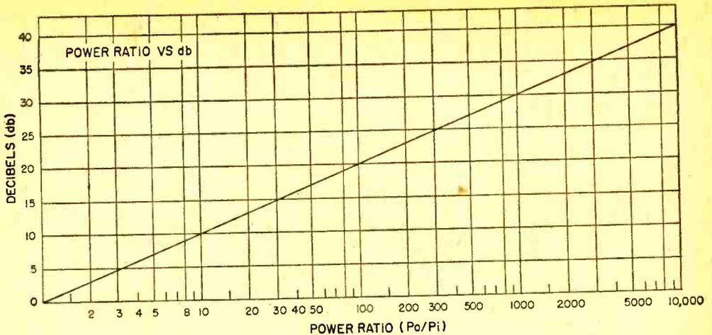
Fig. 2. Graph of power ratio versus decibels eliminates computations.
