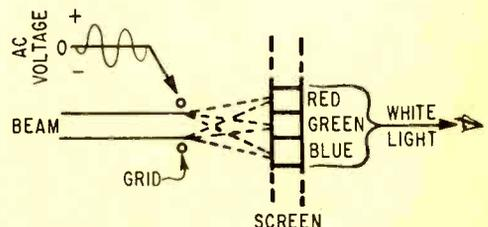
Fig. 6. An alternating voltage on grid wires shifts the beam among screen stripes.
