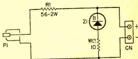
Fig. 13. 12- to 9-volt Zener diode converter for powering transistor radio from automobile.
