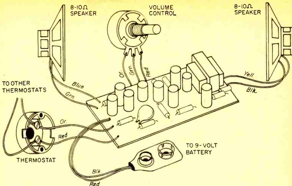
Thermostat is connected as on-off switch, and control is adjusted for desired alarm signal.
