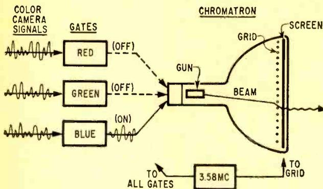
Fig. 7. Action necessary for producing blue image on phosphor screen—the 3.58-mc signal simultaneously positions beam on blue screen stripe and opens blue gate. Blue signal (originally from TV camera) may now control gun's beam strength at this short instant.
