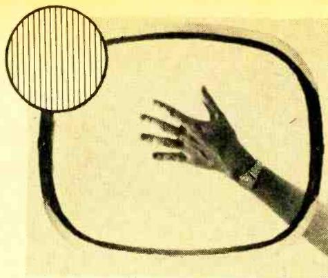
Fig. 1. Conventional color tubes use a dot-pattern shadow mask (left) that consists of many fine holes; Chromatron uses fine, evenly spaced grid wires (right). Note difference in transparency of the masks which increases brightness.
