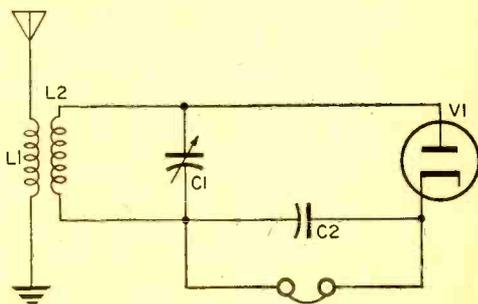
Fig. 7. In this AM detector circuit, capacitor  $C_2$  functions as an RF bypass for the headset.
