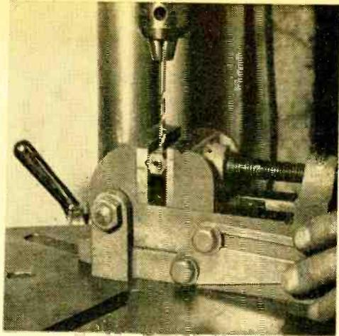
Each of three pole end pieces is drilled with a countersunk hole and tapped to take 10-32 flathead machine screws filed flush.
