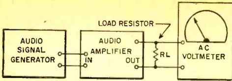
Fig. 5. An AC voltmeter and a calibrated load resistor can be used to measure db's.
