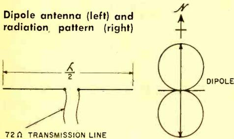
wavelength. Something known as "end effect" electrically shortens the antenna, so it must be shortened physically to be electrically correct. For this reason, a dipole's length is calculated from the modified formula.
