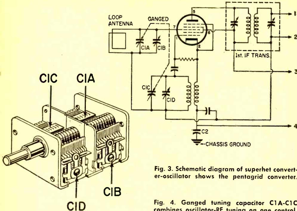
Fig. 3. Schematic diagram of superhet converter-oscillator shows the pentagrid converter.
