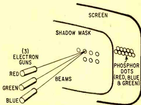
Fig. 8. Conventional color tube uses three guns, shadow mask, and phosphor-dot screen.
