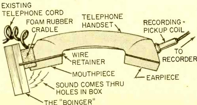
The Boinger attaches directly to the mouthpiece of your telephone, and puts out an audible "boing" every 15 seconds. It is used when recording a telephone conversation to remind both parties that the conversation is being recorded. This is a Federal law on interstate calls and is also a law on local telephone calls in a large number of our 50 states.
