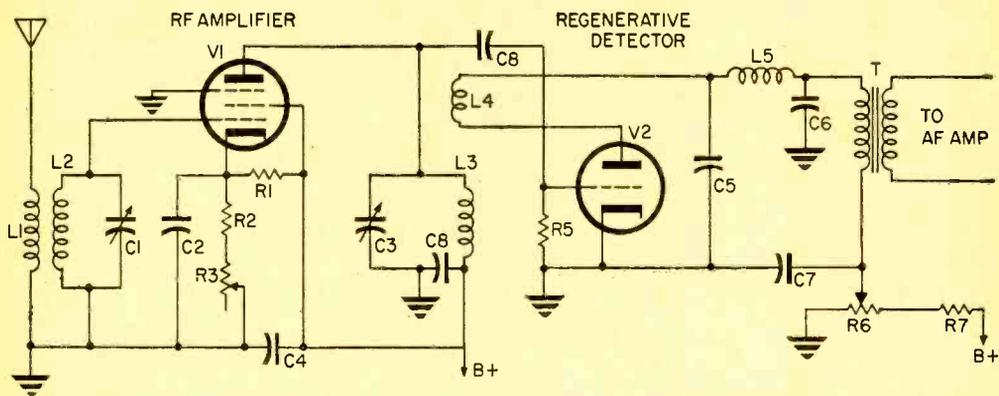
Fig. 20. Receiver circuit with tuned RF stage and regenerative detector is very sensitive and quite selective for VLF to VHF.
