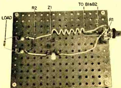
Fig. 10. Series voltage regulator breadboard.
