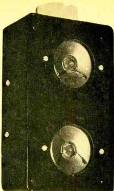
Alarm's shrill signal is started and maintained by feedback from the output to input speaker.
