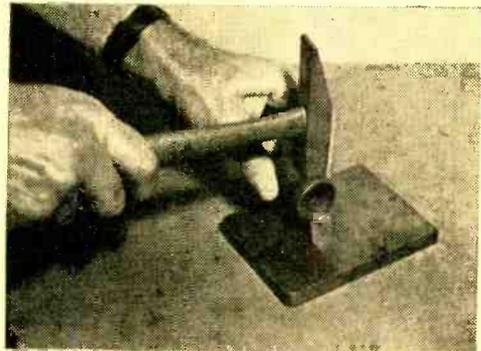
Slight curvature is given to the pole end pieces by striking a pipe coupling on a V-block with end piece in between as shown.
