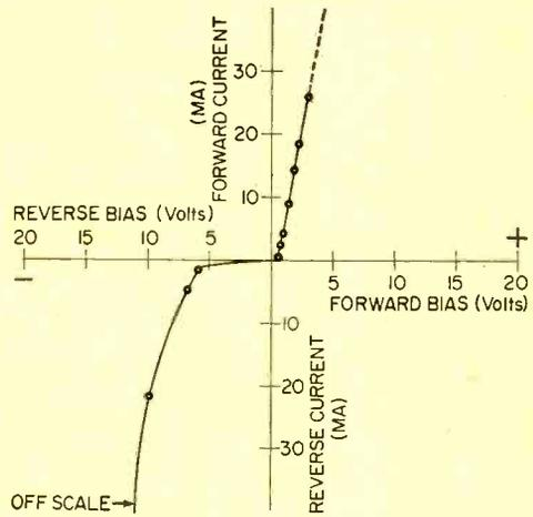
**Fig. 8. Forward and reverse characteristics.**
