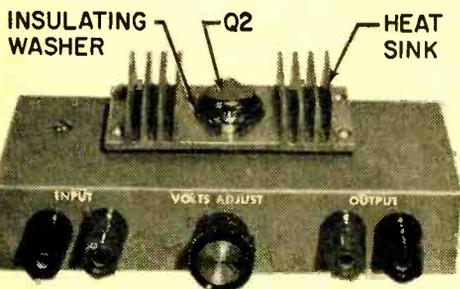
Top mount and heat sink dissipate Q2's heat.
