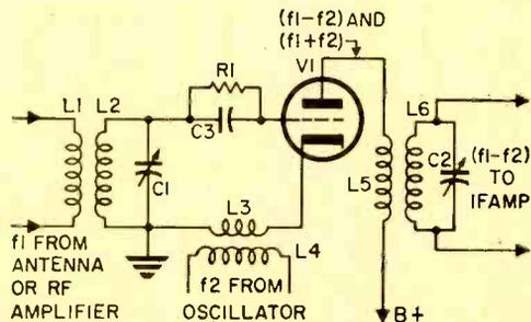
Fig. 3. In this circuit, triode V1 is the converter where frequencies  $f_1$  and  $f_2$  are mixed.
