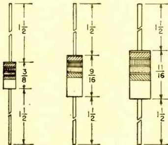
TYPE RC-20 (1/2 WATT)      TYPE RC-32 (1 WATT)      TYPE RC-42 (2 WATT)
