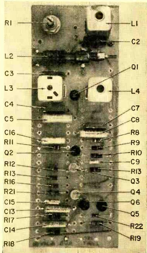
Top view of circuit board that holds almost all the components for an SCA-FM adapter project; rat's nest wiring is eliminated.
