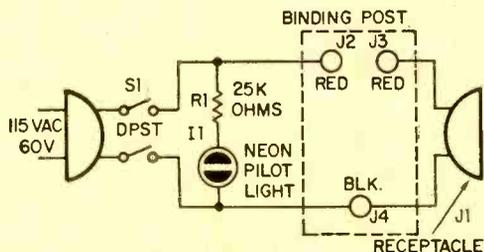
The neon pilot light connected across the line voltage reminds you the tap is "hot."
