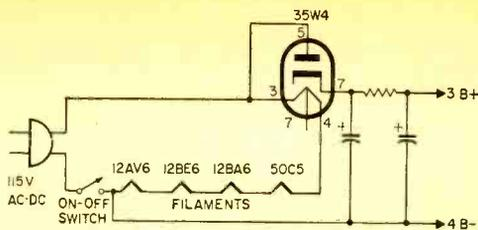
Fig. 7. The power supply that provides the DC voltages for receiver utilizes 35W4 diode tube in filtered half-wave rectifier circuit.
