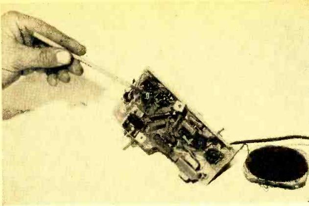
Make sure you have identified all components before aligning receiver. On some receivers, the oscillator coil looks just like the IF cans.
