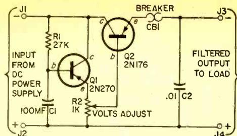
Fig. 2. Schematic diagram of actual filter shows improvements over the basic principle.
