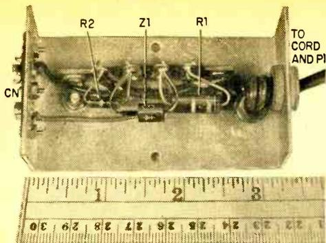
Fig. 14. Underside of auto adapter chassis.
