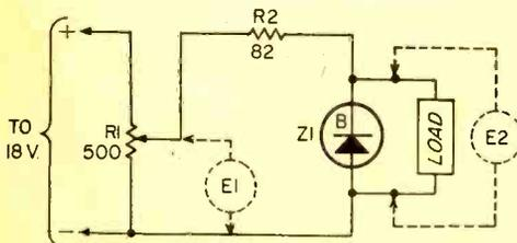
**Fig. 11. Schematic of shunt regulator circuit.**
