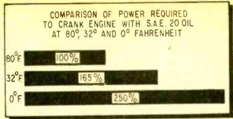
Fig. 9. During winter engines are harder to crank and less battery energy is available.
