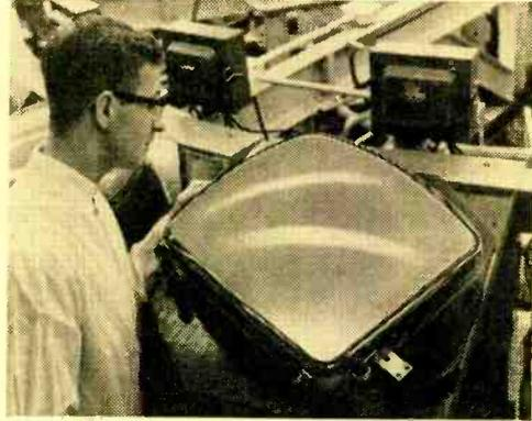
Zenith engineers new 25-inch three-gun color picture tube with 90-degree deflection.
