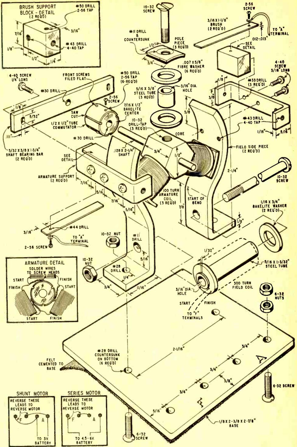
The exact construction details for the author's unit are shown in the above detail drawing. Minor variations can be made to suit available materials.
