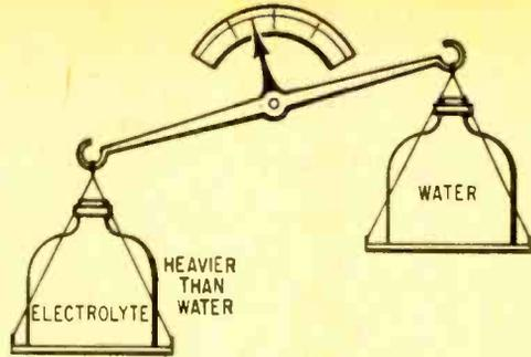
Fig. 2. Specific gravity of sulphuric acid-water electrolyte is greater than that of pure water.
