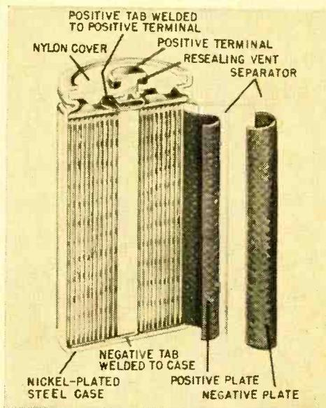
Cutaway of General Electric's nickel-cadmium battery with new safety vent. The vent assures a continuous safe power source for cordless appliances by acting as a guard against inadvertent cell and battery abuse.
