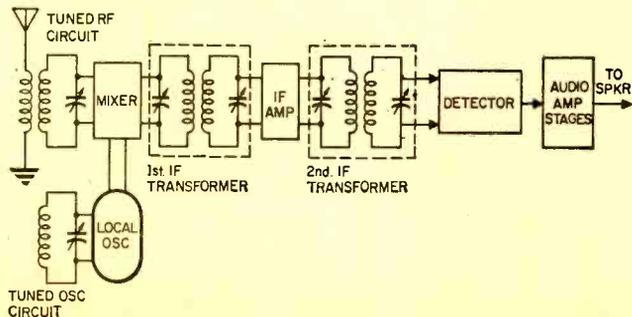
Fig. 2. In the superheterodyne receiver, the incoming RF signal is reduced to an intermediate frequency in the mixer.
