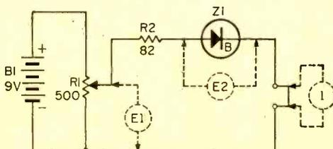
Fig. 4. Diagram for forward characteristics.
