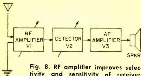
Fig. 8. RF amplifier improves selectivity and sensitivity of receiver.
