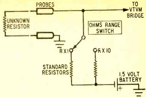
Fig. 7. Simplified input circuit to VTVM bridge circuit for measuring resistance values.
