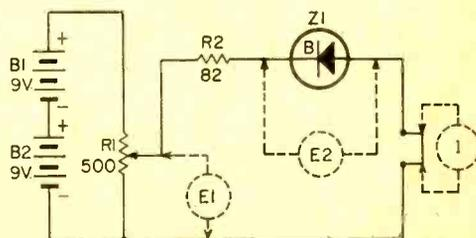
Fig. 7. Diagram for the reverse characteristics.
