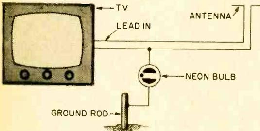
Lightning can ruin a TV set, even one with a lightning arrester. For added protection connect a glow lamp (NE-7) between the set's antenna terminals and ground rod as shown. Voltages over 55 volts will then pass through the bulb to ground, thus bypassing the set.
