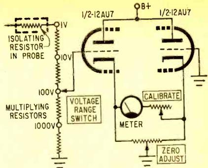
Fig. 4. Basic VTVM circuit showing the zero adjust and calibrate potentiometers.
