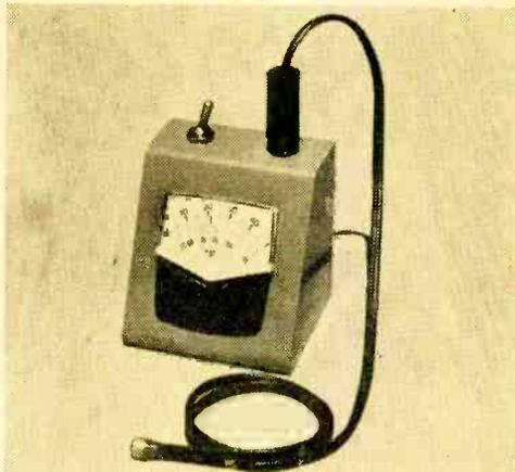
Meter cases are home-brew favorites; this one holds meter scaled for temperature readings. The sensor, plugged into the circuit housed in the meter case, is immersed in photographic fixing baths to monitor their temperature.
