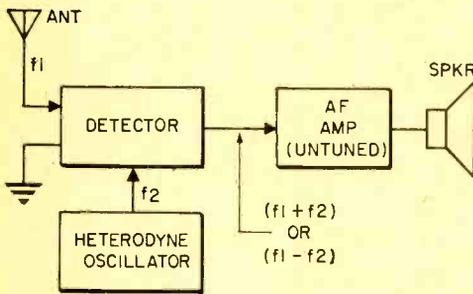
Fig. 1. In the heterodyne receiver, detected signal is passed directly to audio amplifier.
