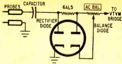
Fig. 6. Typical rectifier circuit used in VTVM's to convert AC to DC for measuring.
