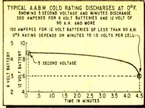
Fig. 7. Another important criterion for rating a battery is its auto engine cranking ability.
