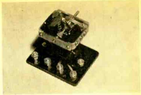
Close-up view of motor reveals simplicity of construction. Of an extremely compact design, the motor stands only 2 3/8 in. high.
