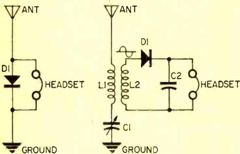
Fig. 1. (left) Selectivity of basic TRF is low.
