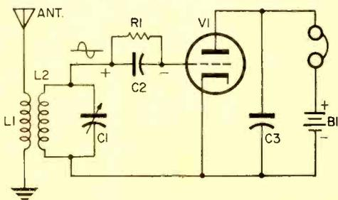
Fig. 4. Triode tube replaced the crystal diode combining detection and audio amplification.
