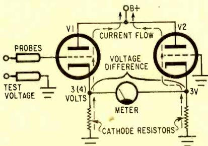
Fig. 3. Simplified balanced bridge circuit that is usually used in modern VTVM devices.
