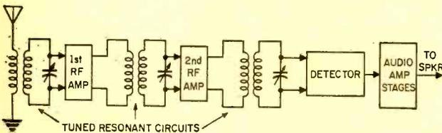
Fig. 1. Each stage of the TRF receiver is tuned individually to ensure the selectivity of the receiver. After RF stages, signal is detected and amplified.
