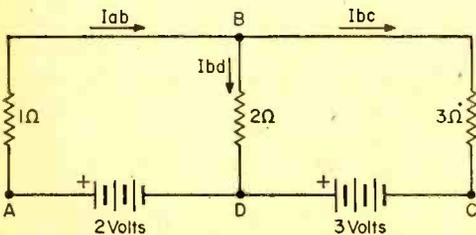
Fig. 2. Kirchhoff's voltage law analyzes closed path circuits; two here are DABD and DBCD.
