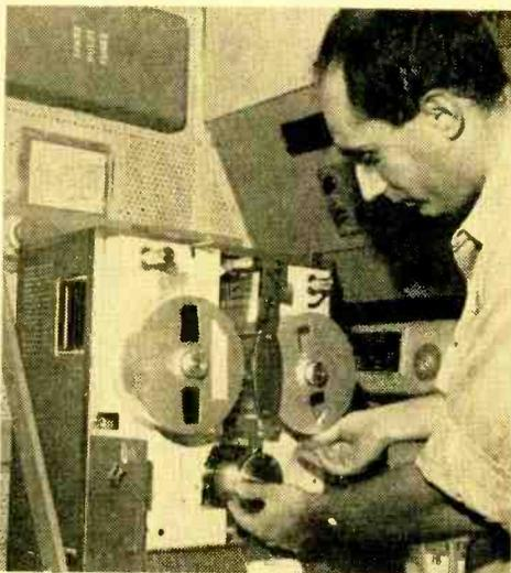
Motion pictures are transmitted from the Sony video tape machine located in cockpit of American's 707 and 720 Astrojets. Astrovision, a four-part in-flight entertainment system, also features stereophonic classical and popular music, live and tape TV, and in-flight photos.
