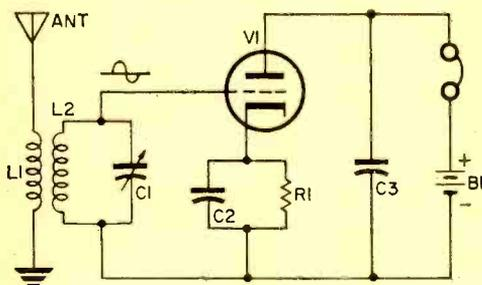
Fig. 5. Detection of audio signal from RF carrier in this triode is termed plate detection.
