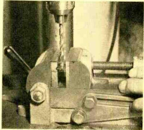
Drill, tap and countersink holes in three alternate sides of the armature to accept flush-fitting 10-32 flathead machine screws.
