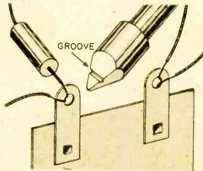
File a groove in one side of your soldering iron for "pouring" solder on connections of a crowded chassis.
