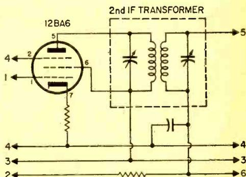
Fig. 5. IF amplifier tube 12BA6 boosts signal; second IF transformer increases selectivity.
