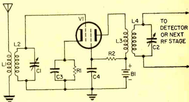
cathode resistors which are bypassed by capacitors for RF. Their tuned circuits are equipped with RF bypass capacitors ( $C_2$  and  $C_4$ ) which are large enough to not affect the tuning by  $C_1$  and  $C_3$  and, at the same time, to increase the AVC time constant so as to prevent too fast a change in AVC voltage.
