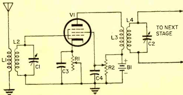
Fig. 12. Addition of a third grid results in pentode which has improved gain over lesser element tubes, and easier control of gain. Choice of control gives remote or sharp cutoff.
