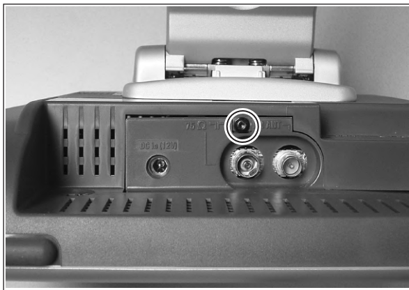
Figure 4-4 Rear cover removal hidden screw EU version
