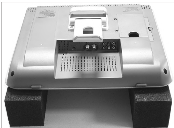
Figure 4-1 Service position with ESD protective service buffers
