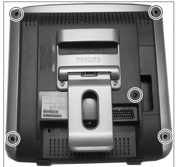
Figure 4-2 Rear cover removal 13- and 15-inch
