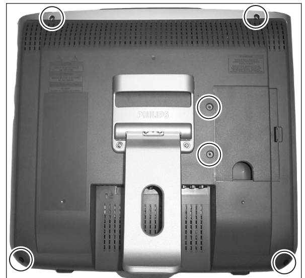
Figure 4-3 Rear cover removal 20-inch
