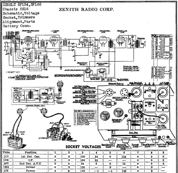
All voltages measured with a 1900 ohm per volt D.C. meter and using the Zenith 6 V Economy Pack—Antenna and ground disconnected.
