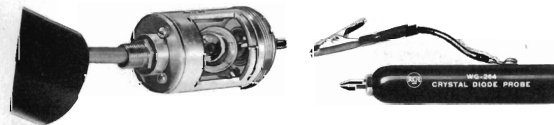
Fig. 9-14. Diode probes: (A) vacuum type; (B) crystal type.
