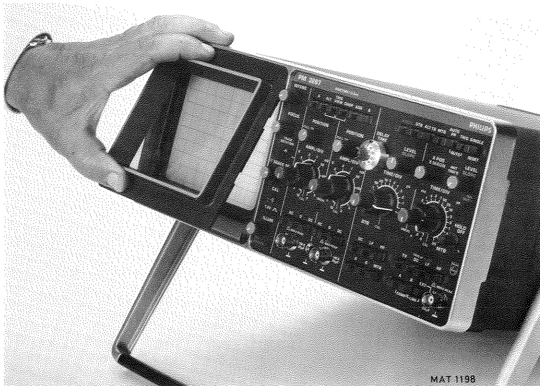
Fig. 5.1. Removing the bezel and contrast plate
