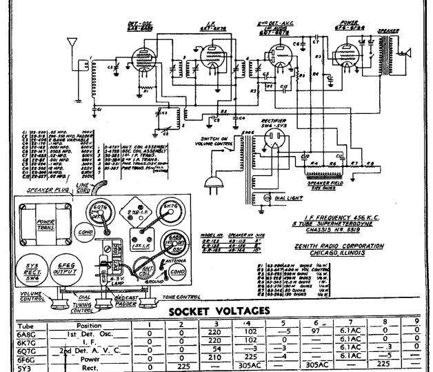
Line voltage 115 V. Antenna and ground disconnected. All voltages measured from point indicated to ground, using a 1000 ohm per volt meter.
