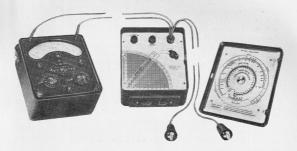
The illustration shows a Power Factor and Wattage Unit connected up to a Model 40 Mk. II Avometer ready for use.
