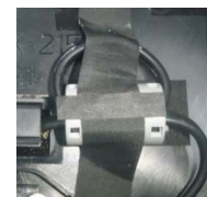
New must stick on the EMI core top side Part Name: HIMELON (FANF) Part Number: 4-466-473-61
