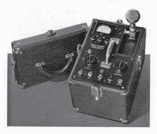
This instrument was designed to meet the demand for an inexpensive sound level meter complying with the tentative standards of the American Standards Association, the American Institute of Electrical Engineers, and the Acoustical Society of America. It incorporates several features previously found only in more expensive and cumbersome instruments and is suitable for practically all types of commercial sound level measurements. Among the features of the new noise meter are the following:
