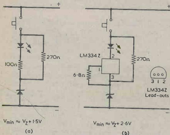
Fig. 4(a). If the l.e.d. in this circuit fails to light when the push-button is pressed the supply voltage is below the  $V_{min}$  level.
