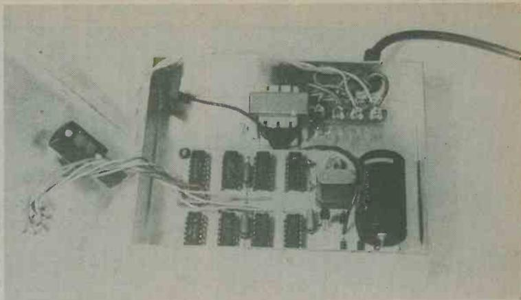
upon positive feedback and oscillation occurs at this frequency. In the present design this is 10MHz. The trimmer enables the oscillation frequency to be set to precisely the nominal figure for the crystal. A third NAND gate, also connected as an inverter, couples to the oscillator output and squares up the oscillator sine wave so that the following stages can operate cleanly. No connections are made to the fourth NAND gate of the i.c.
