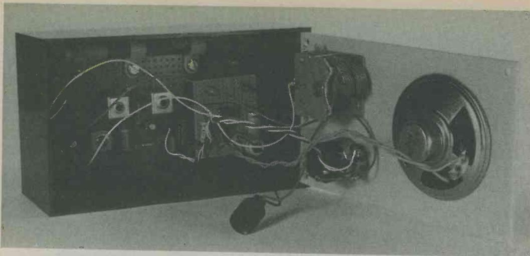
The tuning capacitor, volume control/on-off switch and speaker are mounted on the front panel. The main component board is bolted to the rear panel of the case.
