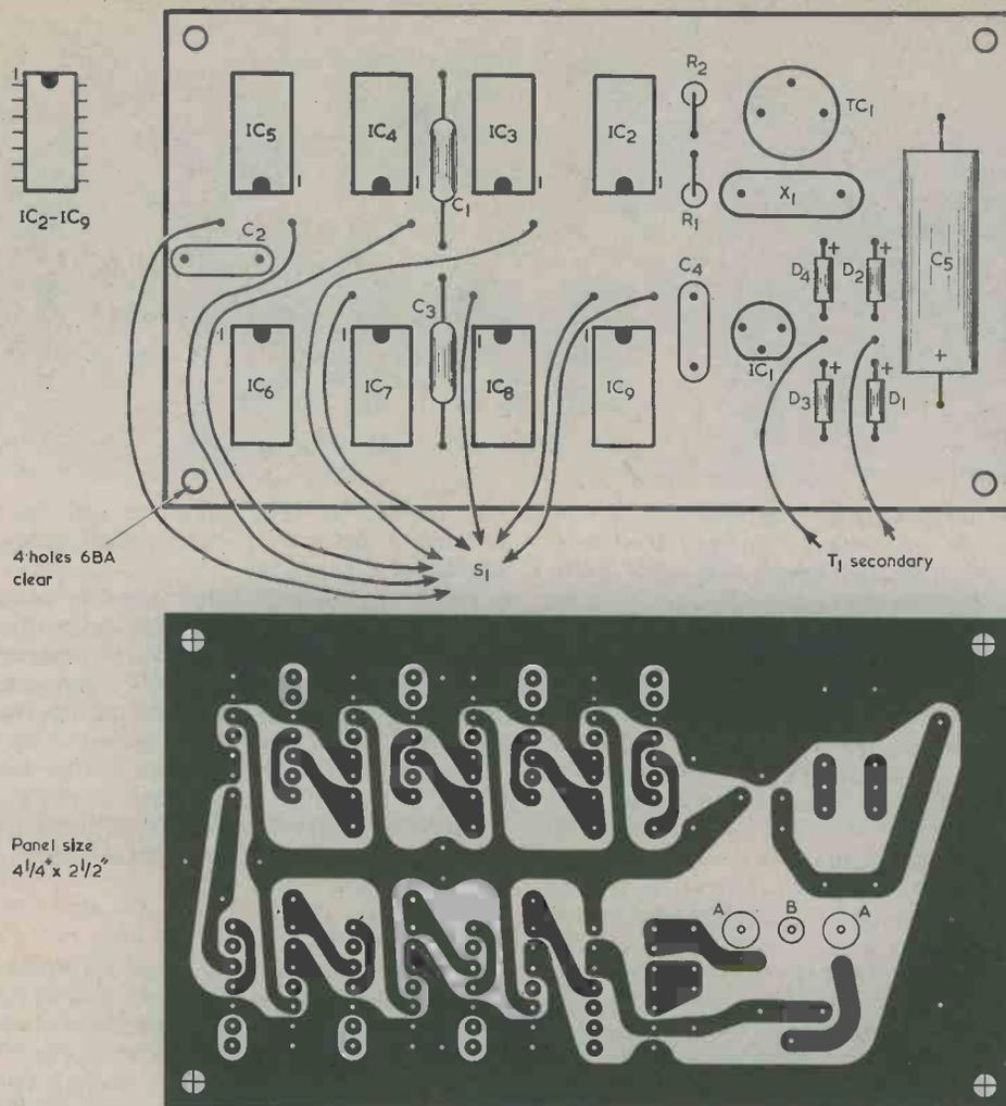
Fig. 2. The component and copper sides of the printed circuit board. This is reproduced full size.
