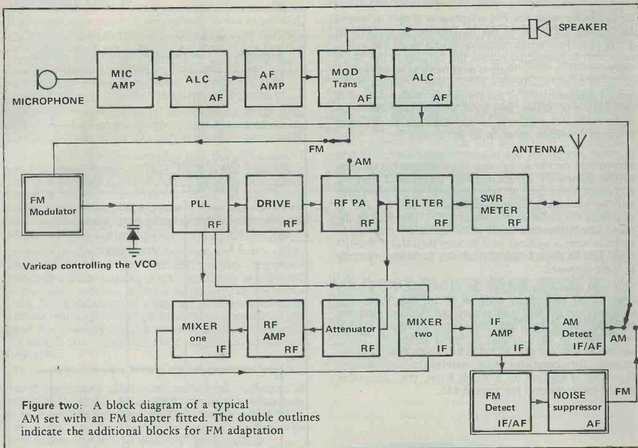
Figure two: A block diagram of a typical AM set with an FM adapter fitted. The double outlines indicate the additional blocks for FM adaptation
