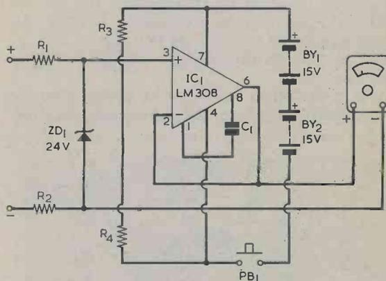
Fig. 2. The circuit of the voltmeter sensitivity booster. This employs an LM308 as a voltage follower, with protection against excessive input voltages being provided by ZD1. The multimeter should, preferably, have a sensitivity of 10,000 $\Omega$  per volt, or better.
