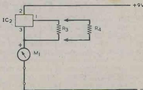
Fig. 3. The meter is initially assembled without R4. Various values are then checked experimentally until the required value is found.
