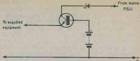
**Fig. 3.** Another solid-state circuit which gives automatic changeover.
