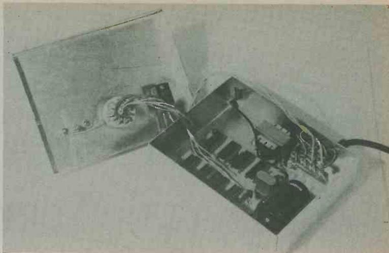
provides an output which is at t.t.l. levels. The waveshape is good when observed on an oscilloscope, although the higher ranges are slightly modulated by the lower two ranges. This is unavoidable and is due to the lack of isolation between outputs. No difficulties were experienced when using the calibrator with sensitive digital equipment.
