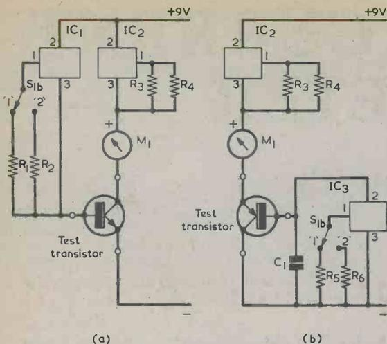
Fig. 2(a). The test circuit which is set up when an n.p.n. transistor is connected to the meter.
