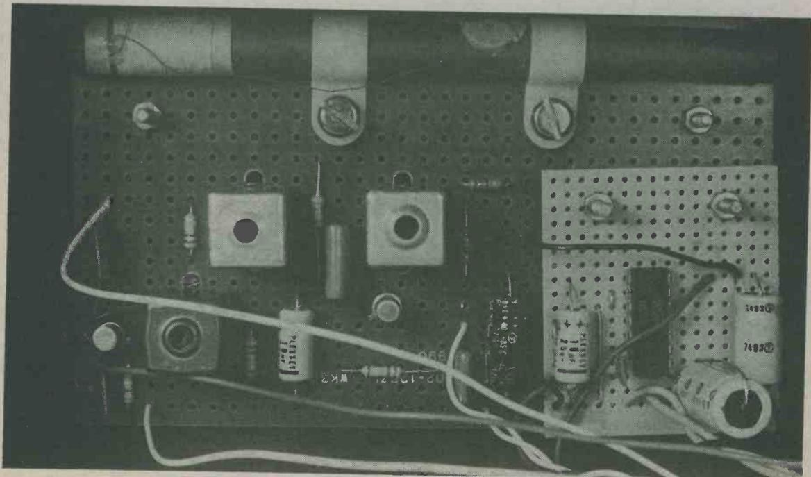
Looking down directly on the main component board and the smaller a.f. board. The ferrite aerial is secured to the main board.
