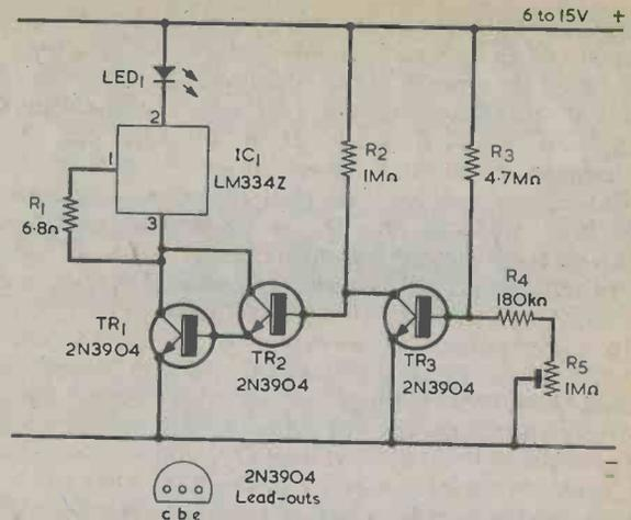
Fig. 5 This circuit is permanently connected across the supply rails and draws a very low quiescent current. The l.e.d. lights up for supply voltages lower than  $V_{min}$
