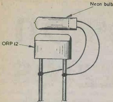
**Fig. 8.** A wire-ended neon bulb soldered to the leads of a photoconductive cell. (This arrangement was originally described by G. A. French in the May 1970 issue.)
