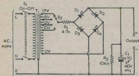
Fig. 1. A very simple variable voltage unregulated mains power supply. Could anything go wrong in such a basic circuit?
