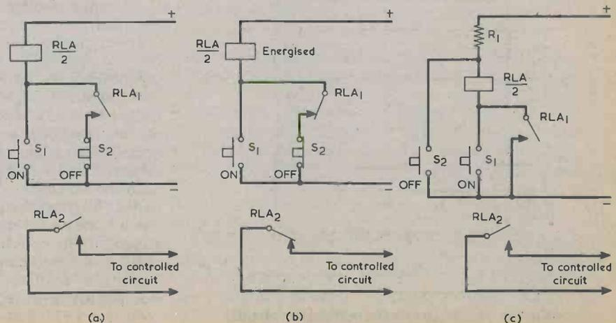
supplied via the resistor R1. When push-button S2 is pressed it short-circuits the relay coil, whereupon the relay releases again and stays released. The resistor will normally have a value of the same order as the relay coil resistance and it requires a wattage rating suitable for the period, with S2 pressed, when it has the whole supply voltage applied across it.
