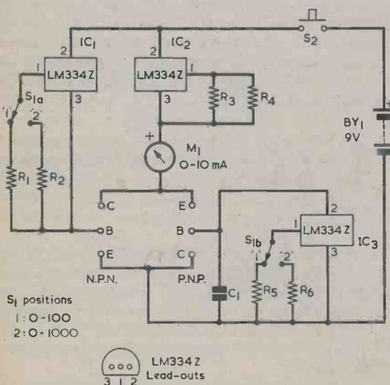
Fig. 1. The complete circuit of the transistor hFe meter. IC1 and IC3 are constant current devices which provide pre-selected base currents. IC3 limits the current in the meter circuit.
