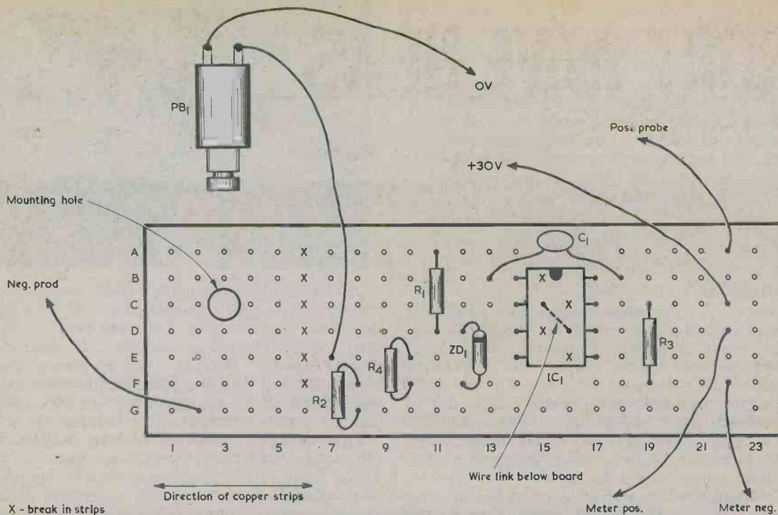
**Fig. 3. The booster Veroboard layout. The bush of PB1 passes through the mounting hole and secures the board to the lid of the plastic case in which the booster is housed.**
