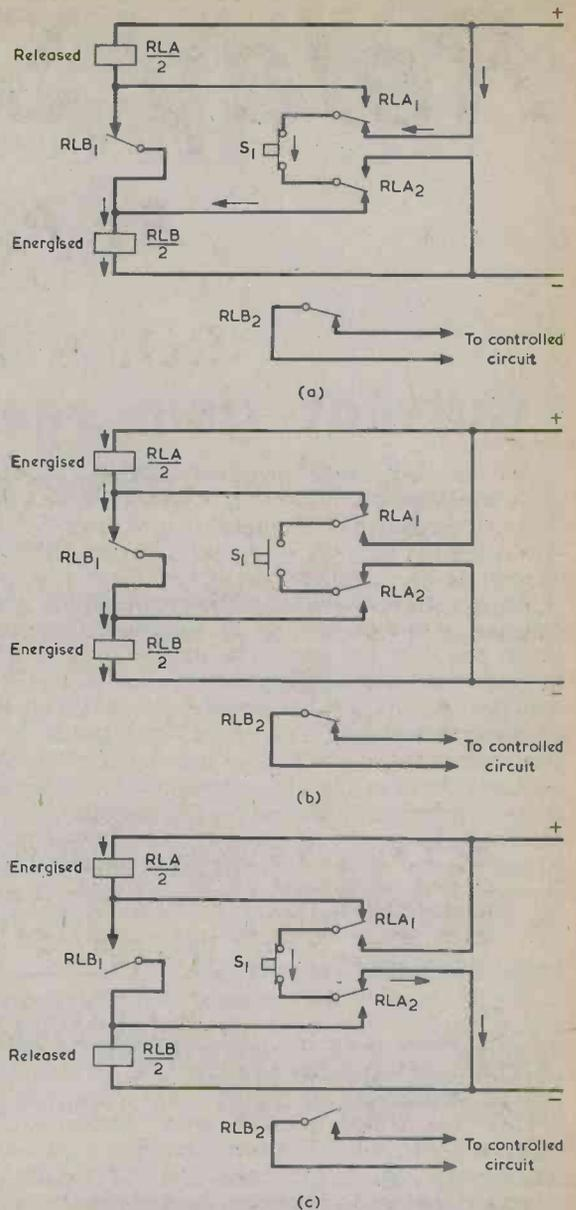
Fig. 4(a). When S1 of Fig. 3 is first pressed, relay RLB energises.
