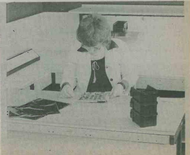
The technician here wears a wrist strap to provide positive body earthing. To further guard against high static voltages, the bench is covered with an earthed conductive top mat, and her feet rest on another earthed mat of the same material. All these items are produced by Modulux Industrial Equipment Ltd.
