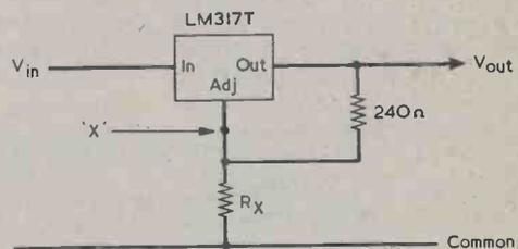
Fig. 2. If RX is short-circuited by the negative pulses of a square wave, another square wave appears at the regulator output.
