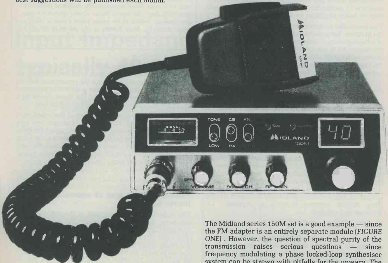
The Midland series 150M set is a good example — since the FM adapter is an entirely separate module (FIGURE ONE). However, the question of spectral purity of the transmission raises serious questions — since frequency modulating a phase locked-loop synthesiser system can be strewn with pitfalls for the unwary. The maximum deviation that can be expected from such an arrangement is likely to be only 1-2kHz. Purpose designed FM systems can naturally cope with any value required.
