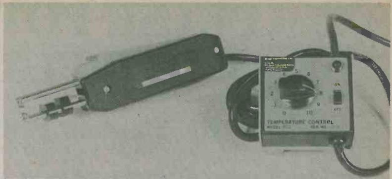
The Eraser International thermal wire stripper type TWC-1 and the TC-1 temperature control unit. Stripping temperatures up to 700 deg F are available for high temperature insulations. Lower temperatures, for PVC, nylon and similar insulations can also be selected.
