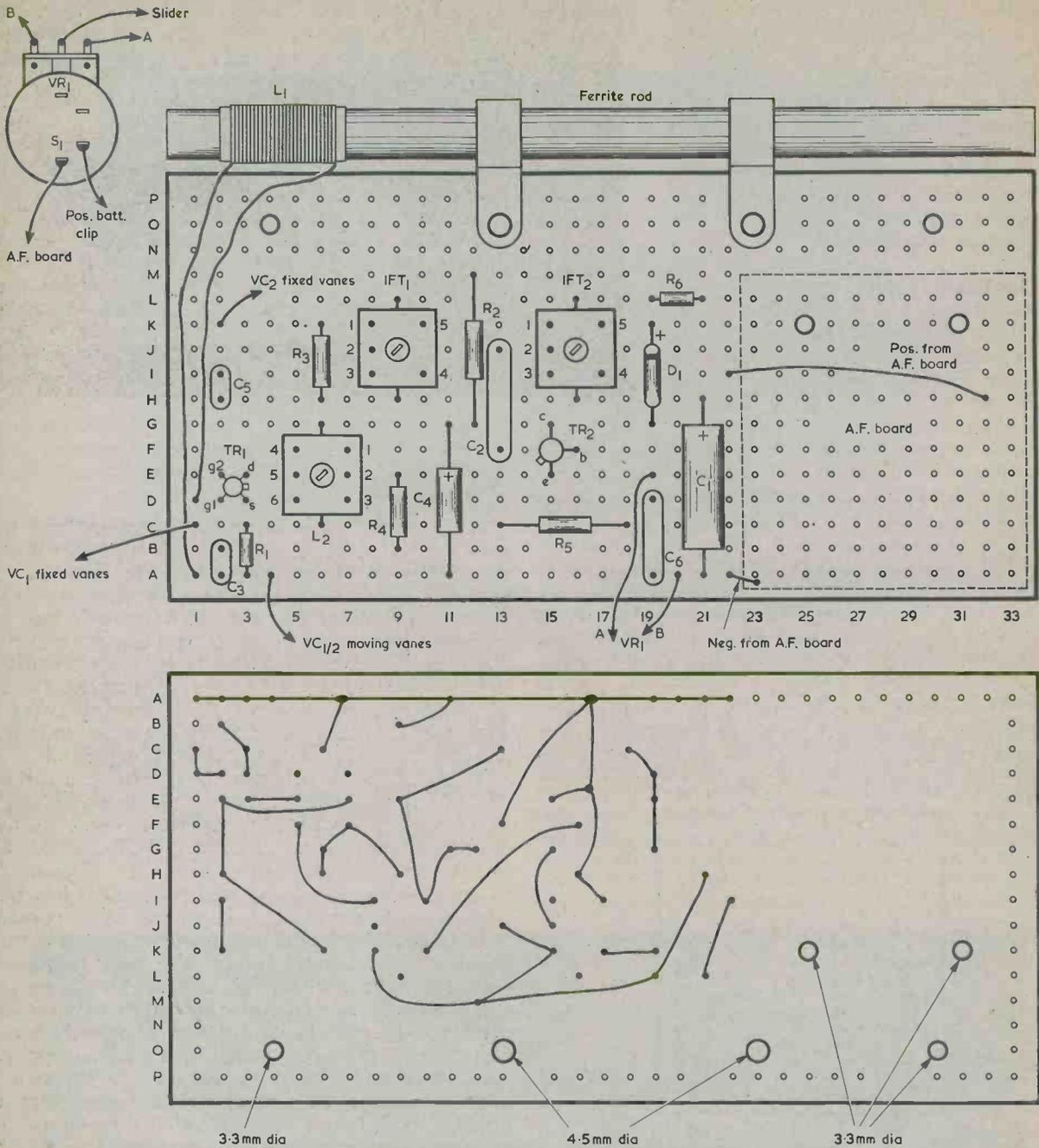
Fig. 2. The main component board. Check with the inset diagram of Fig. 1. to obtain correct orientation of L2.
