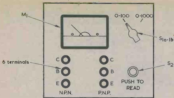
**Fig. 4. A recommended front panel layout for the hFE meter. Connections to test transistors are made by way of short flexible leads terminated in small crocodile clips.**
