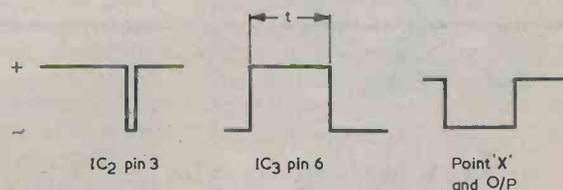
Fig. 4. The waveforms which appear in the power supply circuit. The length of  $t$  is set by R3.
