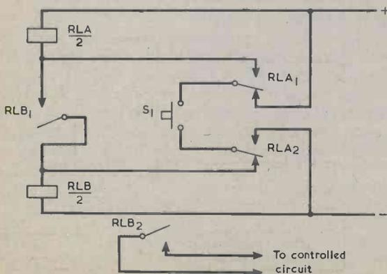
Fig. 3. A sequential switching circuit.
