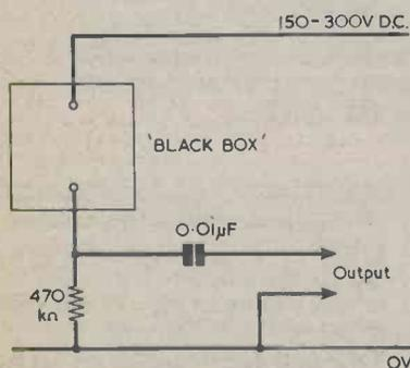
Fig. 7. Dick's black box. What are the two components inside the box which produce the mysterious 100Hz oscillation at the circuit output?
