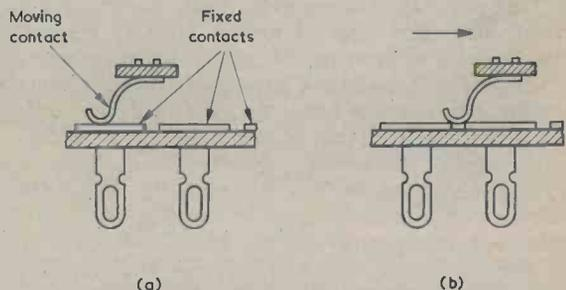
Fig. 2(a). Side view showing two fixed contacts in a typical make-before-break rotary switch.
