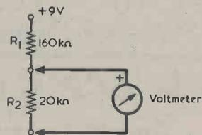
Fig. 1. A simple test circuit. The voltage across R2 is 1 volt, but an analogue voltmeter will indicate a voltage lower than this.
