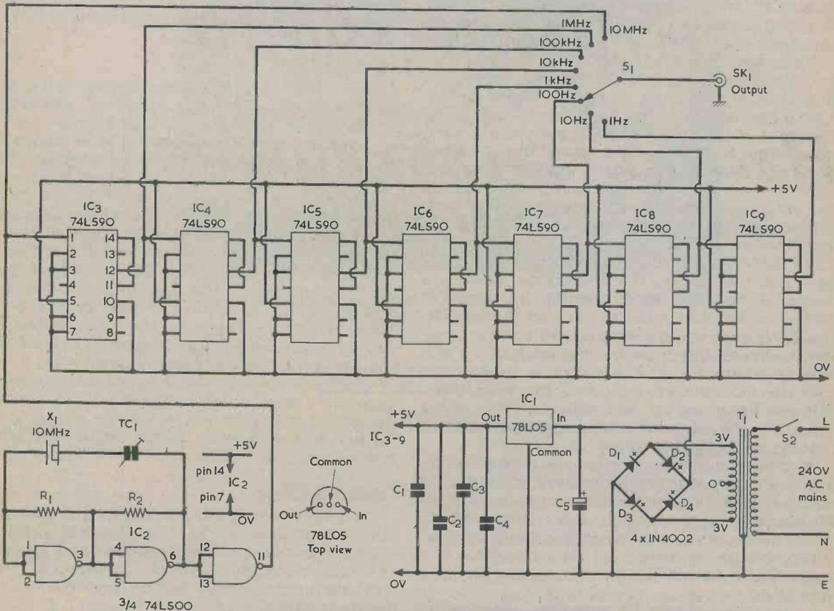
Fig. 1. The circuit of the crystal calibrator. Two gates of IC2 function as a 10MHz crystal controlled oscillator, with the third gate squaring up the output. Each 74LS90 acts as a decade divider.
