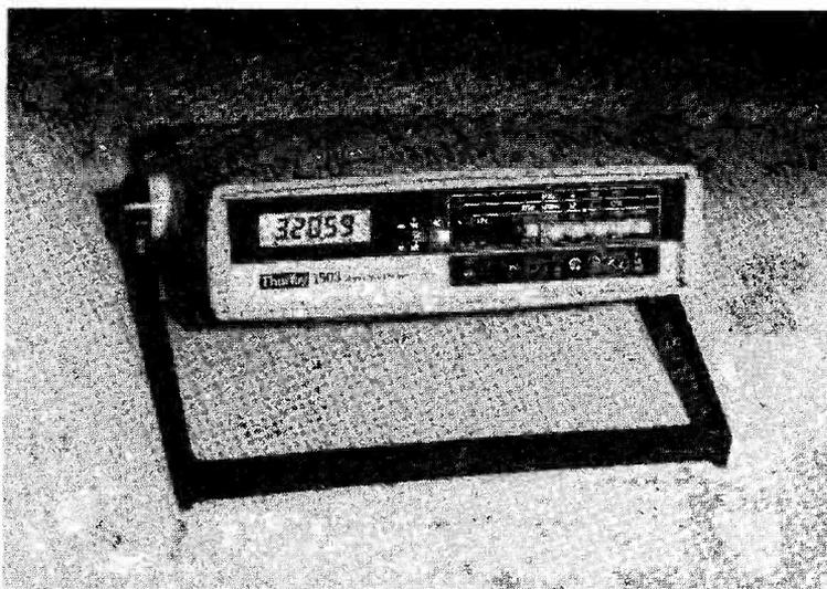
1,000M $\Omega$  can be selected for low voltage readings as an alternative to the standard 10M $\Omega$ . Maximum voltage input is 1,200 volts and currents can be measured up to 25 amps.
