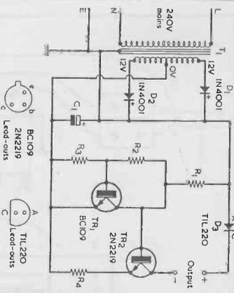
Fig. 1. The circuit of the NiCad battery charger. This is specifically intended for charging PP3 size batteries.
