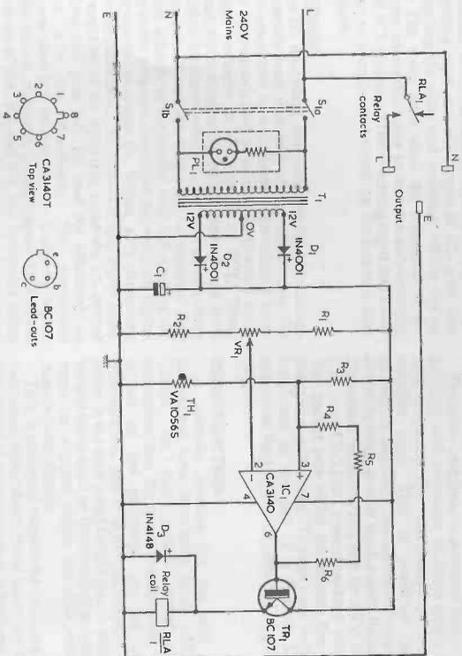
Fig. 1. The circuit of the thermostat unit. The temperature sensing device is TH1. The positive feedback around IC1 provided by R6, R5 and R4 gives snap-action triggering with hysteresis
