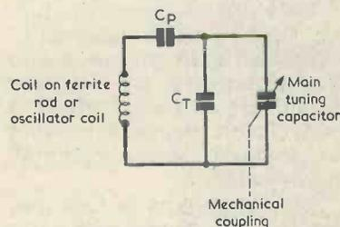
**Fig.3.** Smithy sketched a simple tuned circuit and added two extra preset capacitors . . . Cp is the 'padder' which can effectively reduce the maximum value of the main tuning capacitor. Ct is the 'trimmer' which can effectively increase the minimum value of the main tuning capacitor. By adjusting Cp and Ct the overall tuning range can be altered.
