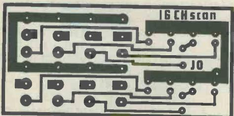
PC foil detail (1:1) for the lockout switch and LED front panel PCB
