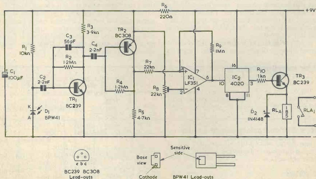
Fig. 4. The circuit diagram of the Infra-Red Receiver.
