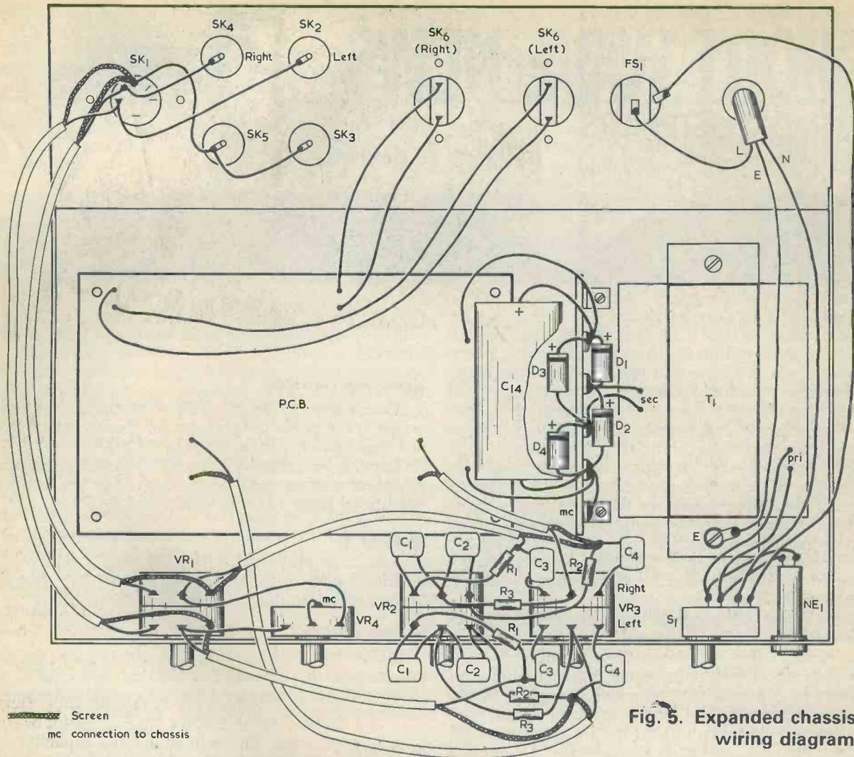
Fig. 5. Expanded chassis wiring diagram
