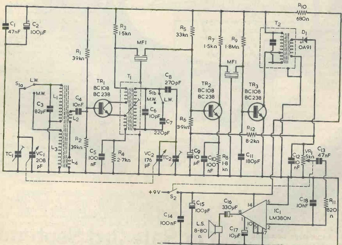
Fig. 1. The complete circuit diagram of MW/LW superhet radio.
