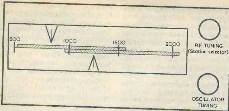
Fig.2. Smithy's idea of the tuning arrangements for a hard-to-tune superhet which nevertheless could achieve perfect tracking. The top pointer is set to select the station. The bottom pointer is then set to be 465kHz higher.
