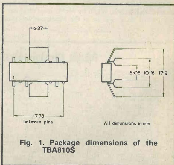
Fig. 1. Package dimensions of the TBA810S
