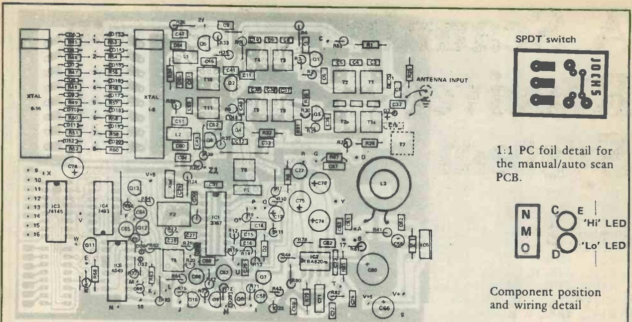
The numbered points on the PCB should be connected to the corresponding numbered point on the front panel PCBs.
