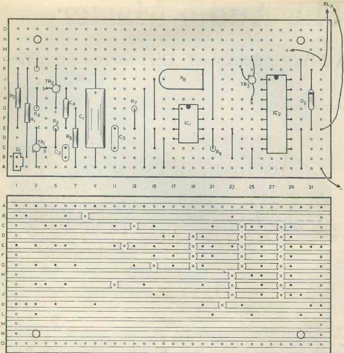
Fig. 6. The 0.1in. matrix stripboard layout for the Infra-Red Receiver.
