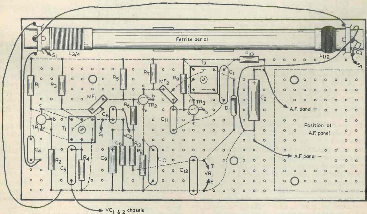
Fig. 2. Details of the plain 0.15in. matrix component panel.
