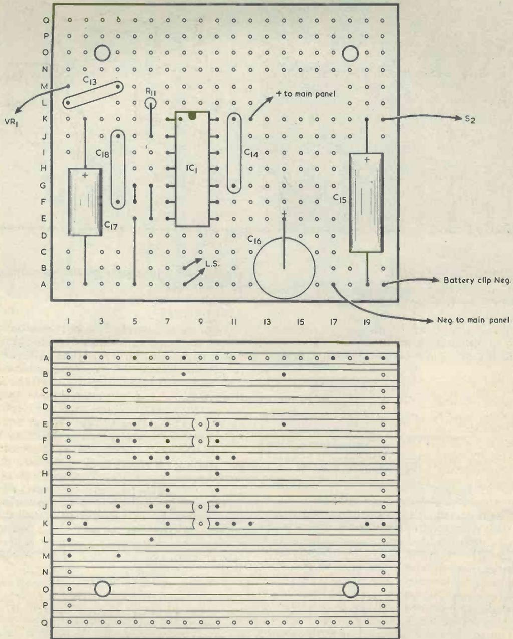
**Fig. 3. Details of 0.1in. stripboard panel on which the AF amplifier is assembled.**
