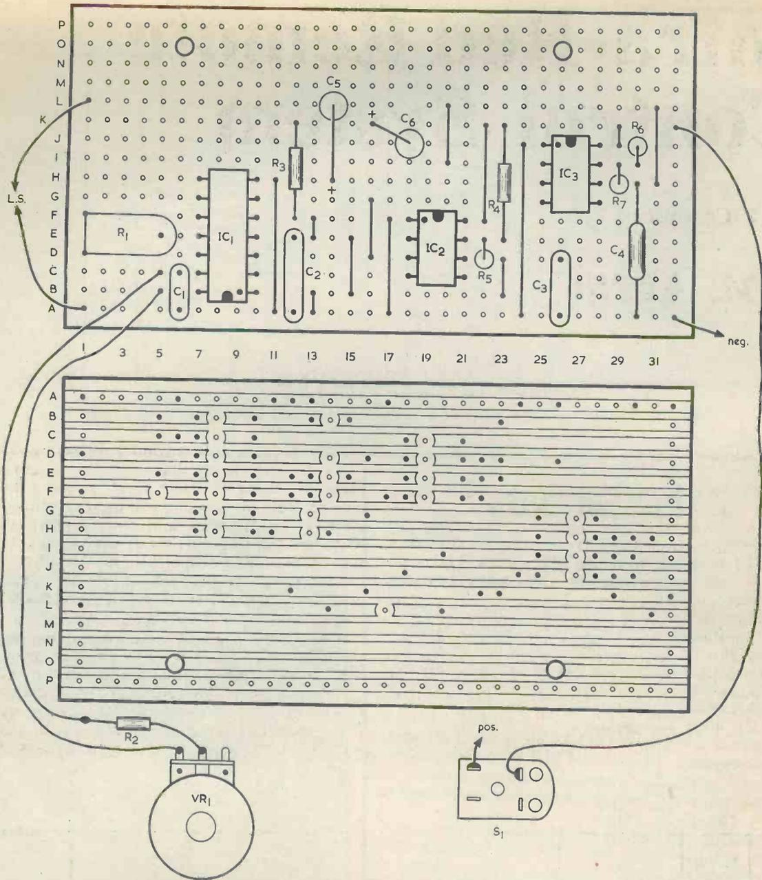
Fig. 5. The wiring of the Timer and details of the component panel.
