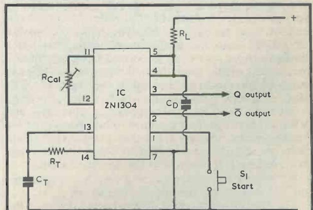
Fig. 2. Basic ZN1034E Timer circuit.
