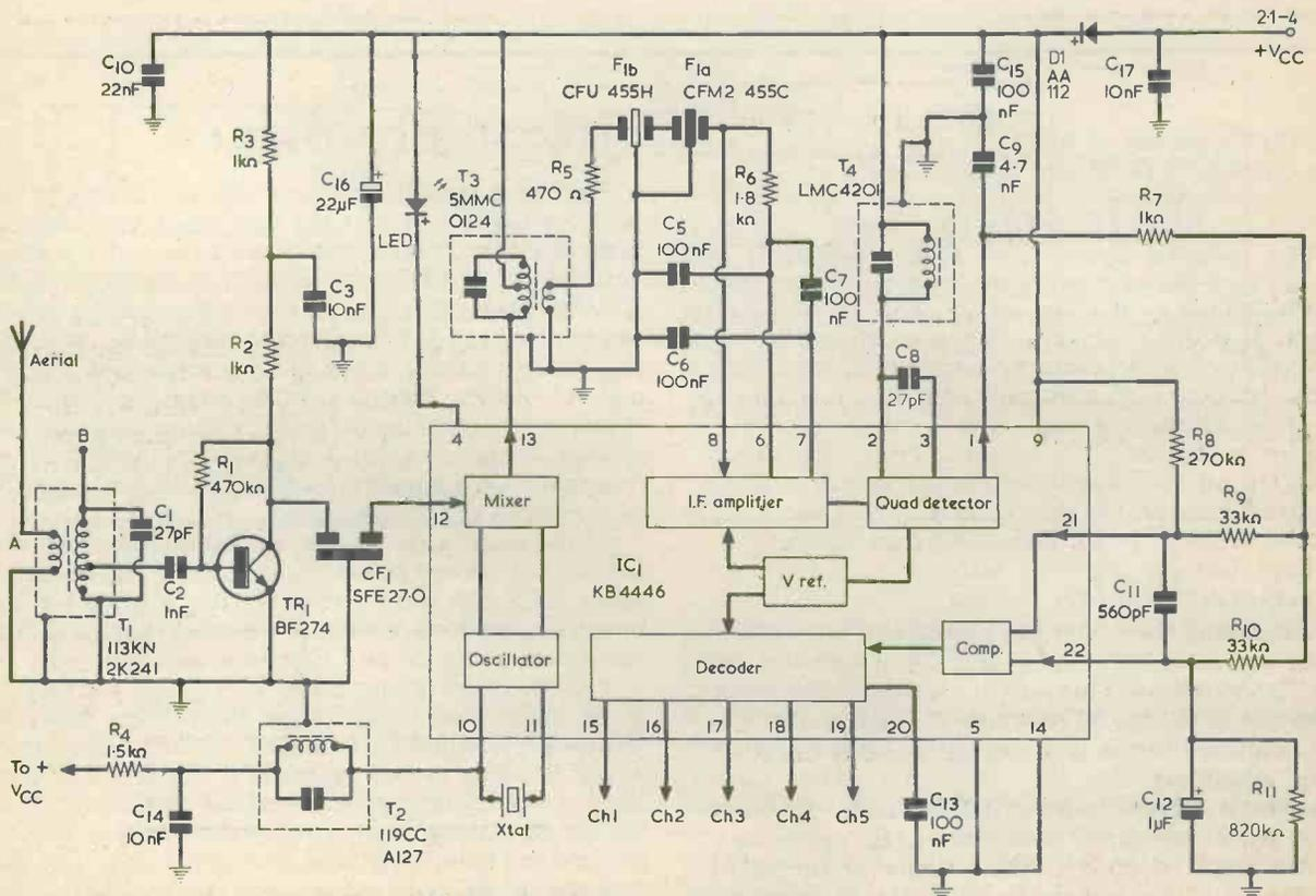
Fig. 5. The receiver circuit.
