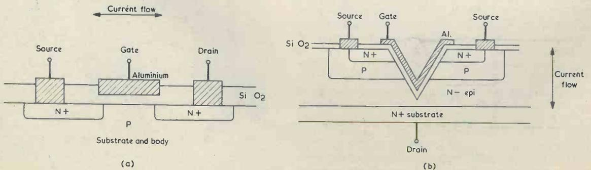
Fig. 1. (a) Cross section of Conventional Mosfet (b) Cross section of Vmos device
