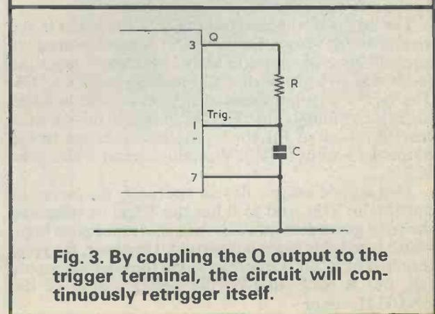
Fig. 3. By coupling the Q output to the trigger terminal, the circuit will continuously retrigger itself.
