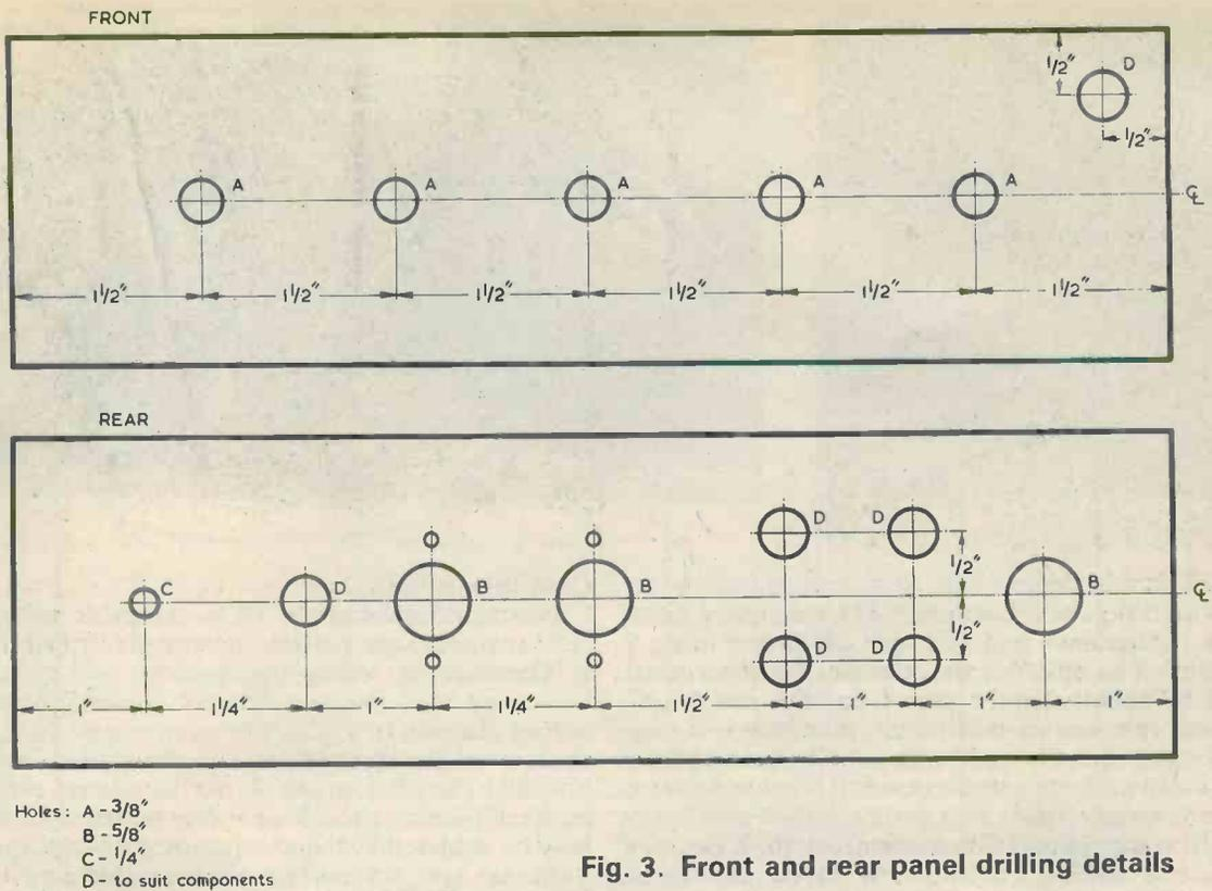
Fig. 3. Front and rear panel drilling details
