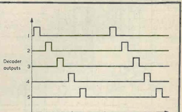
Fig. 3. Decoded output pulses to drive the servos.
