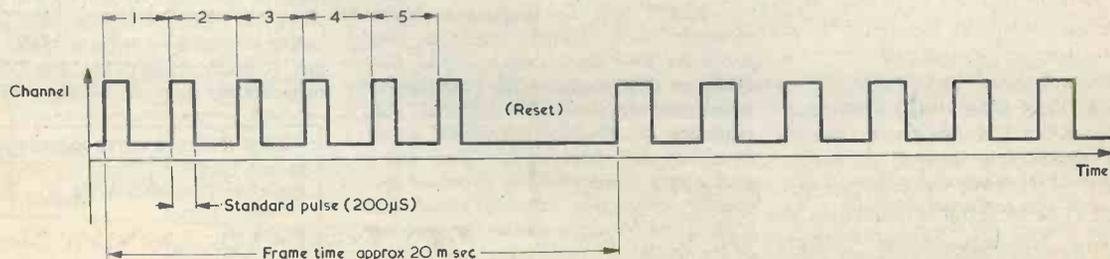
Fig. 1. The control waveform at the encoder output and decoder input.
