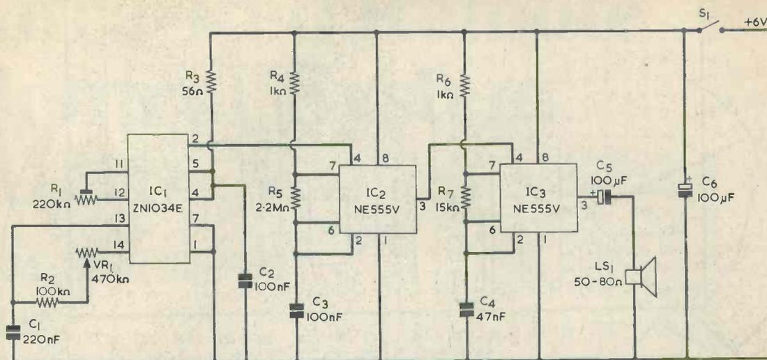
Fig. 4. The circuit diagram of a simple timer using the ZN1034E Timer IC.
