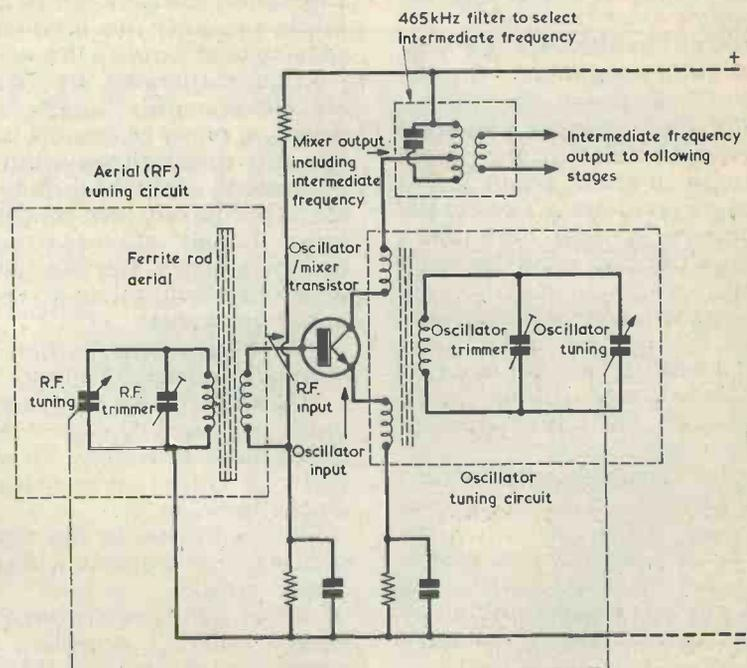
Fig.1. Smithy's sketch of a simple Oscillator/Mixer stage shows the first important sections of Dick's 'tranny' superhet radio. The variable capacitors are 'ganged' together and each has an additional trimmer capacitor to help with the 'tracking'.
