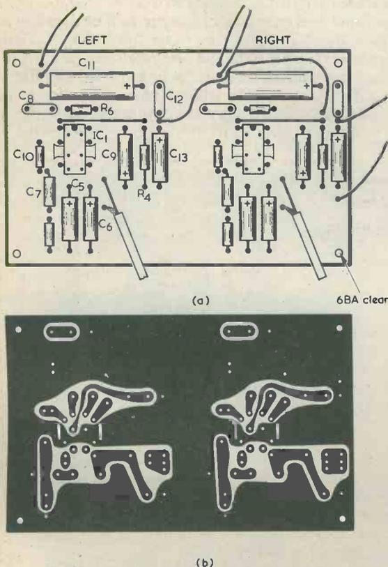
Fig. 4. (a). Component layout on top-side of board
