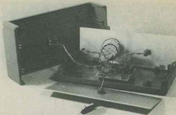
The prototype timer unit with the case disassembled. The Veroboard panel is mounted on the case bottom.
