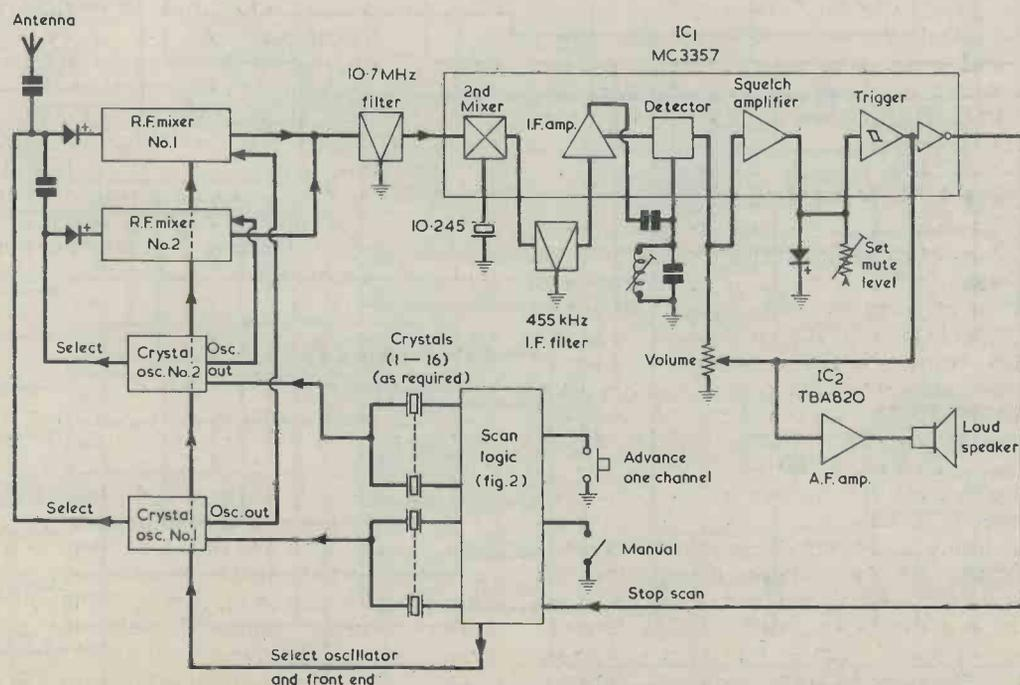
Fig. 1. Block schematic of receiver. The oscillator and mixer stages are duplicated to allow scanning over two widely separated bands.
