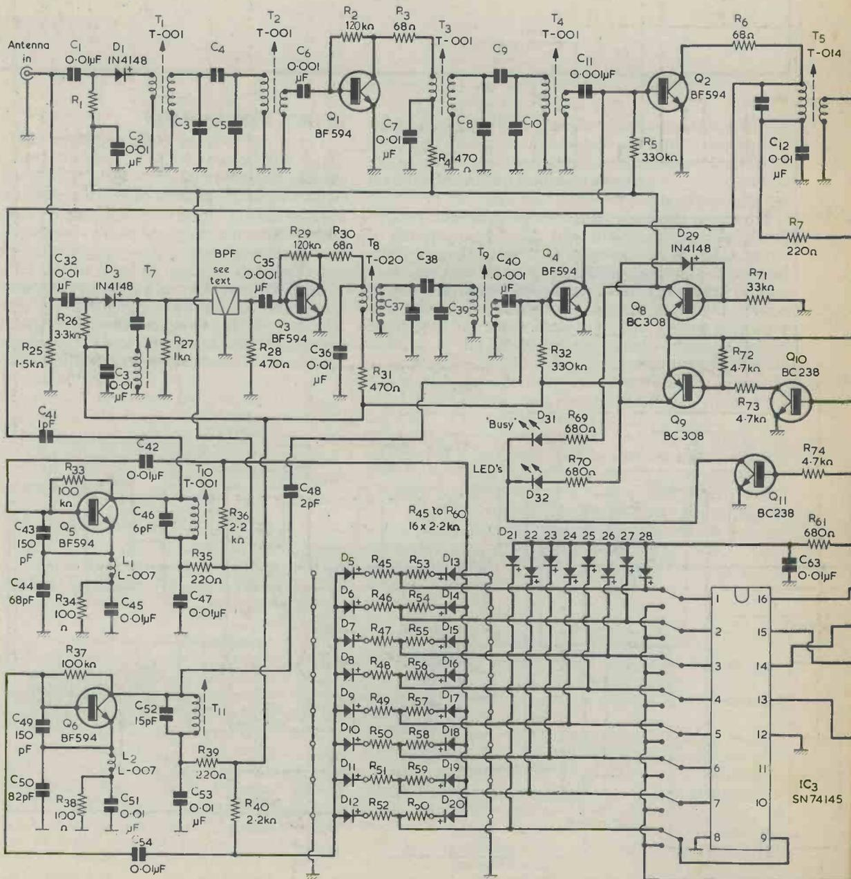
Fig. 3. Circuit of complete receiver. Details
