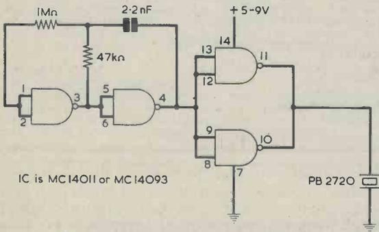
Fig. 4. Simple CMOS drive.
