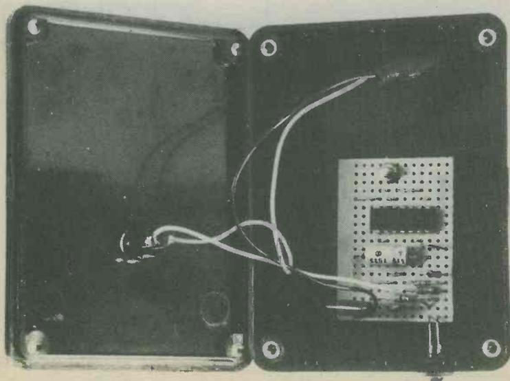
The transmitter electronics in case.
