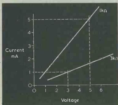
Fig.2. Smithy shows the straight line or 'linear' relationship between voltage and current for fixed values of resistance.
