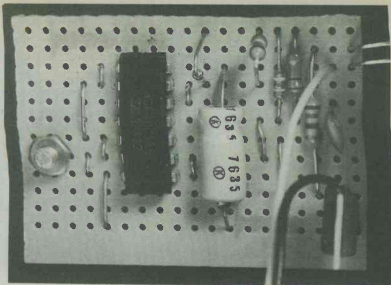
on, and must be reverse biased in order to switch them off. Tr1 is an *enhancement* mode device which, like an ordinary bipolar device, is normally in the off state and must be forward biased in order to switch it on. Thus, during the brief positive output pulses from IC1 Tr1 is biased into conduction and provides pulses of current L.E.D. D1 via current limiting "on" resistance and is capable of providing the high L.E.D. currents required.
