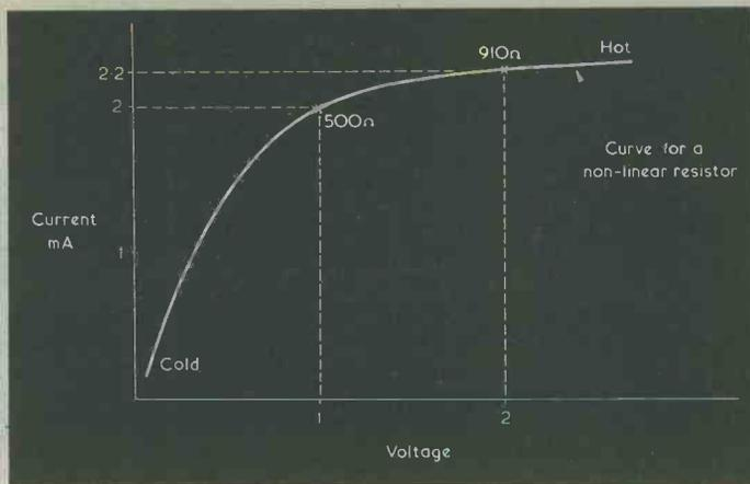
Fig. 3. Positive Temperature Coefficient. Although the resistance is different at each point of the graph, the volts, amps and ohms still obey Ohm's Law.
