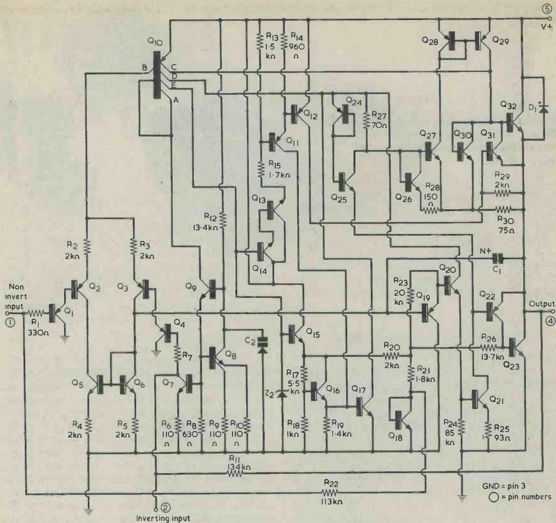
Fig. 3. TDA 2020 internal circuit diagram.
