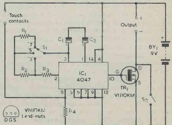
Figure 1. The circuit of the radio switch-off timer unit. IC1 and TR1 draw a negligibly low current in the standby condition.
