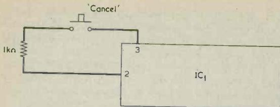
**Figure 3.** If desired, a "cancel" push-button can be connected to the circuit, as shown here. When pressed, this brings timing period rapidly to a close.
