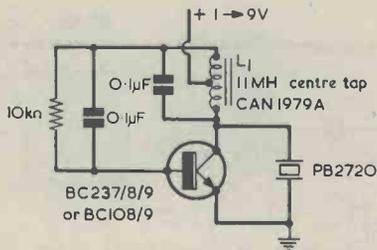
Fig. 3. Tune for resonance. Ultra high output/low consumption tuned transformer drive.
