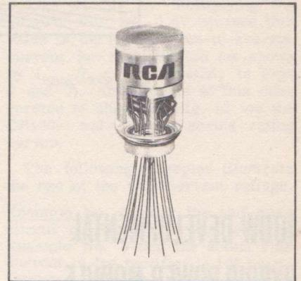
The recently released RCA Developmental Type C31016A is a very short, ruggedized, 10-stage head-on type of photomultiplier tube having a bialkali photocathode of high quantum efficiency and high-stability copper-beryllium dynodes. The maximum length of this tube is only 1.85", its maximum diameter is only 1.05".
