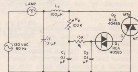
Fig. 6. A typical light-dimmer circuit.
