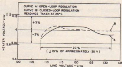
Fig. 5. Heater voltage as a function of line voltage of the open and closed-loop regulators.
