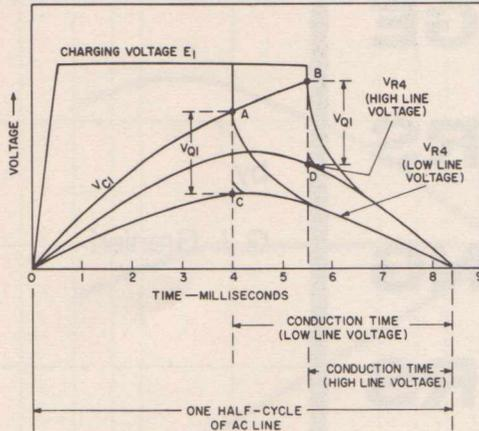
Fig. 2. Voltage waveforms exhibited by the ac regulator in Fig. 1.
