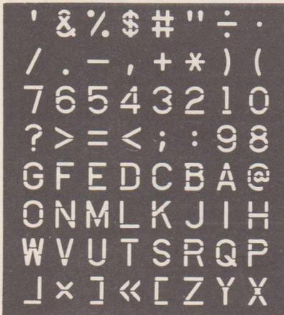
Typical Stencil Electrode Pattern of a 4560 Tube.
