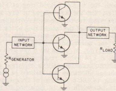
Fig. 16. A method of paralleling rf power transistors at a single point.
