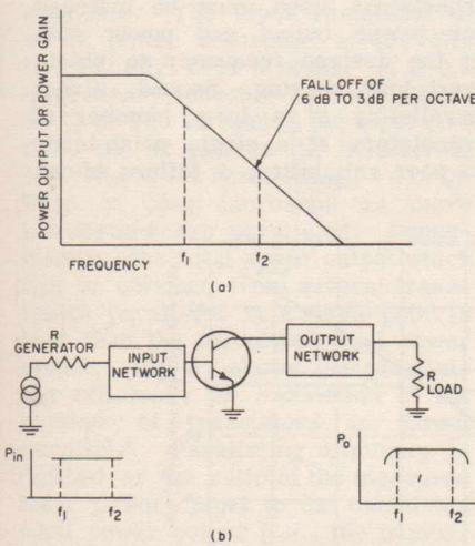
Fig. 10(a) Output power as a function of frequency in a power amplifier; (b) equivalent broadband amplifier.
