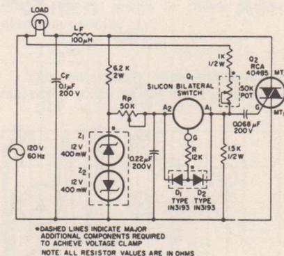
Fig. 7. A light-dimmer circuit that includes clamping.
