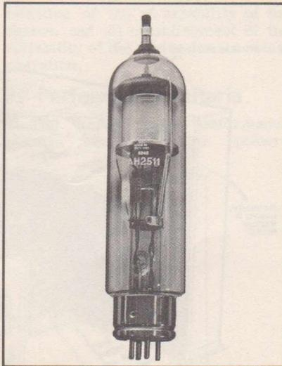
Maximum ratings for the AH2511 are 15kV peak inverse voltage and 12A peak current. In a three-phase full-wave circuit it will provide a d.c. output ranging from 14.4kV 9A to 2.3kV 15A according to the operating conditions.
