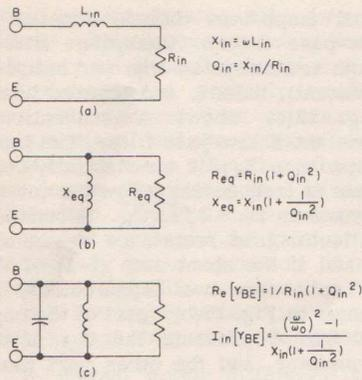
Fig. 13(a) Series equivalent input circuit of an rf power transistor; (b) equivalent parallel input; (c) equivalent parallel input circuit with external base-emitter capacitance.
