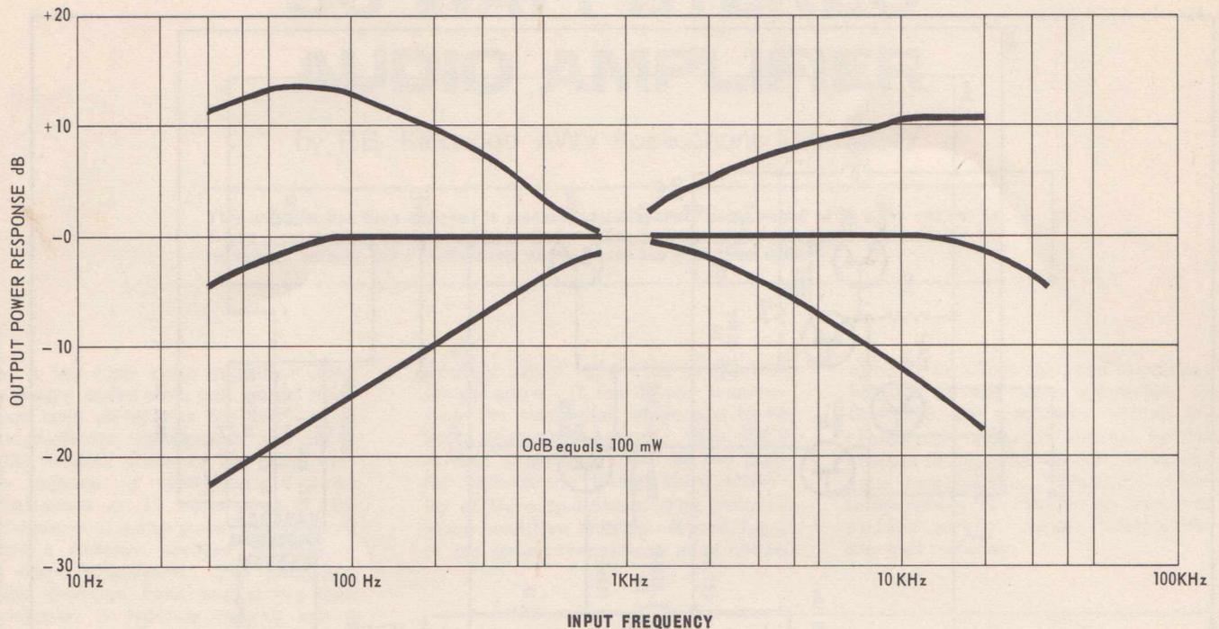
Fig. 2. The above curves indicate the overall flat frequency response of the amplifier and the frequency responses with the bass and treble tone controls set in their maximum positions.
