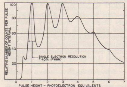
Typical Photoelectron Pulse Height Spectrum
