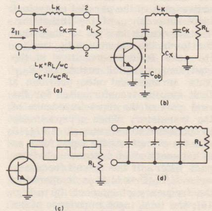
Fig. 12(a) A conventional constant-K low-pass filter; (b) a method of obtaining a constant-collector load resistance; (c) a short step microstrip impedance transformer (d) a lumped-equivalent Chebyshev impedance transformer.
