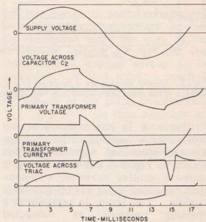
Fig. 11. Voltage waveforms exhibited by the circuit of Fig. 9.
