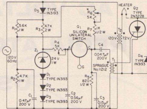
\* IN THE CLOSED-LOOP REGULATOR  $R_6$  IS REPLACED BY A PHOTOCELL RCA SQ2520 AND A POTENTIOMETER IN SERIES WITH A 6-VOLT INCANDESCENT LAMP IS CONNECTED IN PARALLEL WITH THE HEATER TERMINALS
