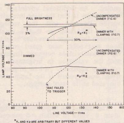
Fig. 8. Lamp voltage as a function of line voltage for two values of  $R_p$  in the circuits.
