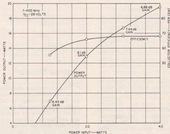
Fig. 14. Output power and efficiency as functions of input power for the RCA Dev. No. TA7344 at 28 volts.
