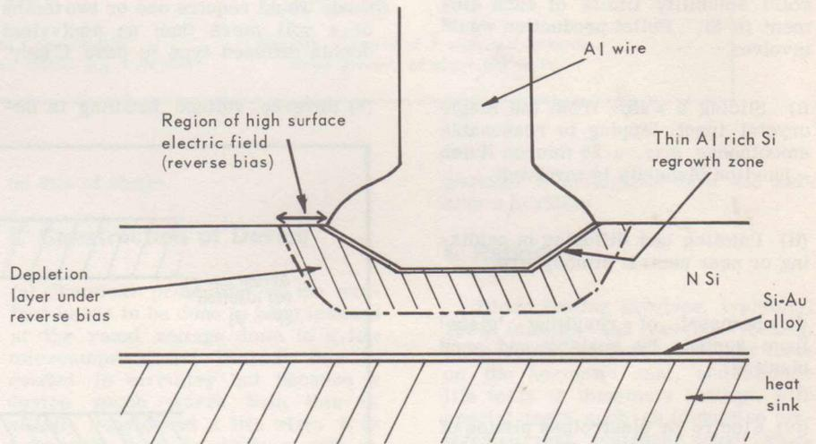
Fig. 1. Typical alloyed diode: rectifying element
