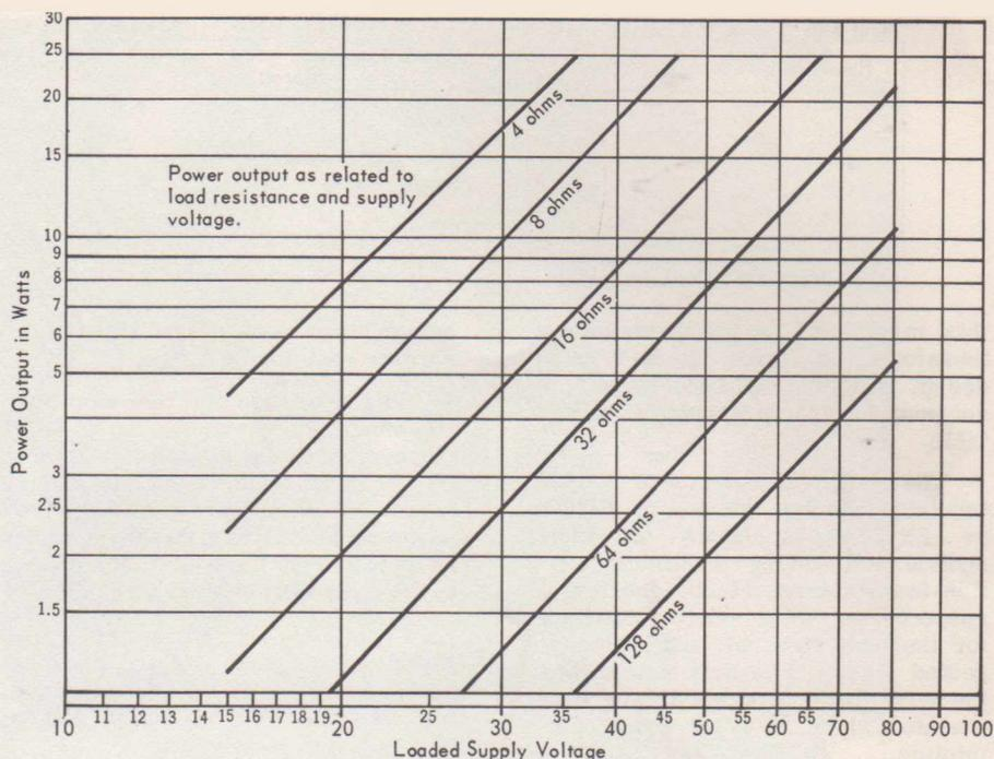
Fig. 5. Operating Characteristics
