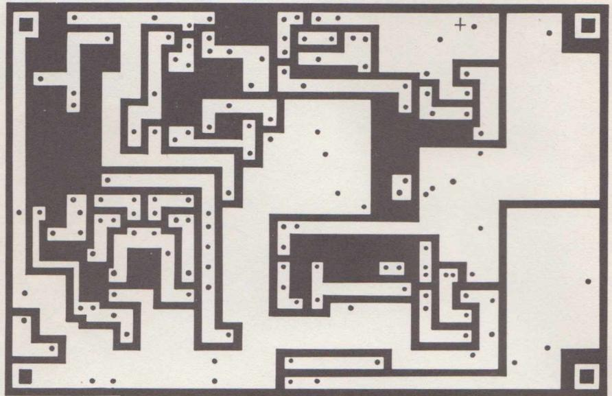
Figure 1. Full size template of the copper side of board.
