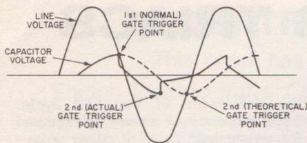
Fig. 4. Charging cycle of the capacitor-diac network in the circuit of Fig. 3
