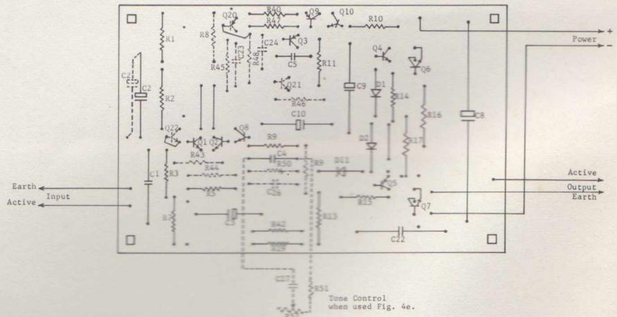
Figure 2. Component layout on top of board.
