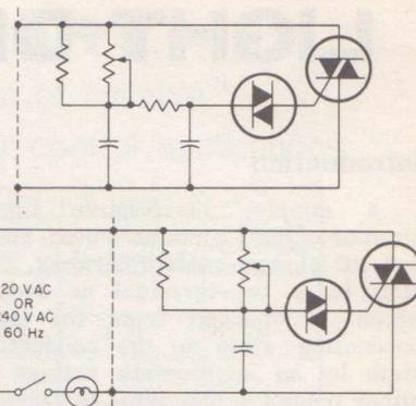
Fig. 9. Light-control circuits incorporating a trimmer resistor across the potentiometer.
