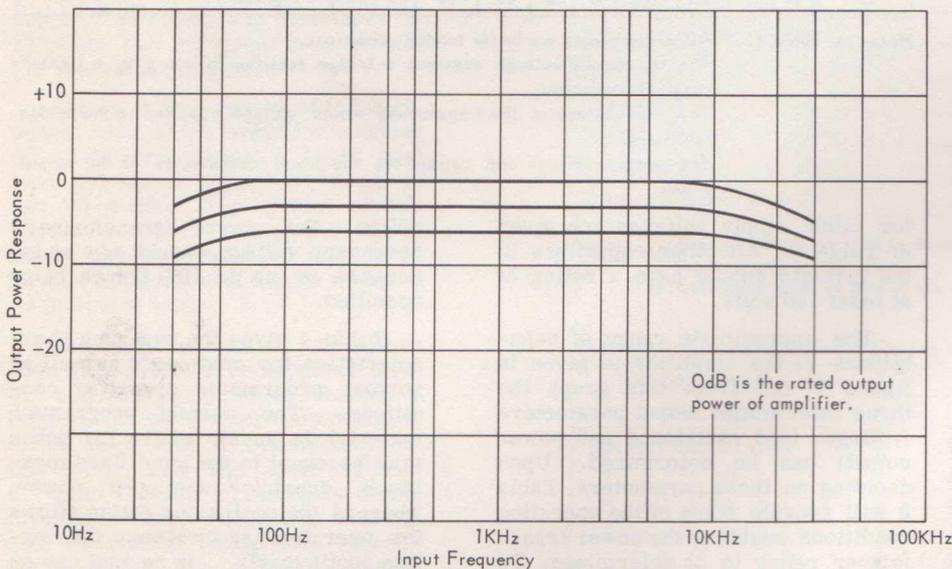
Fig. 6. Frequency Response Curve
