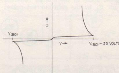
Fig. 2. Voltage-current characteristic of a diac.
