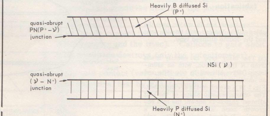
Fig. 4. Doping structure of double diffused Type of Fig. 2.
