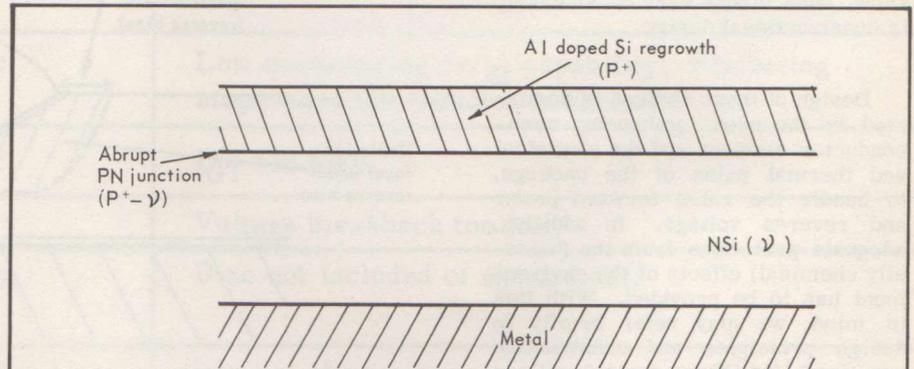
Fig. 3. Doping structure of alloyed type of Fig. 1
