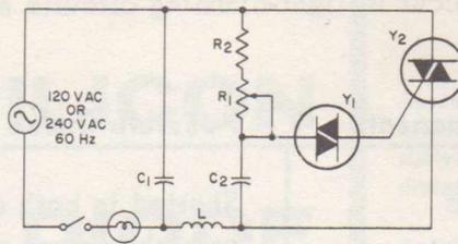
Fig. 11. Single-time-constant light-dimmer circuit.
