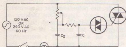
Fig. 6. "Double-time-constant" light-control circuit.
