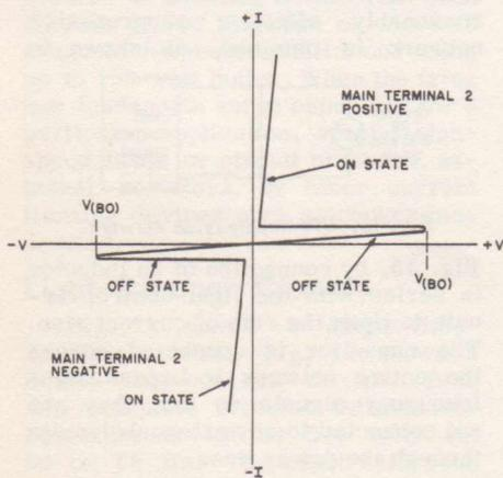
Fig. 1. Voltage-current characteristic of a triac.
