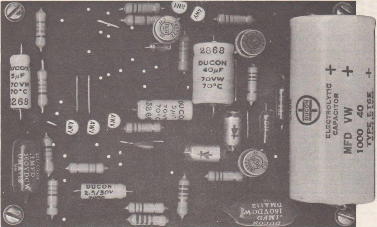
Figure 7. Photograph of component side of board wired for the basic circuit
