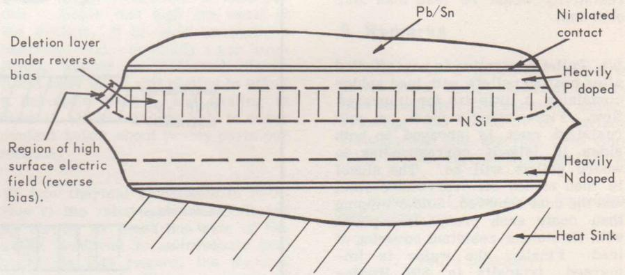
Fig. 2. Typical double diffused diode: rectifying element
