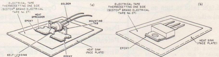
Fig. 13. Examples of isolated mounting of triacs.
