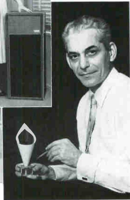
*Small in overall size, the EICO HFS-2 speaker system achieves unusually good bass response through its novel loading slots (above) and treble distribution by a unique free-floating tweeter shown at right with its inventor, Mr. Stewart Hegeman.*
